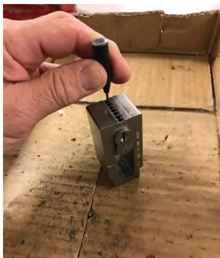
Figure 8. This is how I was using the Annex without the "code book" in place. I needed only to eject the pins in the first chamber and not decode them. Because I would have to remove the code book to dump the pins each time, I decided to save a step and leave it out. This is why you see me doing it in that modified cardboard box — to catch the pins as they ejected.
