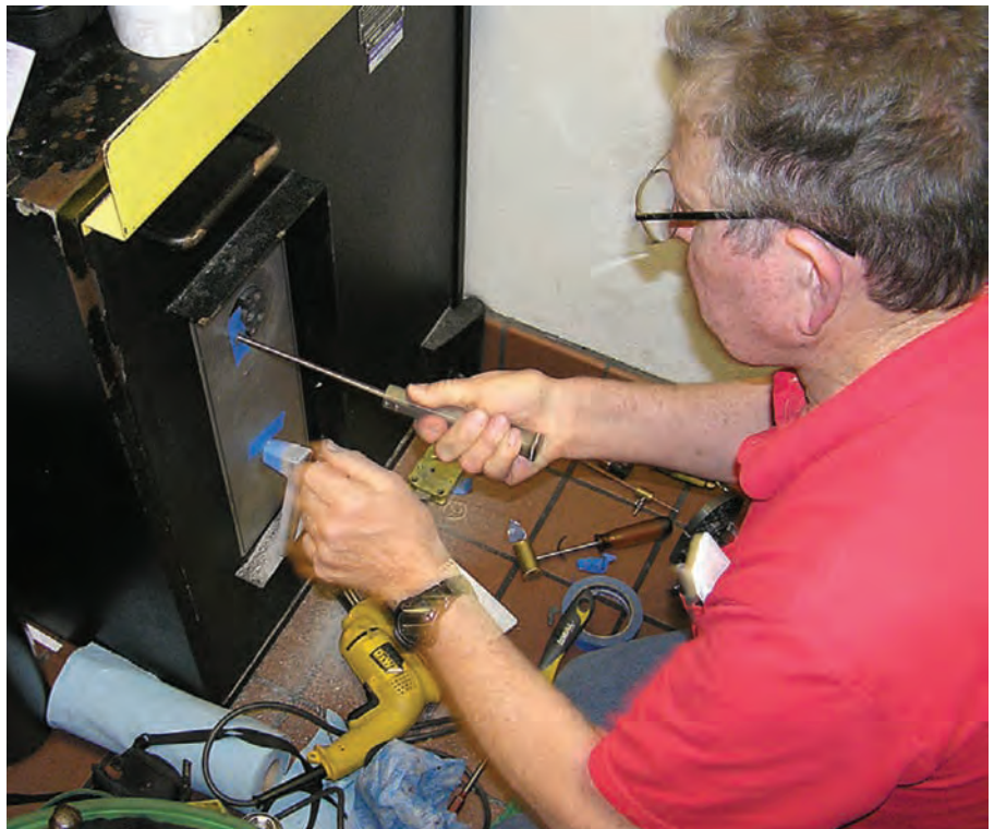
The author is shown packing steel stick in to the hole to help hold the ball bearings.
