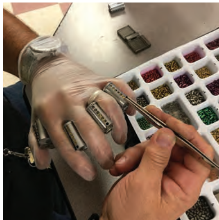
Figure 14. This photo shows how I get a lot of cores done in the least amount of time. Remember that the core pullers are bringing me batches of cores at a time, and I need to keep up. In this picture, I'm holding five cores, but I've done seven at a time in the past. What I'm doing is dropping the bottom pins into the first chamber of each core, moving from right to left. When I get to the last core, I drop the second pin in each going left to right. I continue in this fashion until all the pins are inserted.
