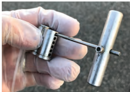
Figure 13. I start by ejecting the first chamber on five or six cores and then use the reamer on that chamber, as shown here. Just insert it and twist it back and forth. I do this because sometimes when you cap a chamber, however you do it, the core moves slightly. This can cause the punch or press topeen over the hole slightly. This can make it difficult to get the pins into the chamber, but the reamer cleans that up. It also removes any crud that might have accumulated.
