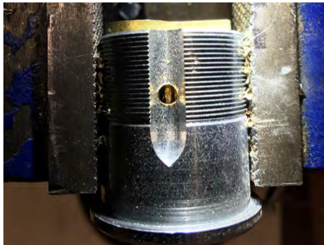
Figure 6. One method to remove a core without damaging it involves drilling a hole in the set screw channel closest to the control lug.
