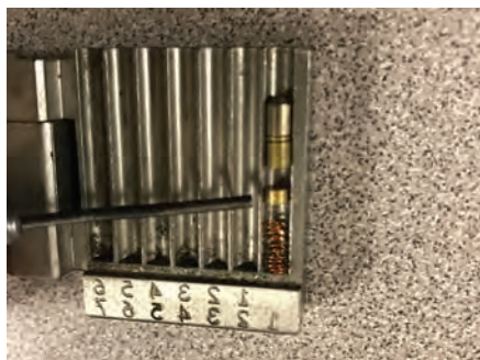
Figure 7. Here, I'm pointing at the top pin. If you can determine what size that pin is and subtract that number from 13, you'll have the control key cut for that chamber. If you did that for all chambers in the core, you'd be able to cut an operating control key for that system. This is golden if you need to remove a lot of cores where the control key is lost. Even better, you can reload the core with the old pins and new springs and caps and still use it. I've found it best to use a dial caliper to measure. You can also place a new pin next to the old to compare, but it's not foolproof. I highly recommend you search online to find Bill Lynk's great article from the April 2008 issue of Keynotes . (Google "decoding an SFIC system" to find it.) Read it. I doubt you'll find a better explanation of the subject anywhere else.
