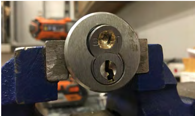
Figure 11. It's possible to drill to shim the core from the front by removing the core's scalp.
