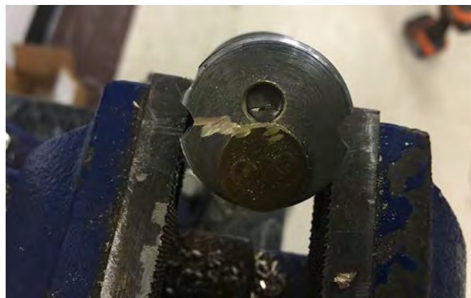
Figure 8. To drill the rear of the housing to shim the core, all that's needed is a 1/4" hole placed directly above the hole used by the cam.
