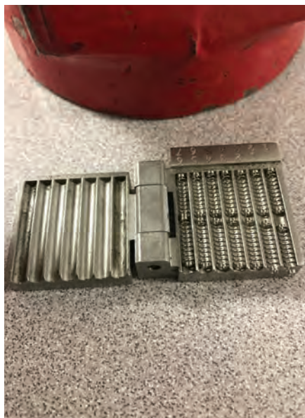
Figure 9. This photo shows another use I found for the code book: holding springs. One of the bigger time wasters on a large job such as this is having to untangle springs as you use them. I take a moment to set them up as you see here, and slide them out as I need them.
