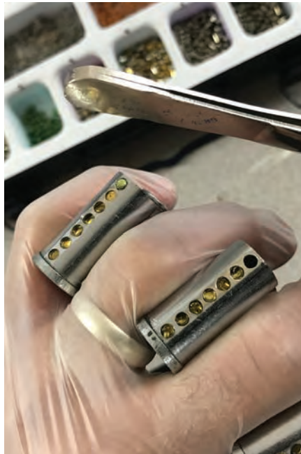
Figure 15. Sometimes, number 4 top pins tend to rotate and get stuck as I try to get them into the chamber. Here, I'm tapping the pin with the back of my tweezers to free it up.
