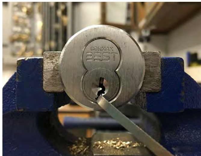
Figure 2. Once the lock is picked you can then use the tension wrench itself to remove the core.
