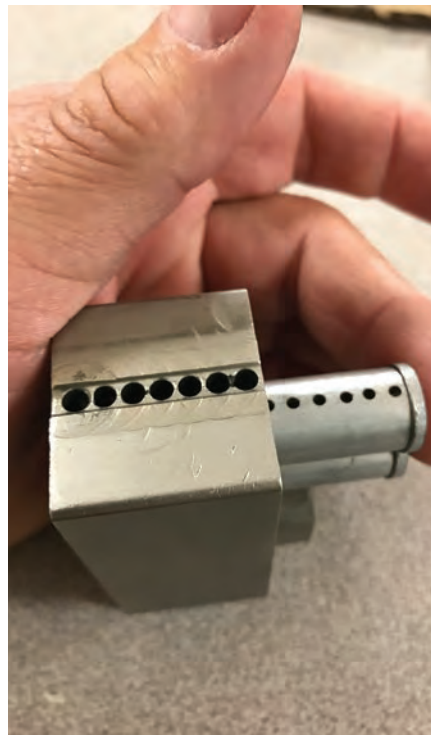
Figure 4. Here, I'm sliding the core into the Annex; note that it's upside down.
