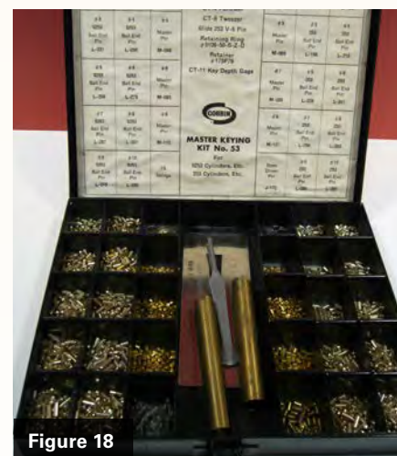
Figures 17-18. The Corbin 53 pin kit was the answer to bottom pins needed (with master pins) for the Corbin master ring cylinders, as well as some conventional cylinders.
