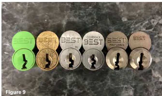
Figures 9-10. The drill point for the control shear line on BEST SF-ICs varies in relation to the BEST logo because the logo isn't the same or in the same spot on all of the brand's cores (Figure 9). What doesn't vary, however, is the distance between the control shear line and the operating key shear line (Figure 10).
