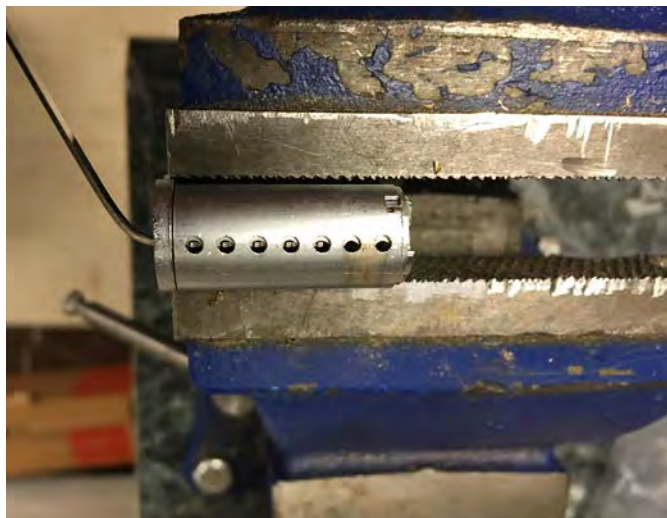
Figure 1. Peterson Manufacturing offers three tension wrenches that work by applying tension to the control lug via the ejector holes.
