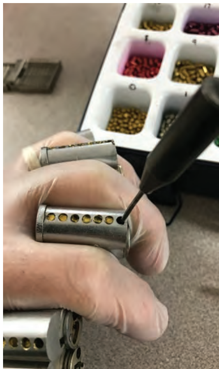
Figure 16. I'm using the pin ejector to make sure that pin isn't stuck. Take note of the lousy capping job on the other chambers. It looks like someone didn't have the right tools for the job.
