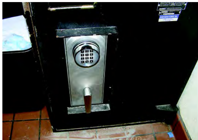
The new lock was installed and the handle was straightened.
