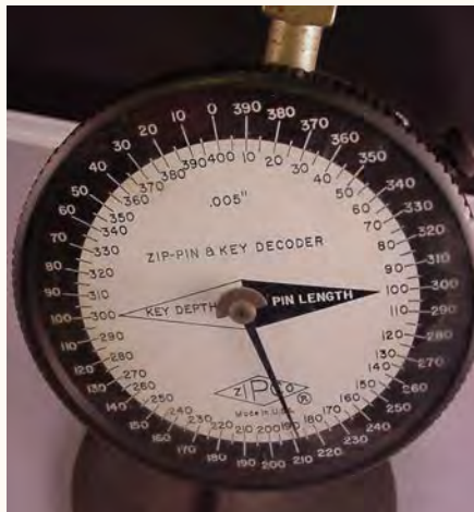
Figure 6. This vintage dial was manufactured by Zipf Lock Company to measure key depths, but it also worked well for deciphering pin depths.
