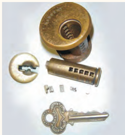
Figure 42. As you can see here, the five chamber holes are square, as are the pins.
