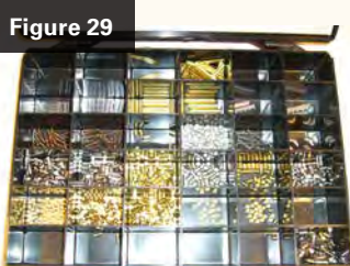
Figures 28-29. The first kit contains 36 compartments only for the six bottom pin orientations at the six increment depths (Figure 28). The second holds the drivers, masters, springs and spring covers (Figure 29).
