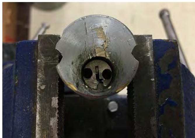
Figure 4. After reaching the control lug, remove the cam from the housing, as shown here.
