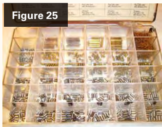
Figures 25-26. The Medeco Original kit 166-36 contained bottom pins in three angles, accommodating six depths and 18 different bottom pins.
