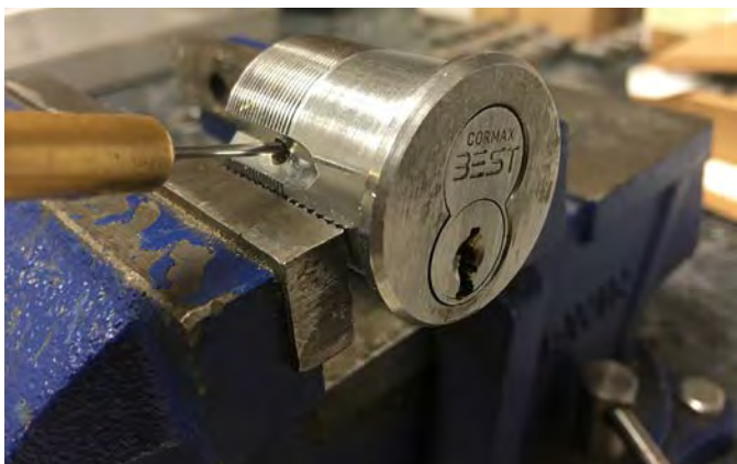
Figure 7. Once the hole in the set screw channel is created, you can then use a probe to apply pressure to the control lug and pick the core at the control shear line.
