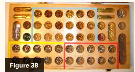
Figures 37-38. The Kaba Peaks Pin Kit has five basic sections: 1.) Master and top pins (top center, blue border), 2.) bottom pins for the .432" diameter plug (bottom right, red border), 3.) Bottom Pins for the .494" diameter plug (bottom left, yellow border), 4.) Misc. .432" diameter plug items (top right) and 5.) Misc. .494" diameter plug items (top left).
