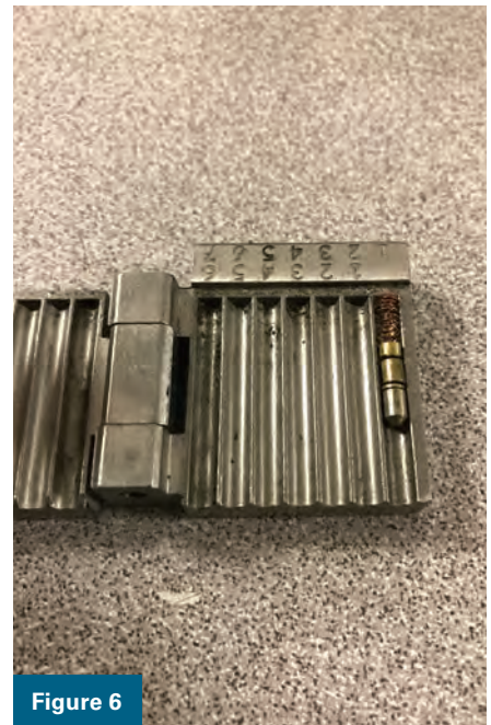
Figures 5-6. In Figure 5 , I'm about to strike the ejector with a small hammer. After carefully sliding out the "code book" and opening it, we get what we see in Figure 6 . What you see is the pins and spring as they appear in the core, except that the spring is crushed beyond repair; don't try to reuse it. One of the great features of the Annex is the ability to save the pin stack like this. I'll explain why in Figure 7 .
