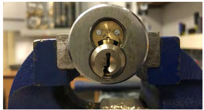
Figure 12. For Kaba/BEST cores, the scalp is held on by two posts: one post to the left and one post to the right of the stack containing the Peaks pins.
