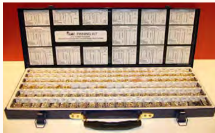
Figure 13. LAB's LCRK6 pin kit can be used for all biting classes, depth systems and both plug diameters.
