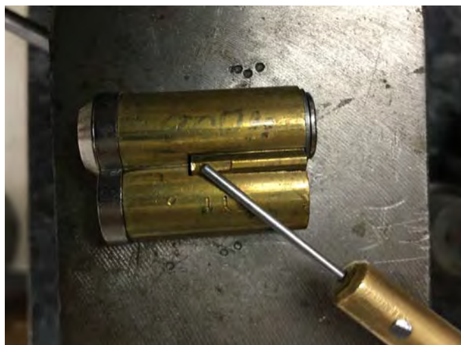
Figure 5. There is a very slight marring to the front edge of the control lug. This is from forcing the core through the remaining brass holding the core inside of the core.
