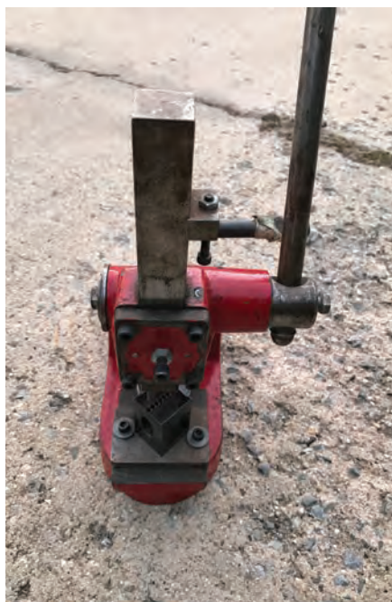
Figure 10. I used both the Annex and a capping press to recap the cores. I prefer to use the press, but it's kind of heavy to carry around and really ought to be screwed down. If there are a small number of cores to be done in a building, I usually used the Annex. You'll see both in use.
