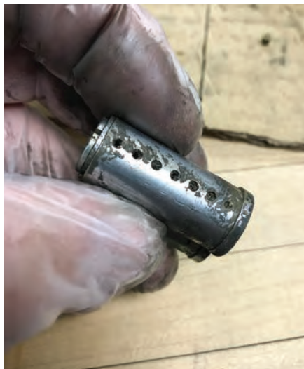
Figure 29. Second, you'll notice I'm not using graphite here. It's filthy to work with and difficult to clean up. A little of it goes a long way, but try telling that to a customer. This photo shows a buildup of graphite that's been mixed with other lubricants (such as WD-40) and caked up. It doesn't drip out the other side of the core if you overdo it, does it? The silicone and dry lubricants of today do a better job than graphite, in my humble opinion.
