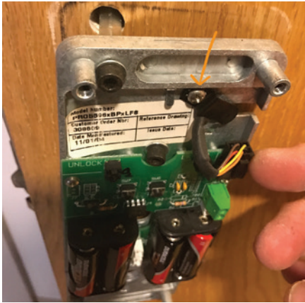
Figure 7. The author has loosened the screws on the backplate; it's hanging on a cable, and he's pointing at the connector at the end of the cable.
