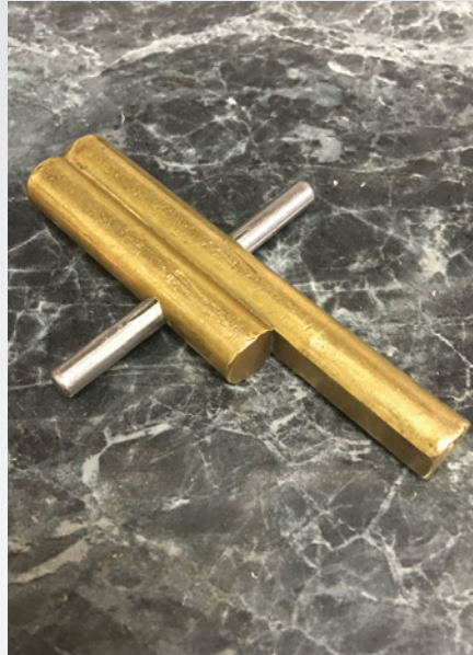
Figure 2. The mortise cylinder wrench, part ED211, can help with testing the timing of the lock.
