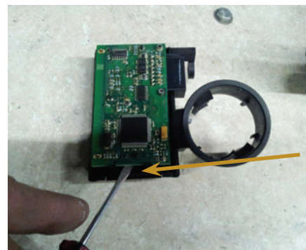
Figure 4. Carefully pry these two tabs to also release the board from the box. You haven't had to use anything but a screwdriver so far.
