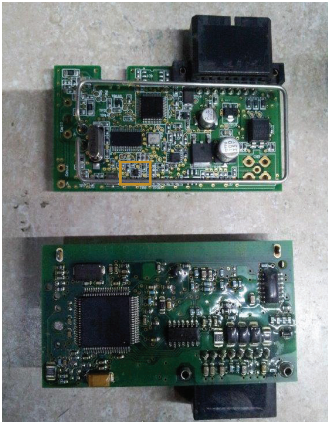
Figure 6. On the left is an old board from a 1999 Dodge we salvaged (we never throw anything away). Can you spot the crystal we're going to salvage? I'll show you because it's pretty small in this picture — much smaller than the one we're taking off.
