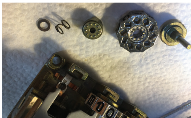
Figure 7. The part slides into the number wheels — one of which is shown here — each time the knob is turned to locked or unlocked.
