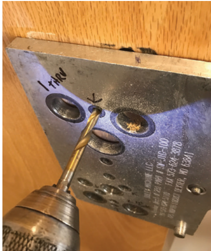
Figure 17. This image relates back to the orange arrows in Figure 14; the author is drilling a 1/4" pilot hole for each of the "A" holes and not the full-size holes. The full-size holes are drilled after the jig is removed.
