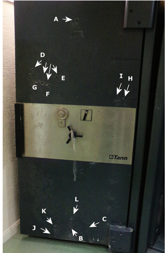
Figure 3. A scope was put down the keyhole, out the back of the lock case and inside the void of the door, showing that the scroll was in one piece. This image shows the location of each hole, marked with letters.
