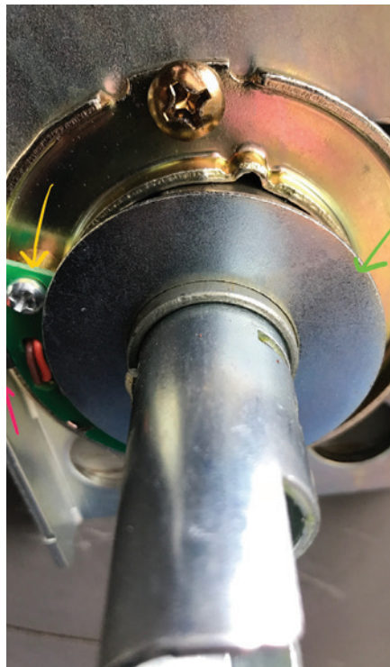
Figure 43. The backplate for the chassis is screwed in.
