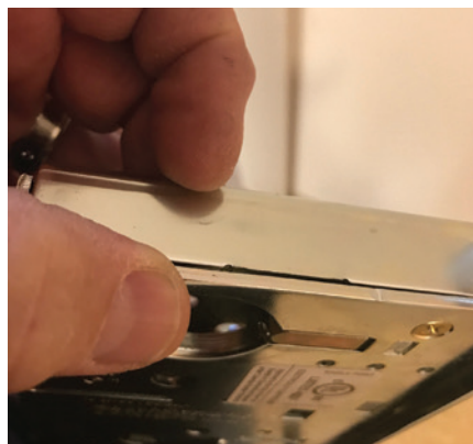
Figure 20. The author's thumb is on the "cover" of the chassis, and his forefinger is on the "case." Whichever of these faces the inside of the door indicates which RQE to use.
