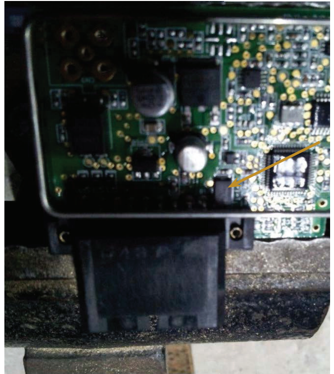
Figure 7. The crystal is always near the larger MCU chip. Here, it's as seen on the previous photo.
