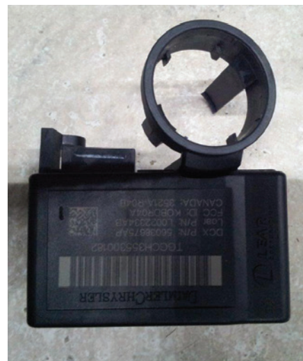
Figure 2. You must buy a transducer coil detector to test for a signal being sent by the coil. It should be the first thing you test once you have the key made — because if it isn't sending, you'll waste a whole lot of time trying to program it.
