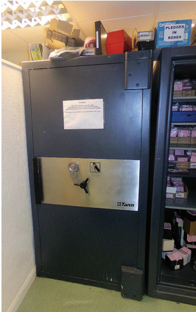
Figure 2. The safe was a Tann, but the model was unknown. The hinges were bigger, giving an indication it was possibly a banker-quality safe.
