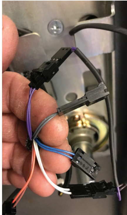
Figure 42. The purple door sensor wire is connected to the white wire, and the purple jumper is connected to the purple wire. The blue and gray wires aren't used.
