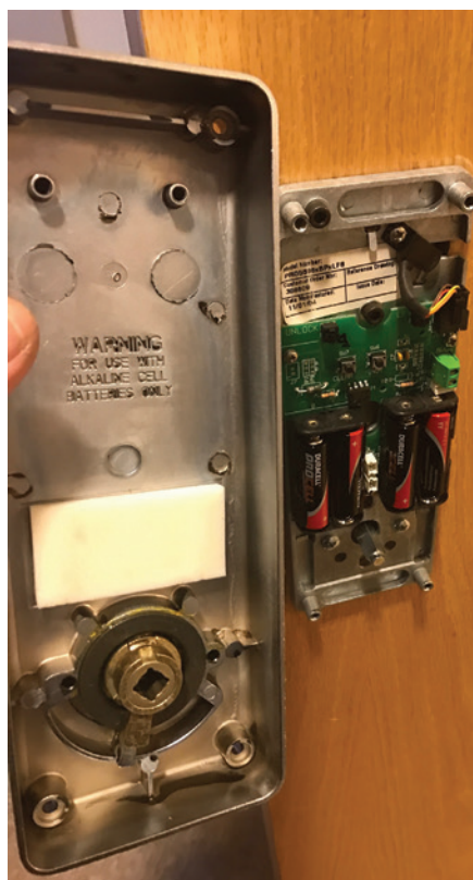
Figure 5. This image shows the inside trim removed and what's under it.
