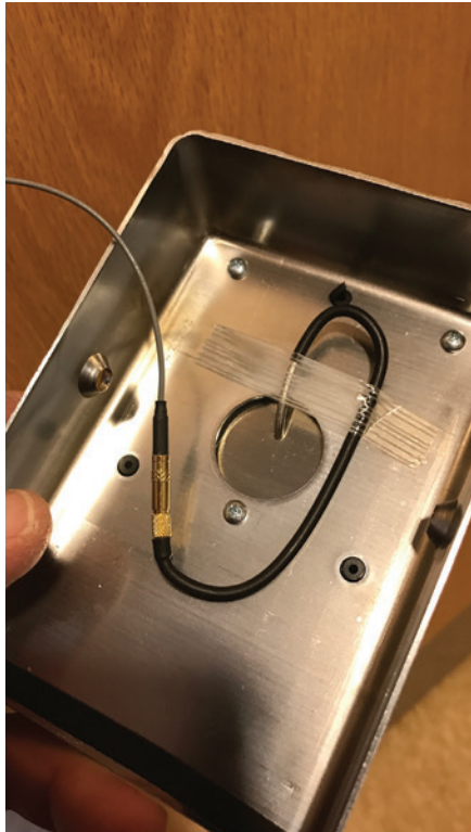
Figure 33. The top cover contains the locks antenna.
