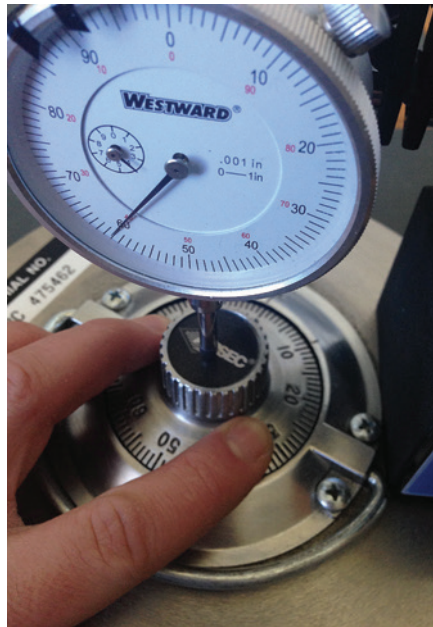
Figure 4. Keep the dial level as it “floats” back up so that each time you find the contact point, your indicator is giving you the same reading. You can use your index and middle fingers to press down on the edge of dial so that it always remains level.
