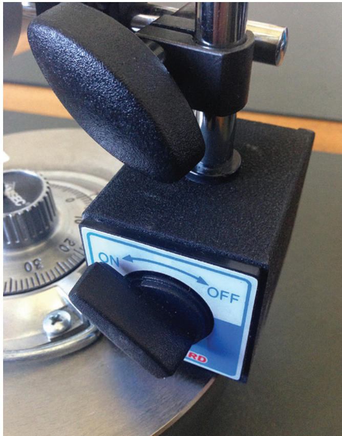
Figure 2. Place the magnetic base on the lid's edge so that the opening index will not be hindered from view, then throw the lever on.
