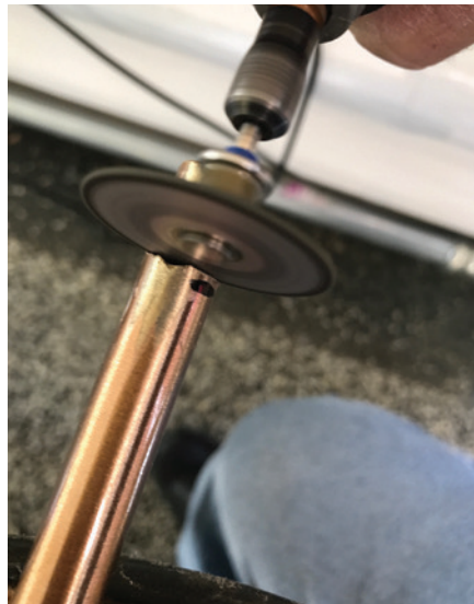
Figure 9. The author is cutting the bar with a Dremel.
