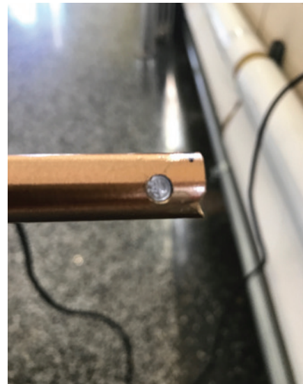
Figure 10. The author drilled a new hole in the rod for a steel pin.
