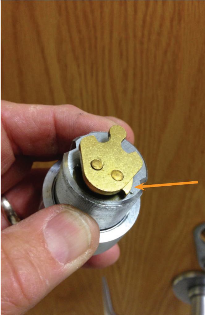
Figure 1. The arrow is pointing to what appears to be another cam under the existing cam.
