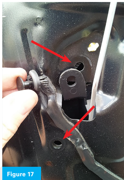
Figures 16-18. Pop these two buttons out and remove them. Then, take the plastic housing out and set aside. This is a lock rod protection piece.
