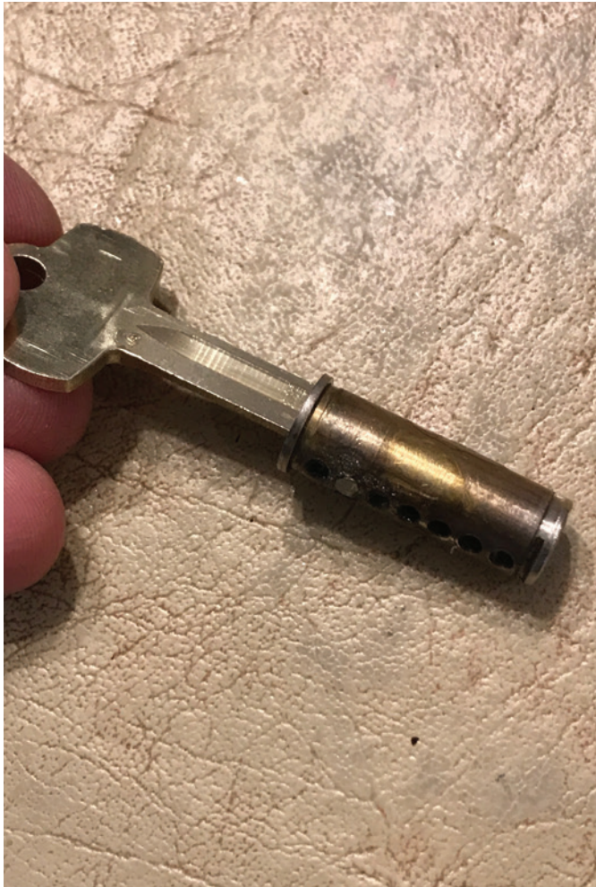
Figure 5. Pictured is something made for each member of the maintenance crew using a key blank and the plug from a discarded core.
