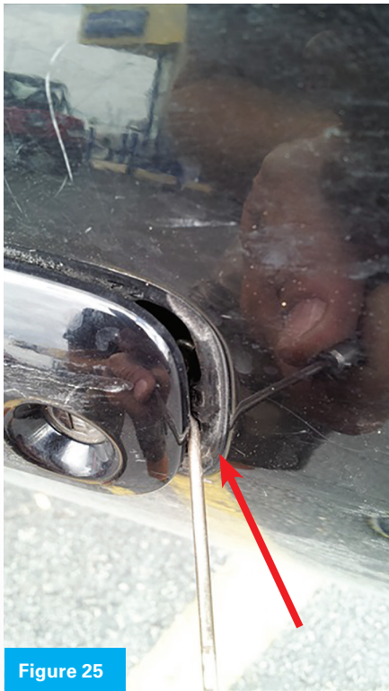
Figure 23. You will need to have a hook-type tool, such as the one shown here.
