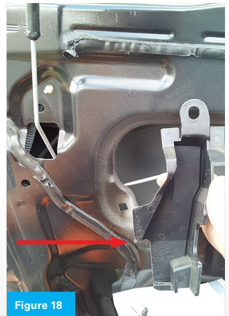
Figures 16-18. Pop these two buttons out and remove them. Then, take the plastic housing out and set aside. This is a lock rod protection piece.
