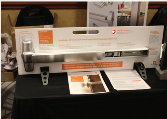
Figure 10. Von Duprin, a division of Allegion, has always produced some great exit devices, but the electronic access control technician will tell you the electric latch retraction model — or EL — can be a bit power hungry. Most electrified locks such as strikes and cylindrical locks draw or consume around 1/4 to at most 1/2 an amp to operate. The EL devices require 16 amps of inrush current. This is 48 times more energy to retract the latch, but once it's retracted, it only takes about 1/3 of an amp to hold it retracted. This previously meant a special power supply to operate the device, and special means more money. They have now come out with a motorized version that draws about 1 1/4 amp, meaning a much less expensive and far more common 2-amp power supply that can operate the exit device.
