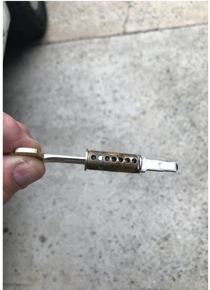
Figure 6. The author's handmade tool is especially useful for 9K Series intruder function cylindrical locks for which you need to time the cores when you put them in. Take a throw member and spread the legs apart a little. It won't drop out inside the lock while you're working, like shown here.
