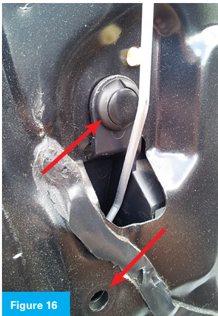
Figures 16-18. Pop these two buttons out and remove them. Then, take the plastic housing out and set aside. This is a lock rod protection piece.
