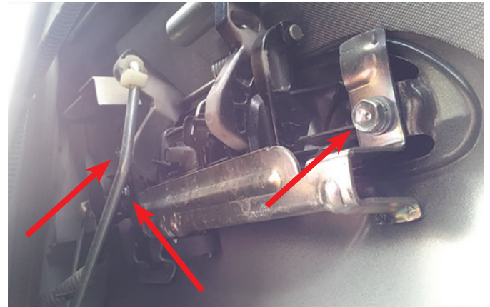
Figure 15. This will all have to come out a piece at a time. You will need to remove the screws — which hold the lock prawl actuator — that the red arrows are pointing to. You will also have to remove some bolts.
