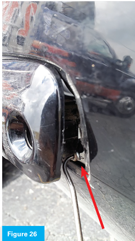
Figure 24. Spread the door handle a little more.
