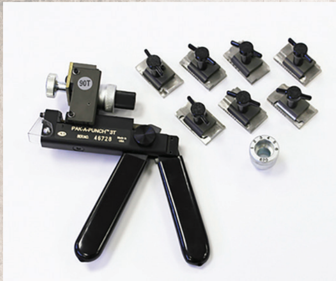
Figure 4. The A-1 Security Manufacturing Pak-A-Punch system cuts types of automotive keys, plus Kwikset, Schlage, small format interchangeable core and Master.
