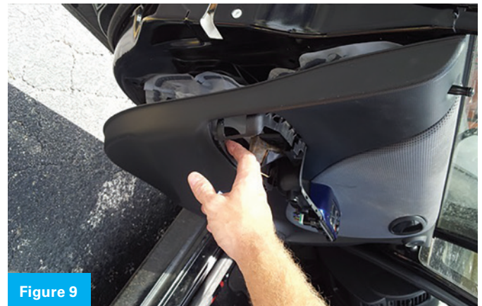
Figures 7-9. There are three screws under the armrest to remove. Then, pop the lower right corner of the panel to start removing it.
