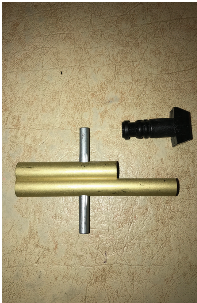
Figure 4. Depicted is a Best cylinder wrench and the black plastic piece that comes with each mortise lock.
