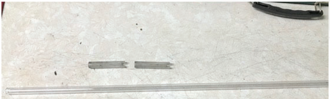
Figure 12. The author makes his own followers out of polycarbonate plastic, buying the rod from U.S. Plastic in six-foot lengths and cutting it to size.
