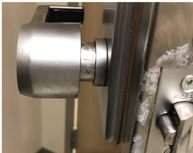
Figure 16. What looked like a retainer access hole in Figure 15 is now a bit more clearly scraped plating in the general location where the retainer access hole should have been. The metal ring must have been rotated by someone who didn't know how the lock came apart.
