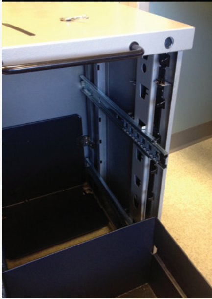
Figure 12. Here is a portable file cabinet with wheels that I opened with the assistance of gravity when the locking mechanism malfunctioned. It locked accidentally without anyone using a key to do it. There are many brands and types of office furniture at the hospital that operate mechanically in so many different ways.
