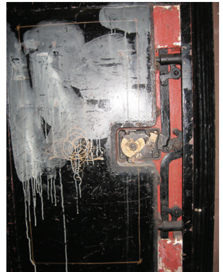
Figure 5. A drill point was selected just outside the dial ring at about 67.
