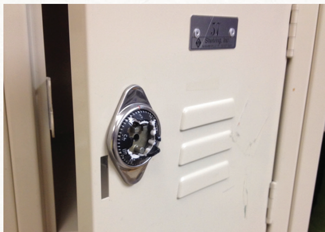
Figure 7. Here is one of the purse locker locks where the nose of the dial has broken off. Like the retractable bolt locks, the combination is dialed similarly to the lift bolt style except the final rotation clockwise will retract the spring latch if the combination was entered correctly. This lock will lock when the door is pressed inward to cause the spring latch to retract and then extend to catch into the door strike. There are at least four or five different types of lockers in the hospital in the various locker rooms, but basically three types of combination locker locks that have been installed on them. I have nowhere near been into all the locker rooms within the hospital. There are multitudes of them. We only can consistently replace broken combination locks. We have very few parts for general locker service or repair.
