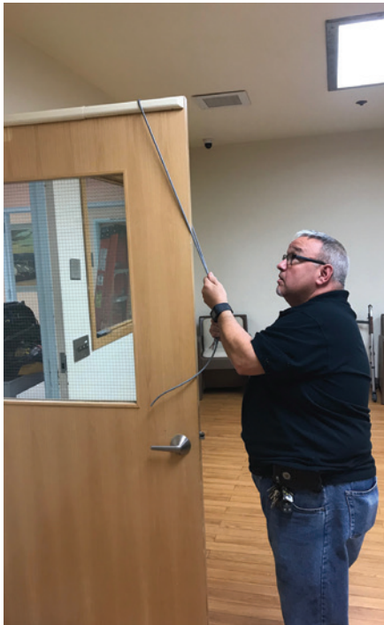
Figure 26. The author is getting ready to test the sensor by simulating a ligature thrown over the door.
