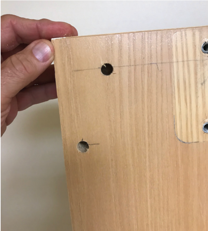
Figure 20. The bottom hole is where the wire on the hinge comes into the door, and the top hole is where it comes out and into the sensor bar.
