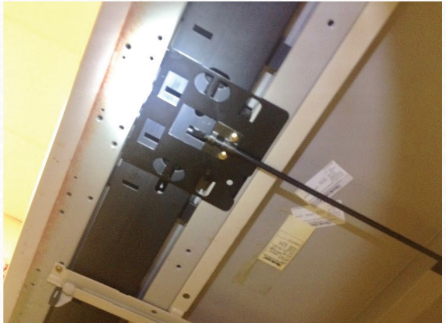
Figure 9. This is the often very uncomfortable view of the locking mechanism of a Steelcase desk from under the desk. Fitting keys to desks is often not the last part of a work order regarding office furniture. I fit the key and test it in the lock. The key turns easily, which means I cut the key properly and it turns. When the unit either doesn't lock, unlock or operate smoothly, the next step can be to trace the movement of the locking mechanism to see what's wrong.
