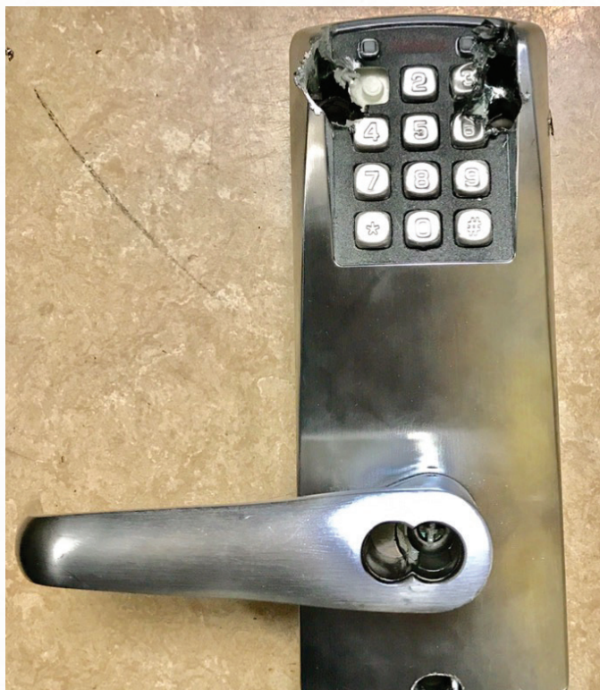
Figure 24. One of the consequences of the inside handle breaking off on a Powerplex lock is that a spring is located in the inside handle, and without the spring, the spindle can disengage. If the door closes with the spindle disengaged, it's impossible to open the door from the outside. This is the case with both entering the combination or even using the mechanical key bypass. The only option — if there is no other point of entry to a room — is to drill the lock off the door. Two holes at the top and one hole at the bottom will release the mounting screws so the lock will come off the door and the latch can be actuated manually.
