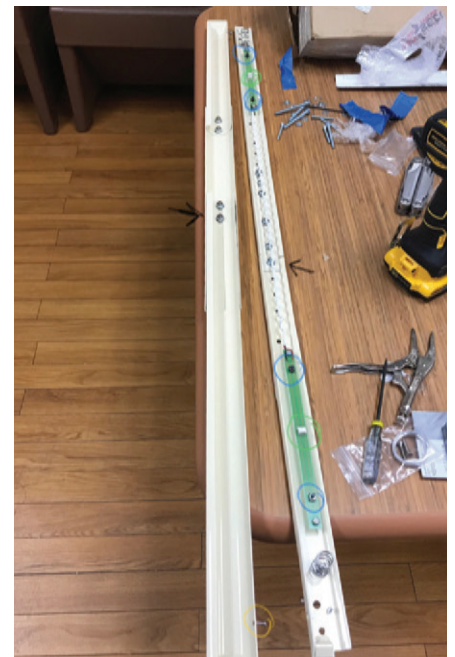
Figure 7. This photo shows the sensor bar. The black arrows point to the adjusting nuts on the bracket and cover. The cover is secured at the bottom with two screws, one of which is in a yellow circle at the bottom of the image.
