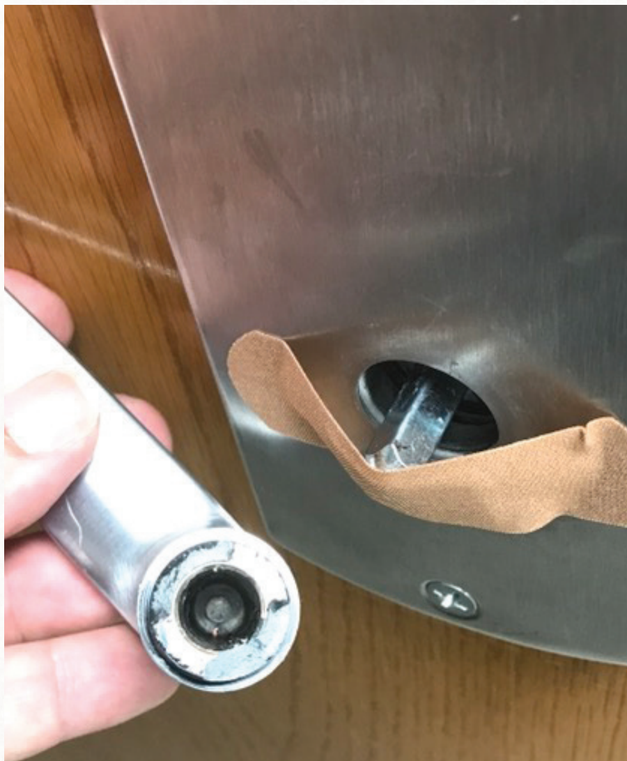
Figure 22. A much closer view gives a clearer view of the broken die cast metal at the end of the handle and the bandage holding the spindle in place.
