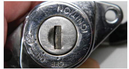
Figure 5. This dust shutter was blocked open when the ignition was received at the shop, which made reading easy.
