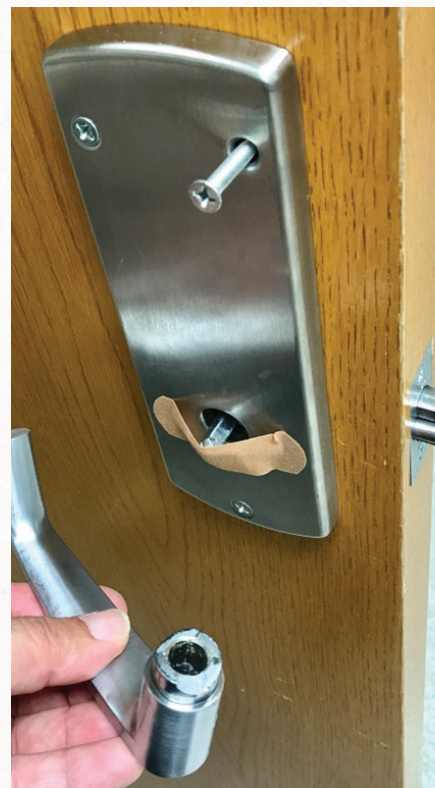
Figure 21. This is the inside handle assembly for a Powerplex electronic keypad lock. The die cast metal at the end where it engages the inside plate broke off, allowing the inside handle to come completely off the door. Being in a hospital, it's appropriate that a bandage is holding the spindle piece from coming out.
