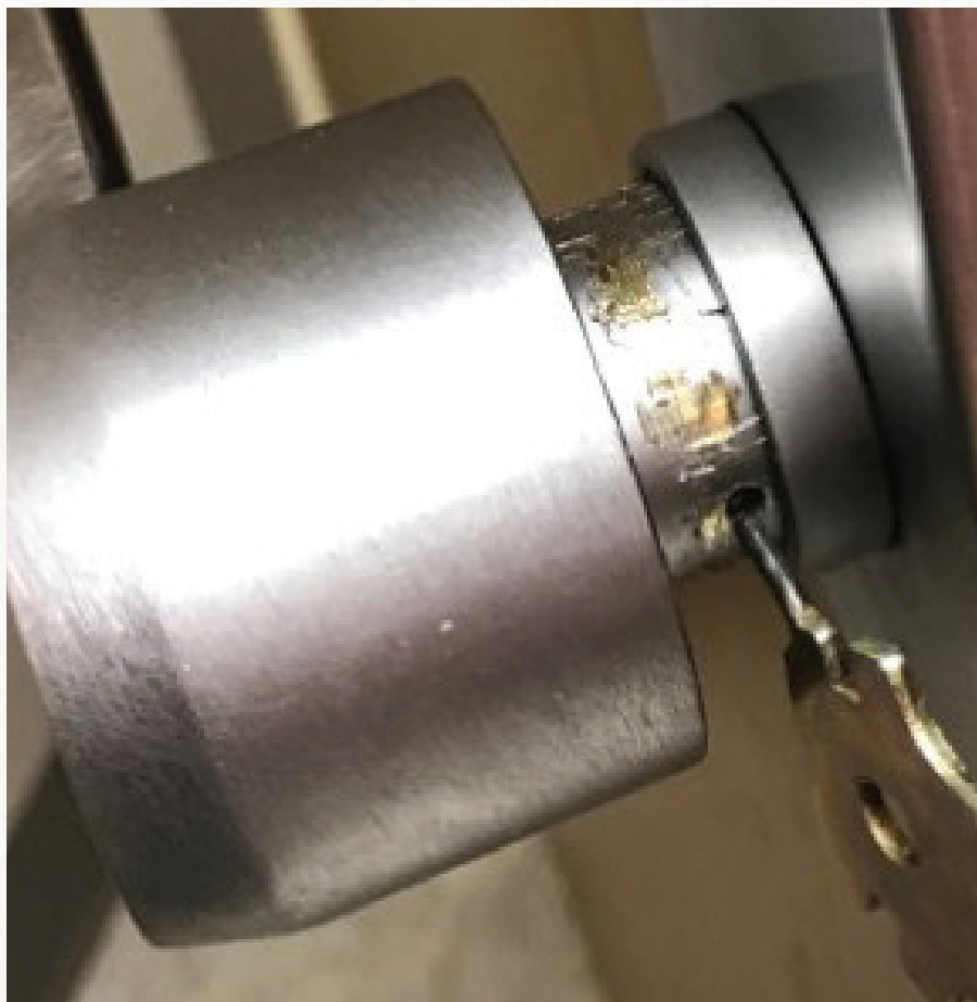
Figure 20. A slightly closer view shows the tool about to engage the retainer. This was a slight inconvenience when someone made a previous attempt to service the lock and apparently didn't quite know what he was doing. Sometimes it can be a lot worse.
