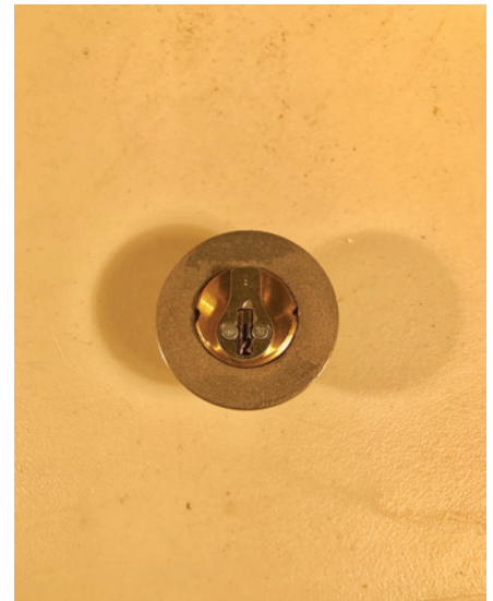
Figure 10. The cam on the cylinder is a standard Yale-type cam.
