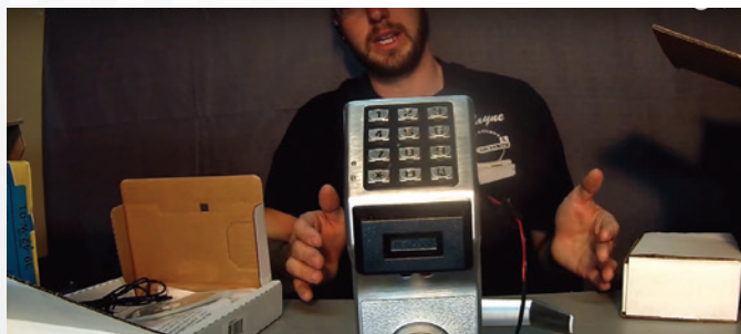
Figure 7. The Alarm Lock PDL 3000 allows the use of prox cards or fobs to access the lock.
