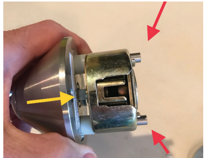
Figure 31. You can see the outside spindle between the grey spacers (yellow arrow). The red arrows point to the studs that the backplate screws into.
