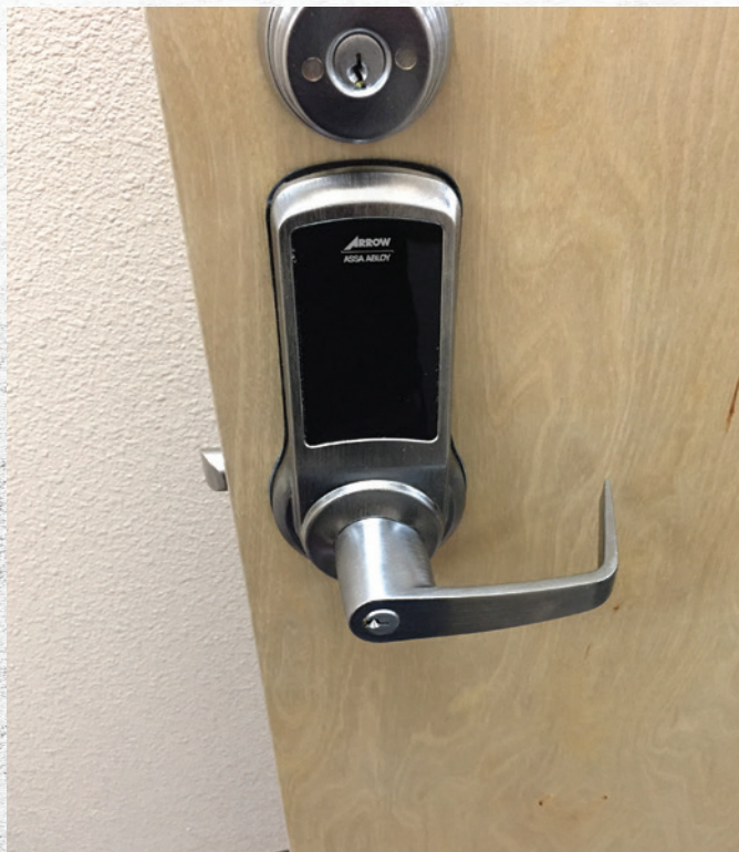
Figure 10. The outside keypad does not display any numbers when idle.
