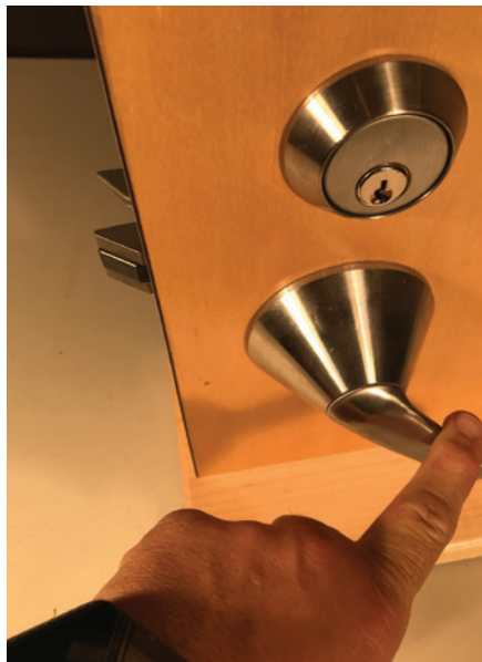
Figure 5. The author is pushing down the outside lever; note that the latch did not retract.
