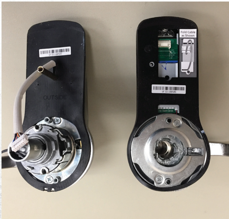
Figure 4. In this photo is the backside of the inner and outer halves. Two things to be careful with during installation: First, the upper cable and lower cables need to not be pinched between the lock and the door. Also, during installation of the lock, ensure the rubber gasket is seated between the lock and the door correctly.
