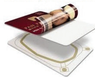
Figure 4. Prox cards, or “contactless smart cards,” contain a chip and a coil of wire, which acts as an antenna.
