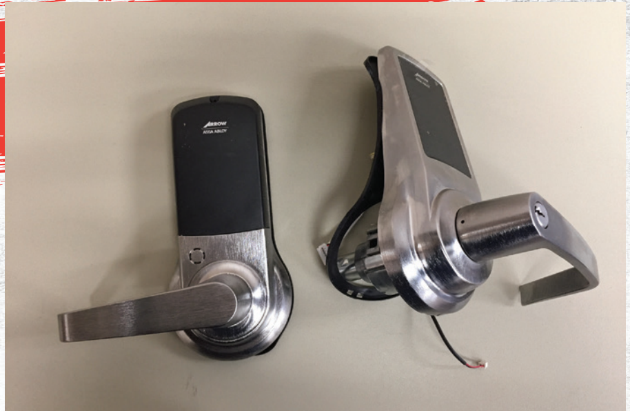
Figure 3. This image depicts the front and back halves of the lockset. The only additional disassembly is the same as most locks: remove the inside lever and trim to install the spring cage first.
