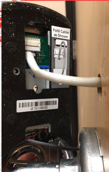
Figure 7. The two cables need to be plugged into the inner housing, and the upper cable is routed or folded as directed according to the diagram on the back of the lock.
