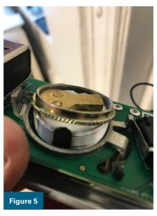
Figures 4 and 5. Shown is a gold-colored ring with a knurled edge on it as it was installed and then after the author unscrewed it.
