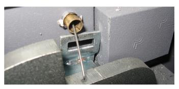
**Figure 10.** The tubing allowed the wire to be inserted all the way into the door, keeping the bend in it so it would drop down as soon as it exited the tube.
