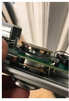
Figure 7. The gold ring is right-side up and about to be tightened down.
