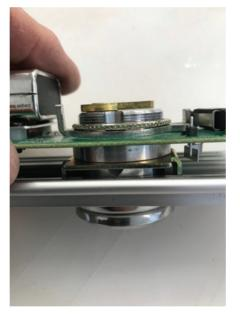
**Figure 8.** Both rings are properly installed; you can see a slight space between them, allowing free movement.
