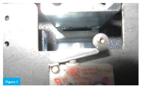
**Figures 1-3.** On these safes the relocker "dangles" from a block attached to the lock bolt. (*Figure 1* is from another safe, but it shows the relocker in its correct position.)
