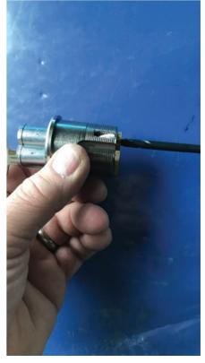
Figure 17. The drill bit is in the cylinder.
