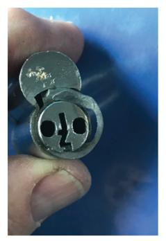
Figure 18. This photo shows the deformed clip that caused an issue.
