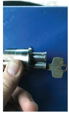
**Figure 15.** The customer had to force a core in, and it then was extremely difficult to turn and could only be halfway removed.
