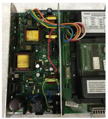
**Figure 5.** The power supply for these controls is essentially a computer power supply that offers multiple output voltages. The power supply provides 5 volts, 18 volts, lock power and battery power all from the same unit. The ribbon cable from the front panel plugs into the top of the motherboard. There is a coin cell battery to maintain programming when the AC power and backup power is removed.
