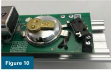
**Figures 9 and 10.** The author's finger is moving the silver ring from the deactivated position to the activated position.
