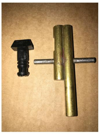
**Figure 2.** Fixing the issue of the cam dropping down requires some white lithium grease and some type of tool such as a Best cylinder wrench or the black plastic tool that comes with Best mortise locks, both shown in this image.
