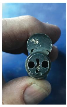
Figure 20. The replacement clip is in place.
