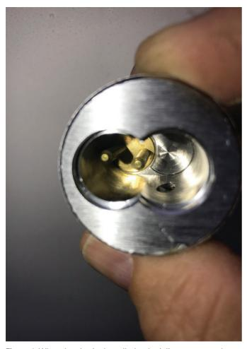
**Figure 1.** When the pins in the cylinder don't line up as seen in this photo, the core won't go in.
