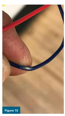
**Figures 12 and 13.** Figure 12 shows how much wire was packed inside the bar, and Figure 13 shows how the wire was damaged by contact with moving parts.
