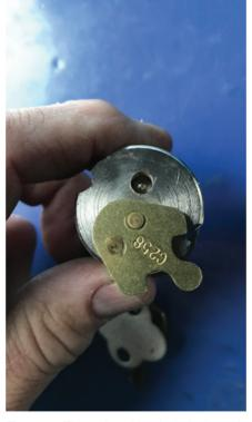
**Figure 16.** The author drilled a hole through the back of the cylinder so he could attempt to push the core out the front.
