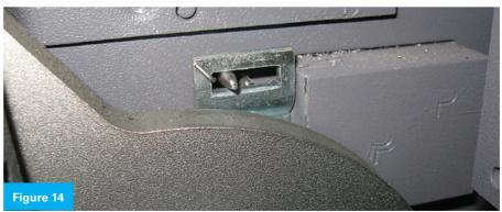
Figures 13 and 14. A probe tool was used to finagle the relocker up enough to allow the handle cam to turn.
