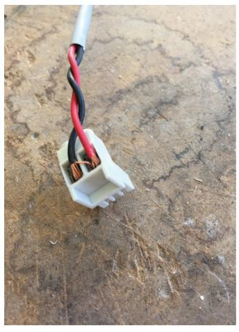
**Figure 8.** This is an example of why you need to recheck all wiring prior to applying power. I intentionally left a strand loose for the photo, but I have had this happen to me on the job.
