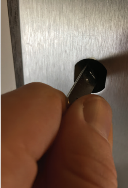
Figure 5. Insert the spanner wrench fully into the combination sleeve and carefully turn the spanner wrench clockwise to the stop position (you should hear and feel it click into position). After the click, turn the spanner wrench counter clockwise until it stops, and remove.
