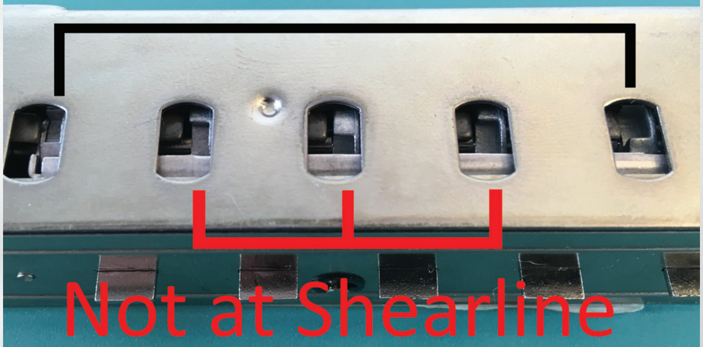
Figure 13. The goal of the decoding process is to align all gates with the unlocking slide; KABA refers to this as a “shearline.”
