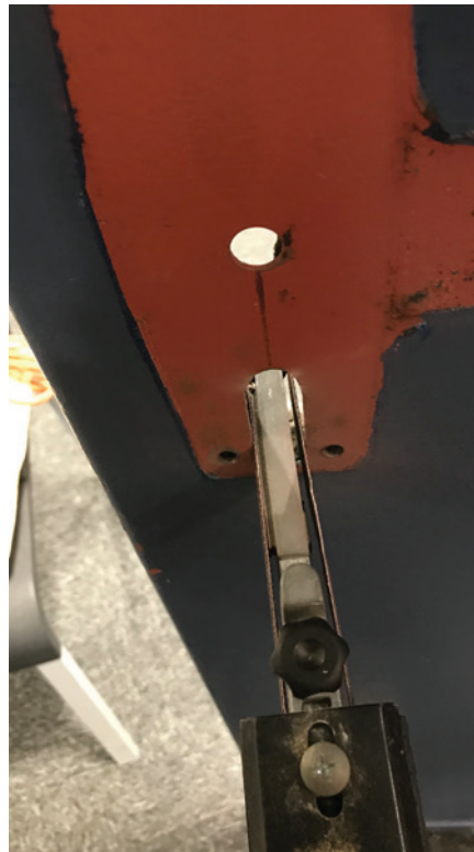
Figure 12. This image shows how the author was able to widen the cutout so the new trim would fit.
