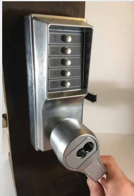
Figure 9. Turn the outside lever fully once more. The latch should not retract. If the latch retracts, however, a step was either missed or not followed properly, and the lock is in zero combination. Follow the entire procedure again except for the step in Figure 4.
