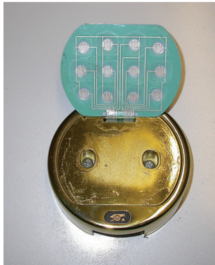
Figure 3. The membrane can be removed by gently peeling the bottom of the keypad up from the mounting base to expose the two mounting screws.
