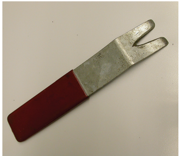
Figure 14. The back panel seemed to be held on with some sort of plastic push nut. A door panel removal tool worked perfectly.
