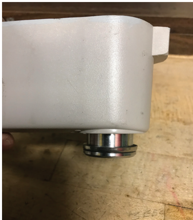
Figure 2. The large nut holding the cylinder in is extremely loose.
