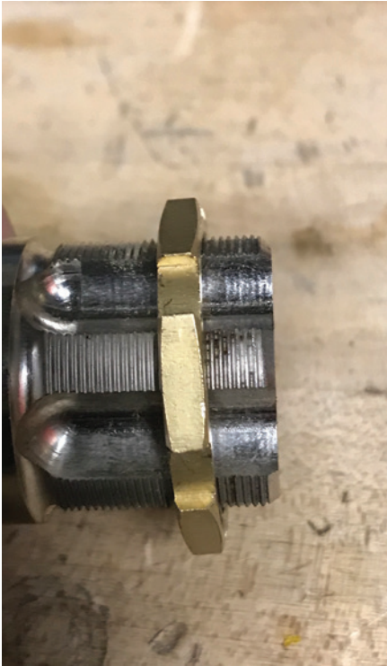
Figure 3. The nut is on a cylinder tap made by HPC. The hole in the nut is slightly bigger than normal.
