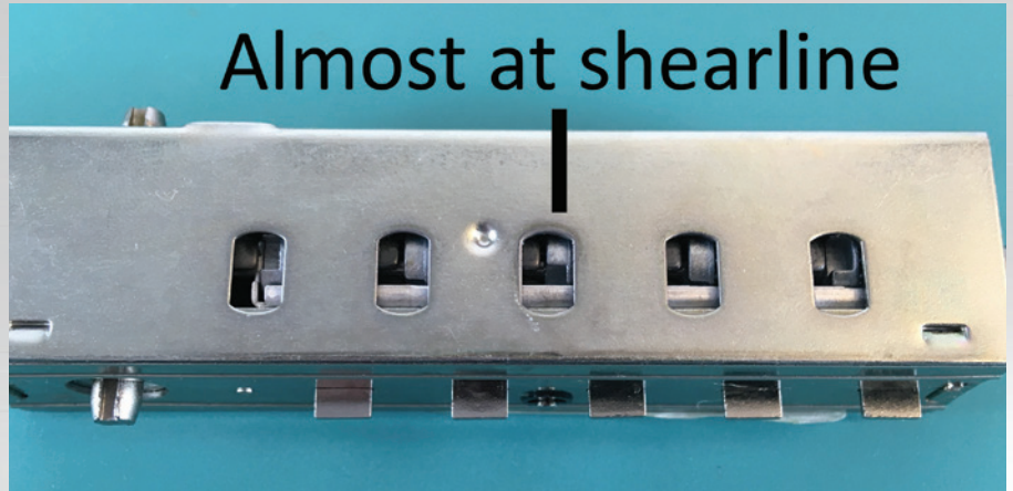
Figure 14. The gears almost at the shearline, but not directly under it, are the last used in the combination.
