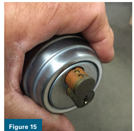
Figures 13-15. To remove a small format IC core intact, get to the back of the core (Figure 13), put pressure on the locking dog, and try to pick it (Figure 14). The result is shown in Figure 15.
