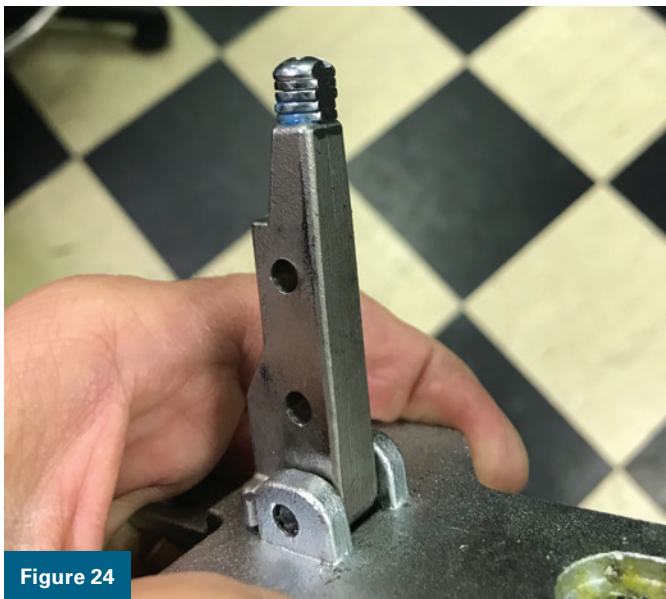
Figure 22. This image shows an innovative way someone replaced a broken lever using a welder.
