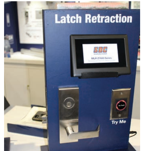
Figure 30. Electric latch retraction has been common in exit devices but not so common in mortise locks. Instead, the lock's outside handle was released or unlocked and still required the person to turn the lever or knob. SDC designed this mortise lock with electric latch retraction, allowing for it to be mated to a power operator when actuated and not require use of an electric strike.
