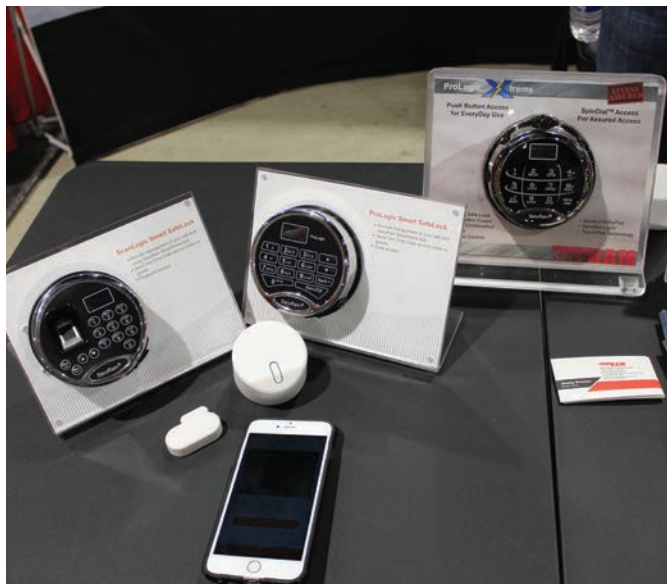
Figure 33. IoT — or Internet of Things — is fast becoming the normal in our society. Anything that can be controlled remotely and connected to the internet is part of the IoT, and that includes electronic safe locks. SecuRam offers Bluetooth-based locks that can be controlled from anywhere in the world via the internet or at the safe. The technology also allows them to offer wireless contacts that can be mounted to doors, windows or anything else you dream of to allow end users to monitor them with the same app on their smartphones.
