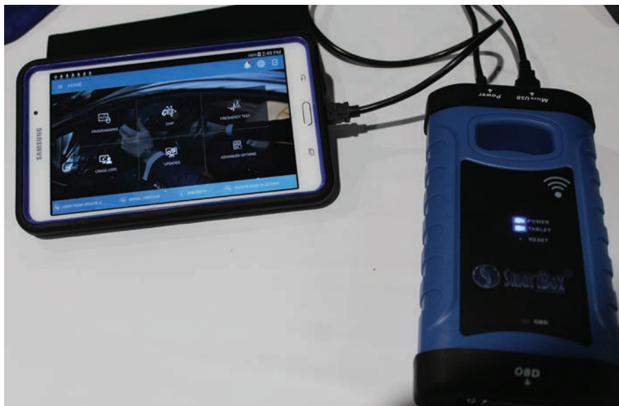
Figure 11. Automotive locksmithing has become its own specialty. The days of mechanical keys to operate our modern vehicles are long gone. Lots of different tools and equipment are available to program transponder keys and remotes. The SmartBox for auto key programming has been around for a few years, and it will program 95% of the transponders and remotes of vehicles on the road today. They will soon be offering even more features with remote key and FOB unlocking.
