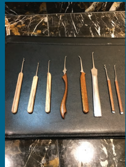
Figure 24. ALOA member Mark Snead of Ohio showed me his impressive homemade picks last year at the convention, but I didn't take pictures then. Shown here is a sample of his work, which he does for his personal use and not for sale. The three on the left aren't done yet. The five on the right are made from a kitchen knife, a Sawzall blade and spring steel. They look and feel great in your hand. 🤖
