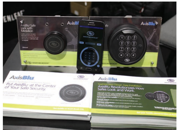
Figure 34. S&G is most well known name in safe locks. Introduced to locksmiths and safe technicians this year at the Security Expo is their AxisBlu line of safe locks. The locks are paired to your phone and don't even require anything on the outside of the safe. The only thing you may see is the medallion, which covers the emergency power connection for a 9-volt battery in case someone ignores the low battery warning. If you are more comfortable with a keypad and external battery, they offer that option. The lock is based on their Titan series swing bolt, but if you need it to be a traditional square bolt, they can make that — if you need enough of them, or a safe manufacturer decides to.
