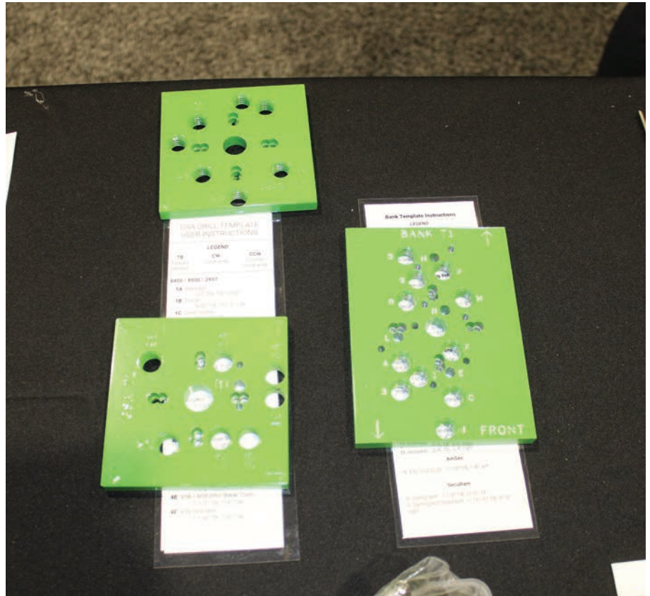
Figure 10. Many technicians prefer a fixed rig for drilling safes. Fixed rigs use templates, and TimeMaster has several different plates or templates for GSA and bank vault locks.
