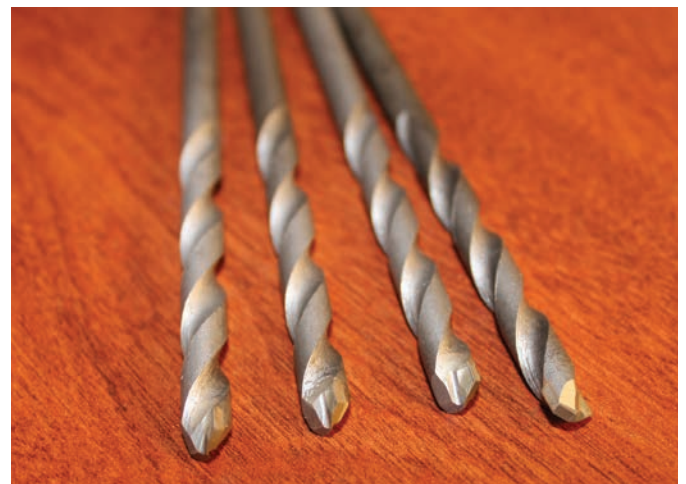
Figure 8. Ryan has drilled his share of safes and decided to make a different bit with a lightly different geometry and carbide to add to the safecracker's arsenal. No one bit will cut all hardplate, and we all have different styles of drilling. It is important to have a variety of carbide bits. If your bit of choice stops cutting, try a different one. Ryan's Boss bits offer a great alternative.
