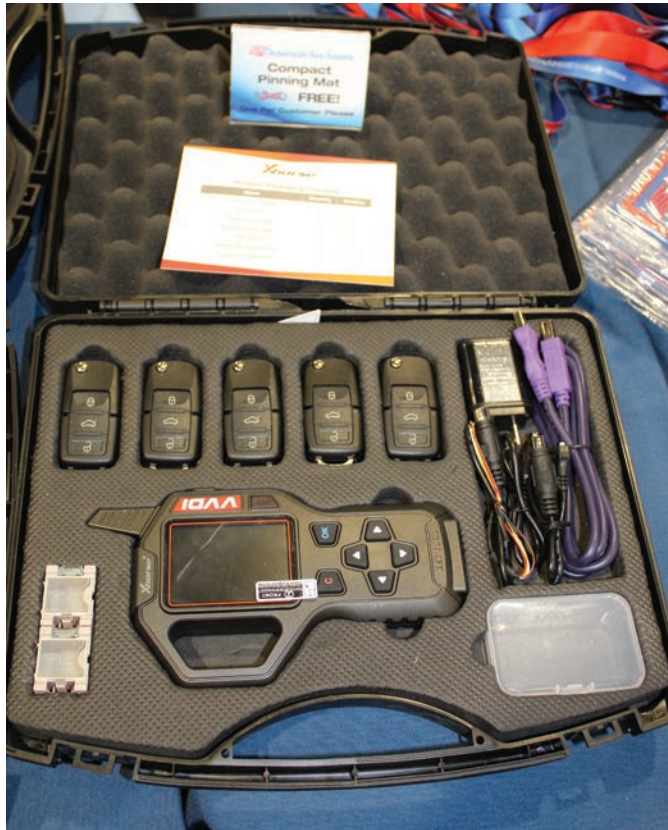
Figure 13. Another tool for the automotive locksmith is from XHorse. This tool can reduce your inventory by programming special remotes to the FCC number needed for specific vehicles — in many cases, at a lower cost than the factory-original remote. This is great for field techs to be able to carry the tool and a few remotes. They can generate new remote fobs and remote head keys with minimal inventory, possibly saving a trip back to the shop for the “right” one or having to carry a lot of inventory in the truck.
