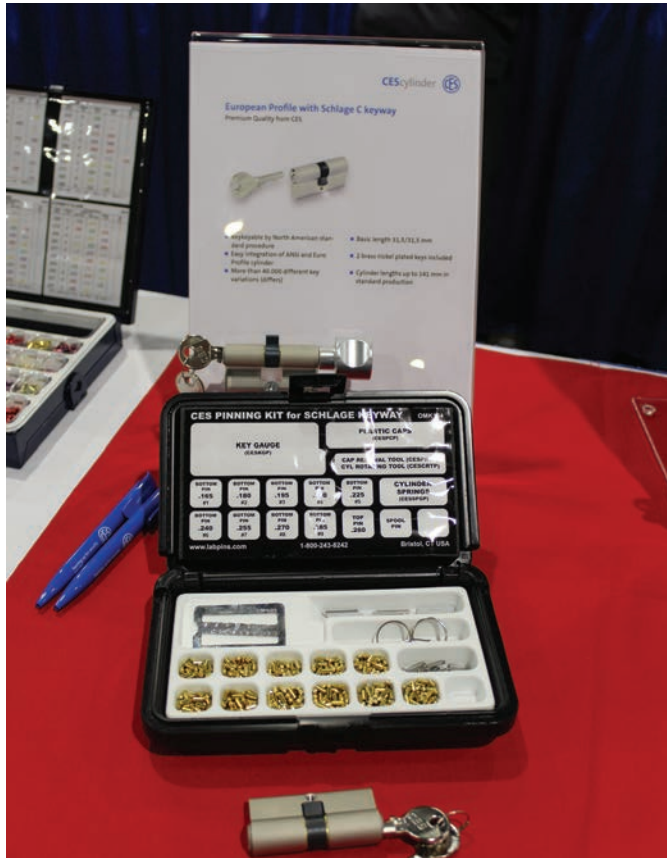
Figure 20. Lab has been producing great-quality pins and tools for many years. This year, they introduced a profile cylinder pin kit for the locksmith. It includes the plastic caps common on the Hoppe cylinders.
