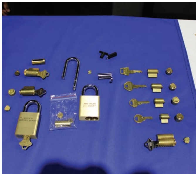
Figure 46. American Padlock made our life easier and lowered our inventory when they introduced the American 3650 multi-platform cylinder system. Most of us are familiar with the 3600 line that accepts the common key-in-knob cylinders. They took that idea to a new level with the new design. Not only can it take the KIK cylinders, but it also takes Master padlock 4-, 5- and 6-pin cylinders; American padlock cylinders with the correct adaptor sleeve; and the Abus 83 series cylinders, all with the appropriate cam. They even made the shackle easy to change in the field with a couple of little tools.
