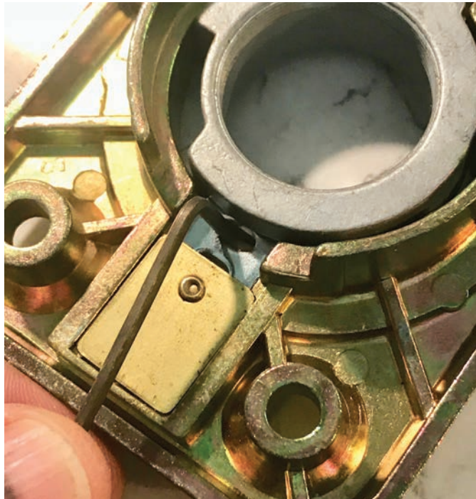
Figure 15. The Allen wrench, supplied with the lock, is inserted into the spring-loaded tab, ready to pull it back.
