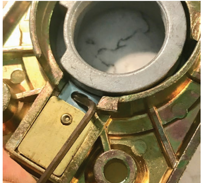
Figure 16. The tab is out of the slot, and the cylinder holder is ready to be rotated out of the back plate. After that, the inside escutcheon could be removed to expose the four ¼-20 machine screws that hold the lock together. Once the outside plate is removed, you can reach the setscrew holding that cylinder in.
