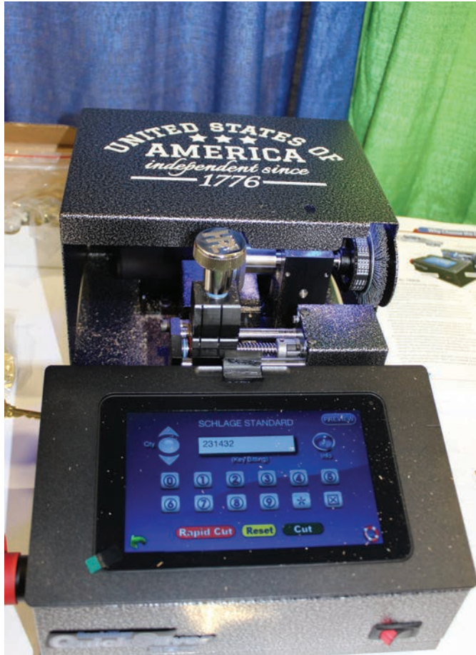
Figure 4. The HPC QuickSilver code machine is an extremely fast code-cutting machine. This machine takes longer to load the blank and unload the cut key than it does to actually cut the key.
