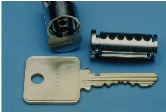
Figure 8. In this picture, the EMK (with ward cut) are aligned together with the cut-out on the plug. The ward in the shell can be clearly seen.
