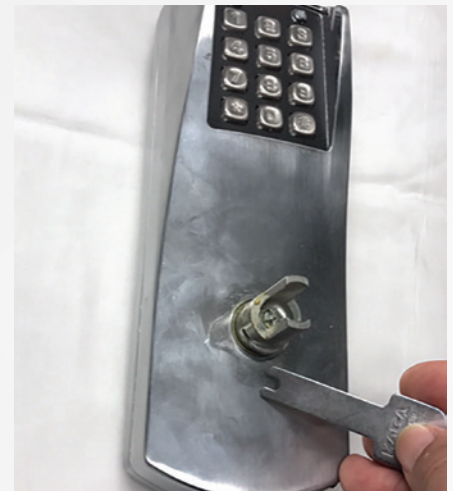
Figure 3. A special notched tool points to the handle retainer extending below the drive tube.
