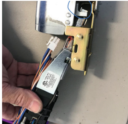
Figure 14. The blue circle shows the hooked end of the MLR being placed behind the L-shaped piece.
