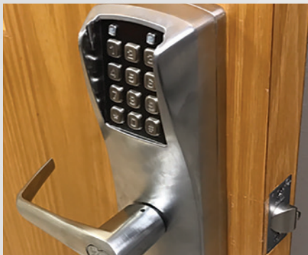
Figure 1. The keypad of the lock is like a telephone keypad. It has 10 numerical digits and the "*" and "#" keys for programming. There are two LEDs at the top of the keypad. The lock core (or lock cylinder in the non-IC versions of the PowerPlex) acts as a mechanical key override.
