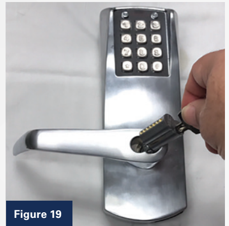
Figures 18 and 19. Turning the control key 15 degrees clockwise will draw in the lug ( Figure 18 ) and allow you to place the core into the housing ( Figure 19 ).
