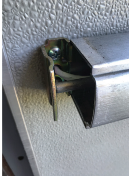
Figure 5. This image shows the end bracket and how the wire passes through it.
