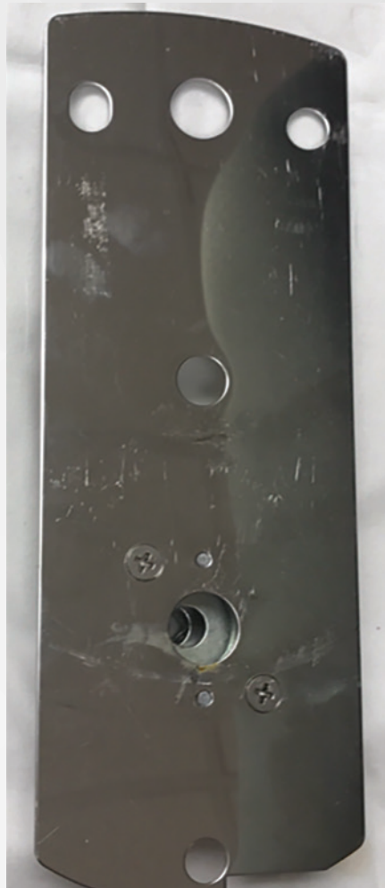
Figure 25. This part comes from the factory left handed but can be quickly and easily converted to right hand by turning it around and removing the two exposed Phillips-head screws. The metal plate can be reversed up for down and the screws reattached in the opposite holes.
