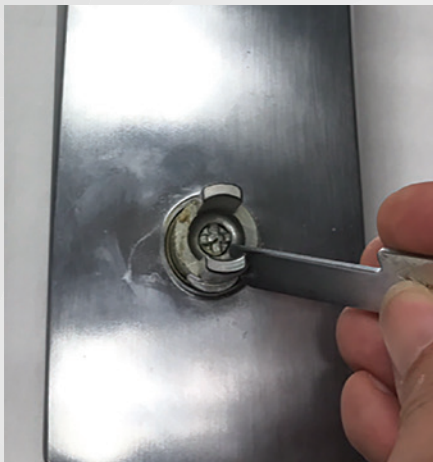
Figure 4. A cross-shaped part shows in the middle of the drive tube. That part will be rotated with the special tool to engage and disengage the retainer.
