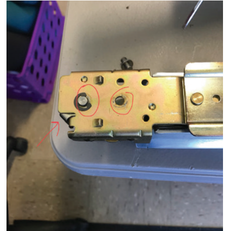
Figure 12. The back of the bar is behind the dogging device. The two circles are the two E-clips that hold it on, one of which has been removed.
