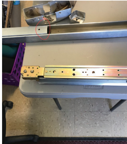
Figure 11. The cover is removed, and the red circle shows the hole for the Allen wrench used to dog the bar open.
