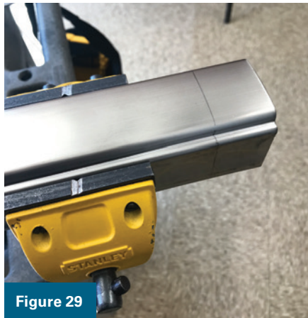
Figures 29–31. These photos show the cover marked and in a swivel head vise, the Skilsaw with a Diablo cutoff blade, and the author getting ready to cut it.
