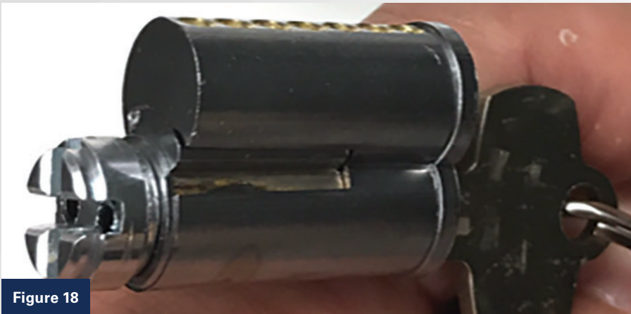
Figures 18 and 19. Turning the control key 15 degrees clockwise will draw in the lug ( Figure 18 ) and allow you to place the core into the housing ( Figure 19 ).
