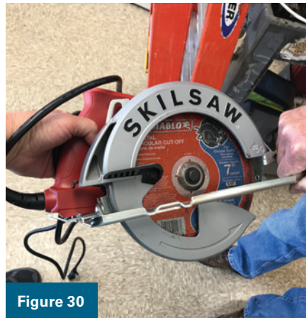
Figures 29–31. These photos show the cover marked and in a swivel head vise, the Skilsaw with a Diablo cutoff blade, and the author getting ready to cut it.
