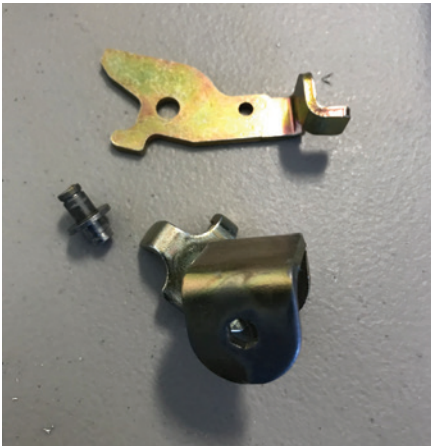
Figure 13. Shown are the removed parts that make up the dogging device.
