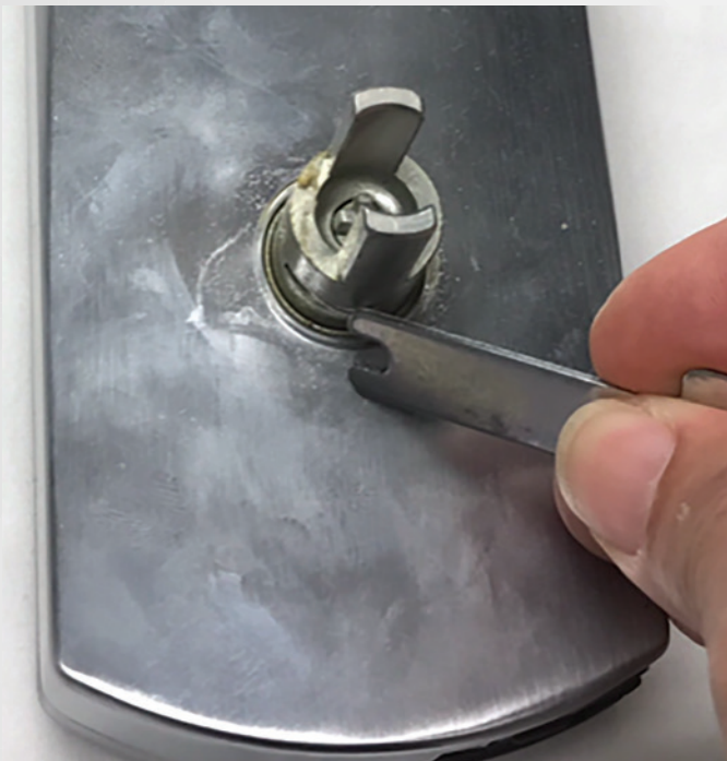
Figure 8. With the part fully rotated clockwise, the retainer is movable and can be pushed upward to accept the handle.
