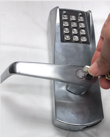
Figure 20. Once the core is all the way into the housing, you can turn the control key counterclockwise to extend the locking lug and hold the core within the housing.
