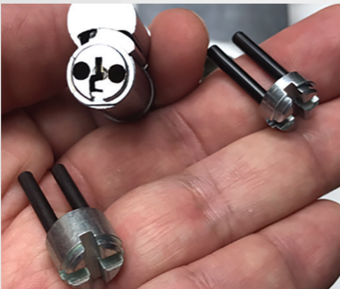
Figure 14. Shown is a back view of a core and the thicker 6-pin core tailpiece adapter at the left and the thinner 7-pin core tailpiece.
