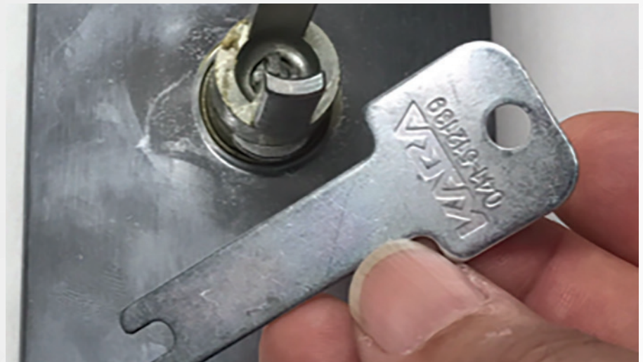
Figure 5. You can see how the shape of the notch can engage the cross-shaped part, and you either rotate it clockwise to extend the retainer or counterclockwise to release it.
