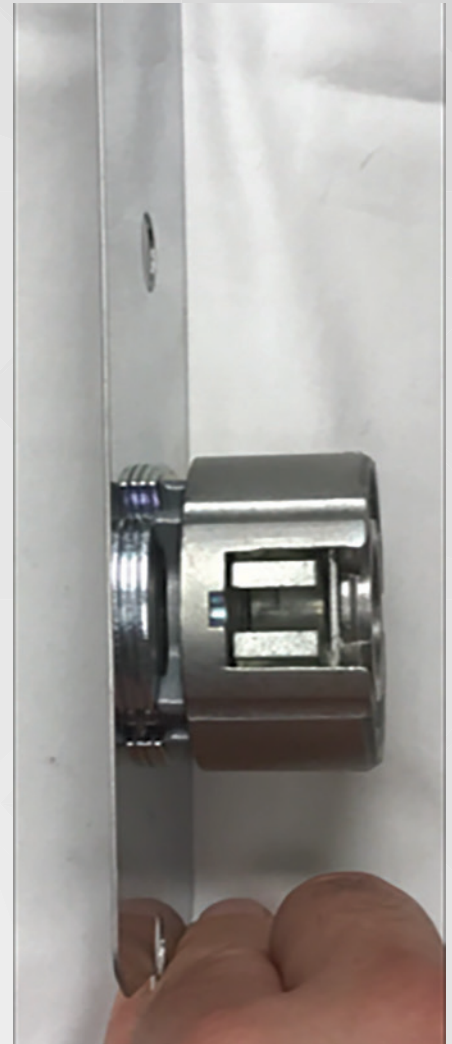
Figure 26. The gripper part that engages the latch can be seen from the side view. The interior handle assembly has to be handed too. It also can be either left or right handed.
