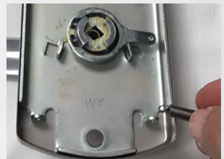
Figure 28. The spring is being attached on the right side of the unit to make it left handed. Putting the spring on the left side makes it right handed.
