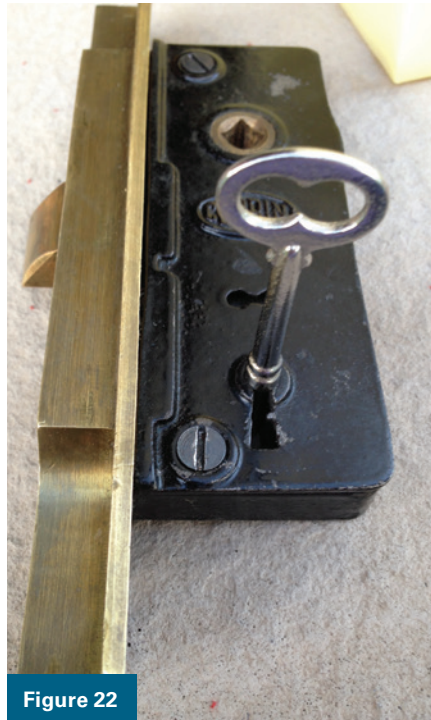
Figures 20-23. These images show the front and back of the working key and the bolt thrown by the key and also retracted.
