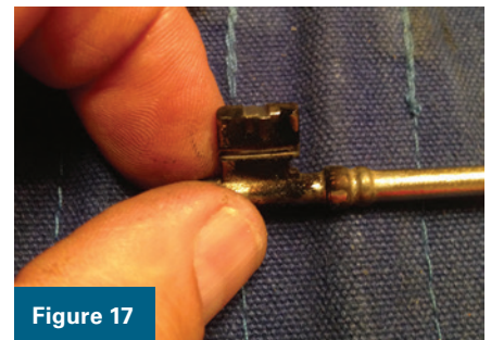
Figures 16 and 17. These photos show the re-smoked blank and the soot removed by filing the cuts.
