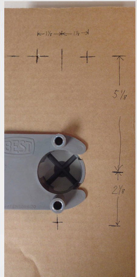
Figure 4. The jig is positioned in the 2 1/8" diameter hole in the cardboard template.
