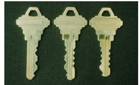
Figure 13. Notice that the ward cuts at the bottom of the blade are necessary on the control key and EMK.
