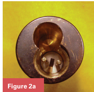
Figures 2a and 2b. Both of these pictures show the Sargent LFIC hotel function Housing. Figure 2a has no shot pins visible, and Figure 2b has only one shot pin visible.
