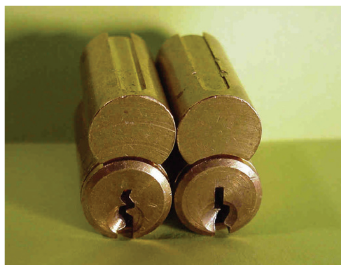
Figure 21. This image shows the front view of the core with Lockwood and Schlage keyways.
