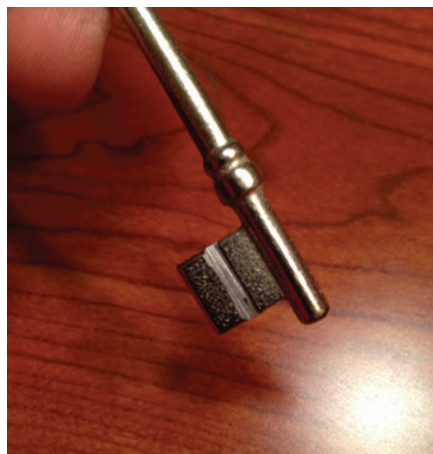
Figure 4. The shown cut will allow the blank to bypass the side ward and go into the lock.
