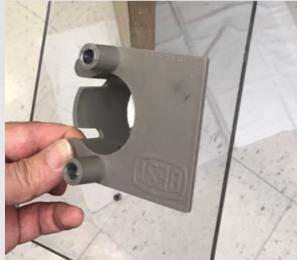
Figure 6. The plastic jig fits inside the Plexiglas template the same way it fit into the cardboard template.
