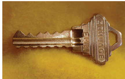
Figure 12. A side view of the Schlage Hotel EMK shows the undercuts to bypass the ward rings.
