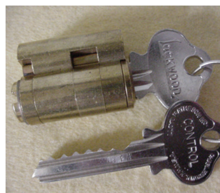
Figure 24. The Lockwood operating key is inserted into the ILCO bypass core, with control key steadfastly at its side.
