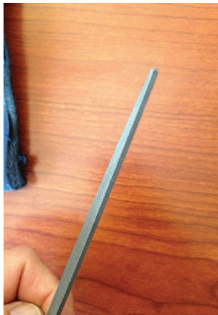
Figure 2. This photo gives a close-up view of one of the warding files.
