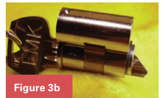
Figures 3a and 3b. These two images illustrate an operating key inserted into the first core. Figure 3b shows an EMK with extended tip pushing farther outward.
