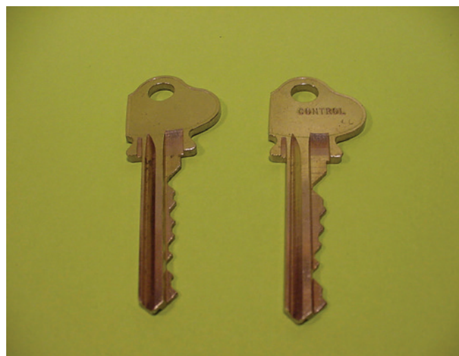
Figure 19. Notice how the bow of the EMK must be shaved off to turn and bypass the bottom of the escutcheon.
