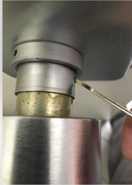
Figure 10. Angling the tip of the spanner wrench away from you is the quickest way to depress the retaining clip and allow the insider level to slide in place.
