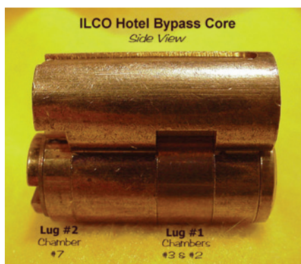
Figure 22. Note the placement of the two separate control lugs. This is unusual for any core.
