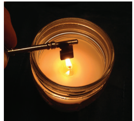
Figure 14. The author is using a candle to coat the blank with soot.
