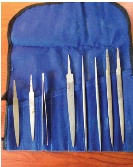
Figure 1. The three files on the left are warding files, and Figure 2 is a close-up of one of them. The four files to the right are two round files, often called “rat tail,” and two “Pippin” files.
