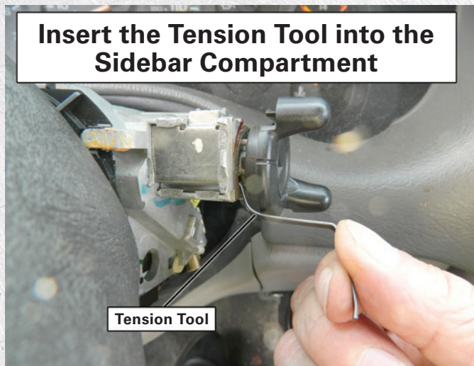
Figure 7. Tip the tension tool down to slip the tool into the front of the sidebar compartment.
