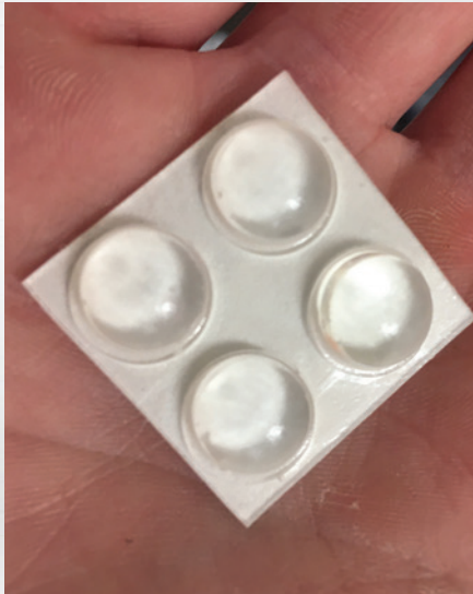
Figure 12. If the deadlock plunger enters the strike, use the provided rubber bumpers (shown) to push the door away from the strike and allow for proper latch/strike alignment.
