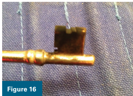
Figures 16 and 17. These photos show the re-smoked blank and the soot removed by filing the cuts.
