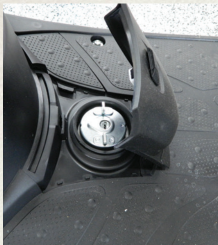
Figure 2. The gas cap is found under a non-locking lift-up cover in the floorboard of the scooter.
