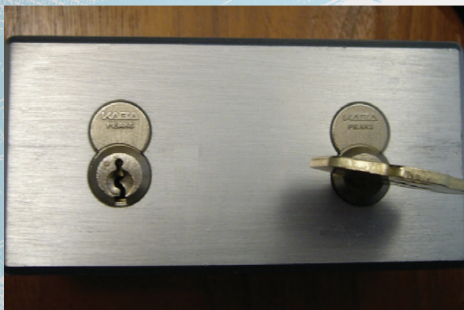
Figure 32. The Peaks SFICs is being tested within a Key Retainer Device (KRD).
