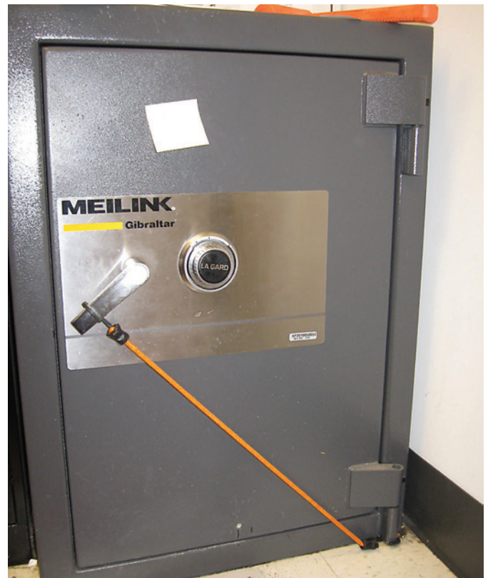
Figure 2. A bungee cord was attached to the handle to hold the rest of the bolts in a retracted position.
