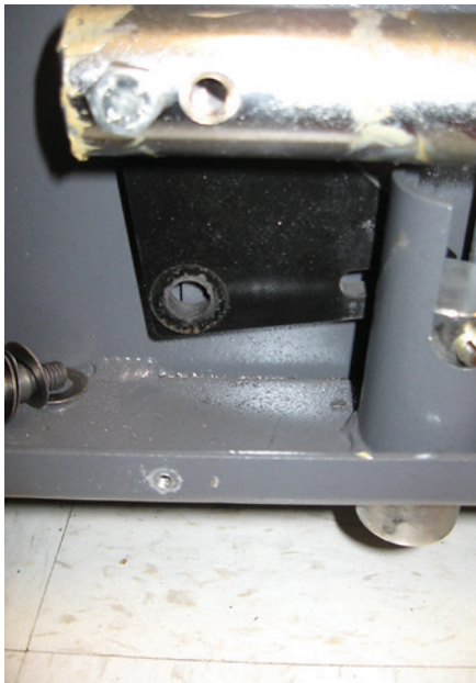
Figure 9. The bolt that holds the bell crank to the door loosened up and fell out.
