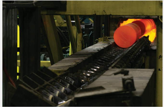
Figure 5. The brass is formed into rolls as it cools and later gets pressed into strips.
