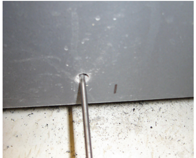
Figure 6. A Jerry Forder probe was inserted into the hole and pried up a little.
