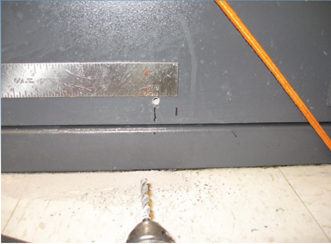
Figure 3. Drilling was done at 11" from the opening edge of the door and 1" up, starting with a 1/4" bit, then a 5/16" bit for more prying room.
