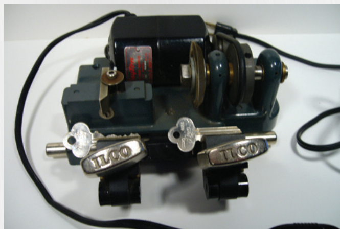
Figure 33. This Ilco KM190 key duplicator is now obsolete but still working.
