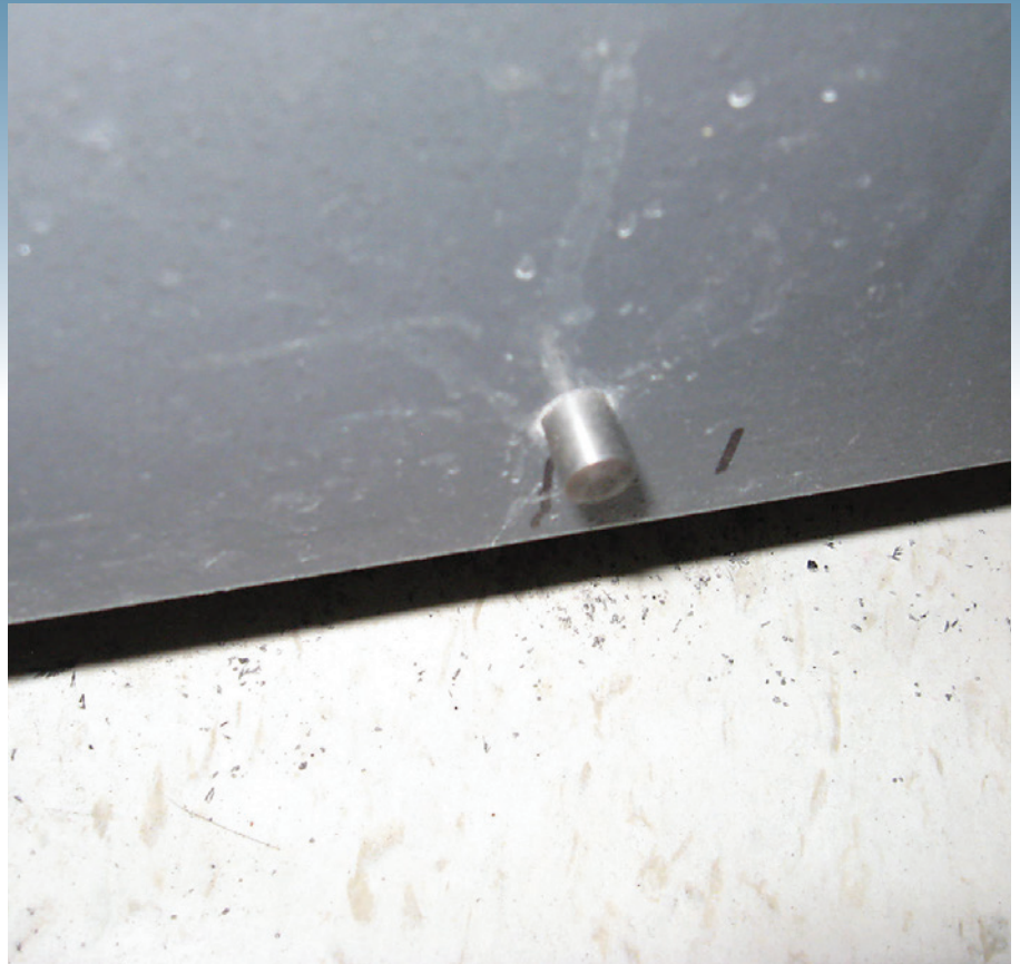
Figure 12. The hole was plugged with a taper pin and Dremelled off flush.
