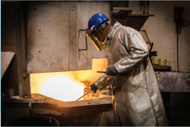
Figure 4. The brass furnace runs 24/7 to melt the brass to a molten state.
