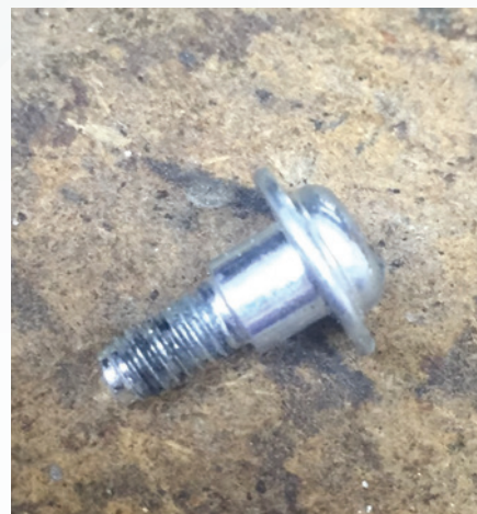
Figure 16. The four screws that hold the plastic to the lock housing are all shouldered to prevent crushing the plastic.
