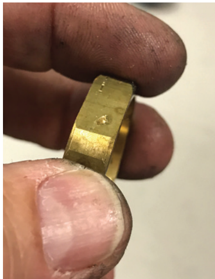
Figure 24. This photo shows the marks made by the author's awl as he loosened the cylinder nut.
