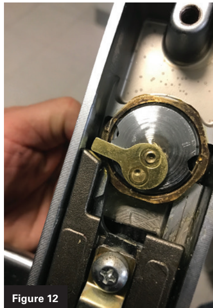
Figures 12 and 13. The cylinder cam is pushing down a slide inside the trim and then lifting it up.
