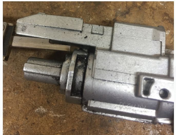
Figure 9. Use a caliper or another method to measure the location of the roll pin to transfer that measurement in to the channel where the key buzzer arm sits.
