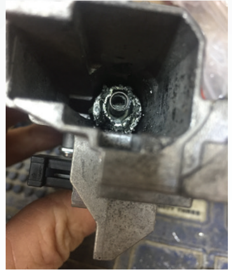
Figure 7. Sometimes the spring stays in the housing. Other times, it stays in the back of the plug.
