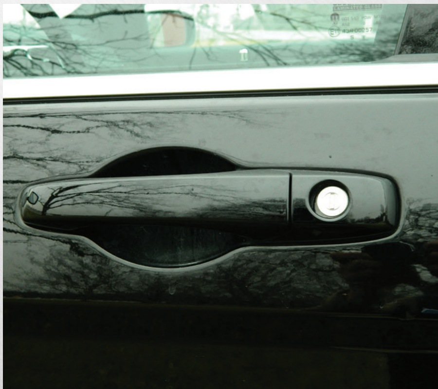
Figure 3. The door cylinder is incorporated into the pull handle trim.
