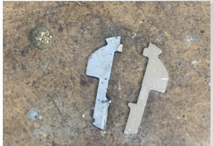
Figure 13. The second tumbler from the lock is on the left and is missing the tab. This is the reason why it was sticking up.
