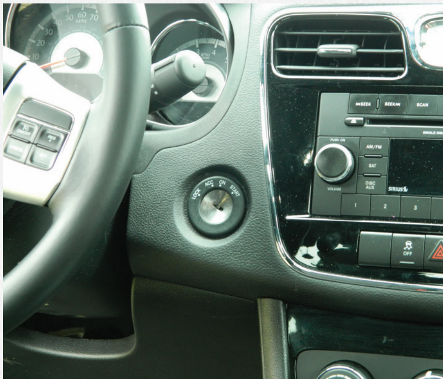
Figure 2. The ignition lock cylinder is mounted in the dash at the right side of the steering column.
