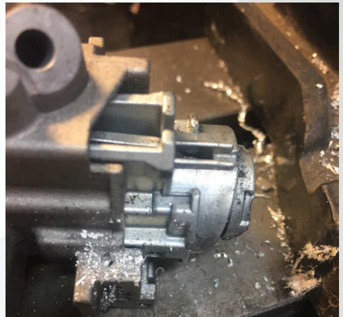
Figure 5. The housing was drilled slightly offset to the pin. When the drill bit touched the pin, it pushed it out of the housing, and the cylinder popped out.
