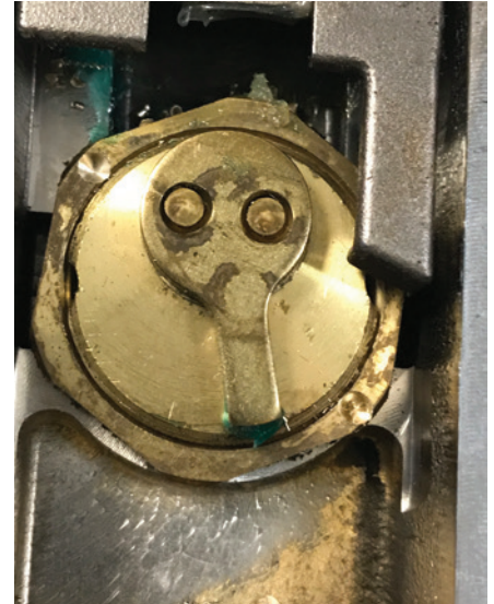
Figure 16. The author drilled two small, shallow holes in the nut.
