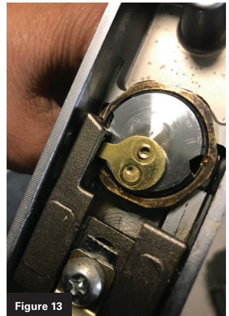
Figures 12 and 13. The cylinder cam is pushing down a slide inside the trim and then lifting it up.
