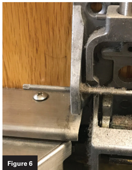
Figures 5-7. These photos show the author using a thin awl to tap the pin out, the pin partly out and where he left it, still attached but out of the way.
