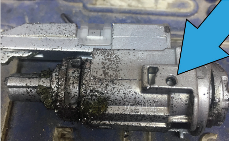
Figure 6. The lock cylinder has been removed. This is the cavity where the roll pin retains it.
