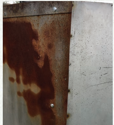
Figure 23. The hinge is secured using 10-24 carriage bolts through the side of the main unit.
