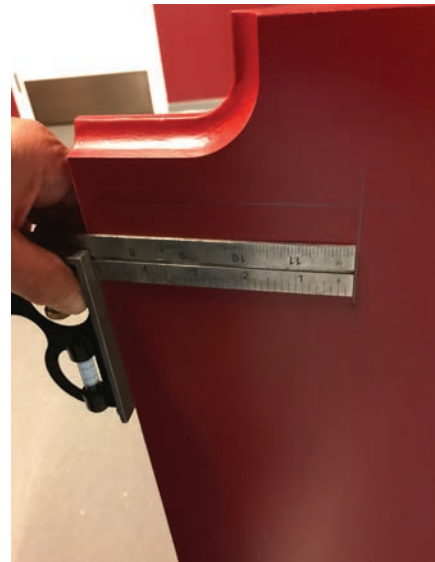
Figure 6. The author is shown marking the mounting location for the locks with a square.
