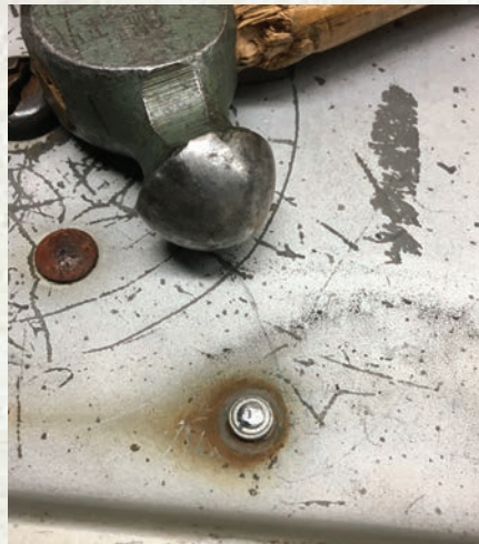
Figure 22. The attaching bolts for the latch bar slide were cut off and peened to prevent removal.
