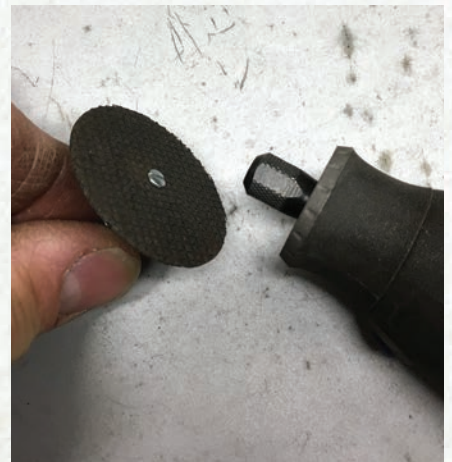
Figure 14. A Dremel tool with a large reinforced cut-off wheel is used to cut the slot between each of the set of holes drilled into the flat bar.
