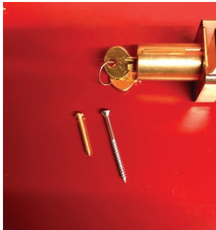
Figure 15. This image shows of the locks and the screws that came with it versus what the author actually used because of the shim.
