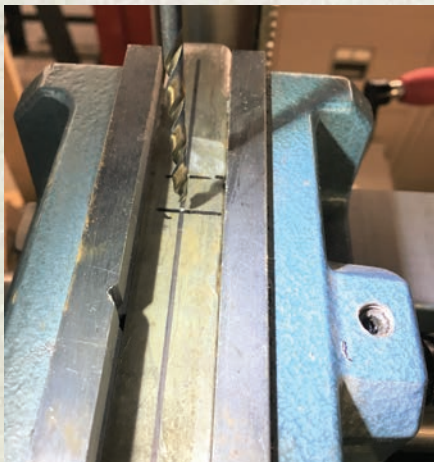
Figure 12. The flat steel has been marked for the slide locations and placed into the cross vise of the drill press in preparation for drilling.
