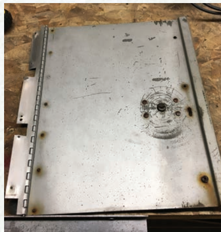
Figure 5. The main door is placed on the workbench in our shop. Note the damaged hinge.
