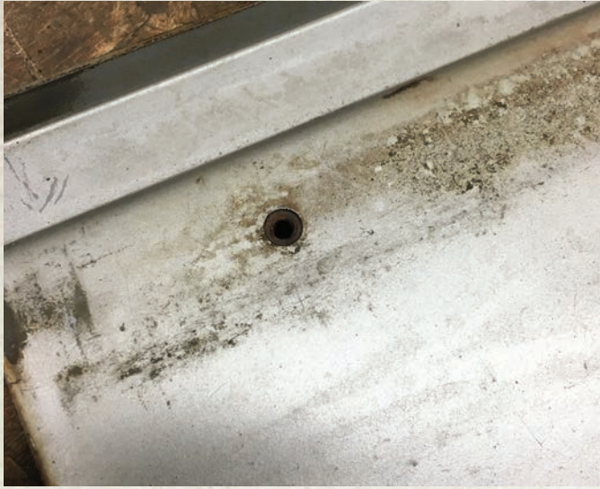
Figure 7. A hole from the old slide rivets is shown.
