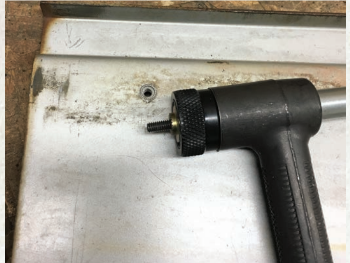
Figure 8. The same hole is shown with a newly installed nutsert (rivnut).
