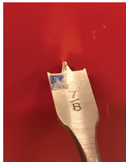
Figure 8. The author is drilling from the other side of the door using a pilot hole.
