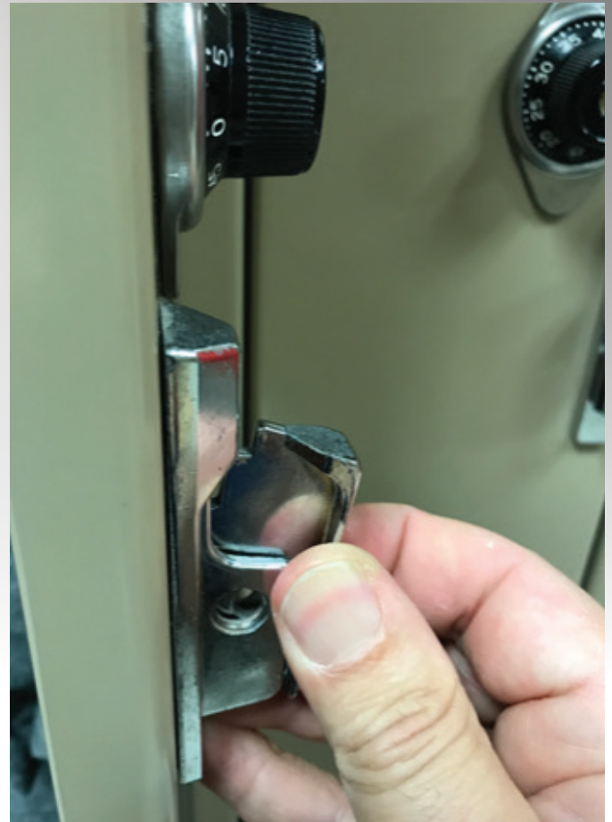
Figure 11. After the correct combination is dialed, the handle is pulled back to engage the mechanism in the door channel to push upward against the lift bolt and open the door.
