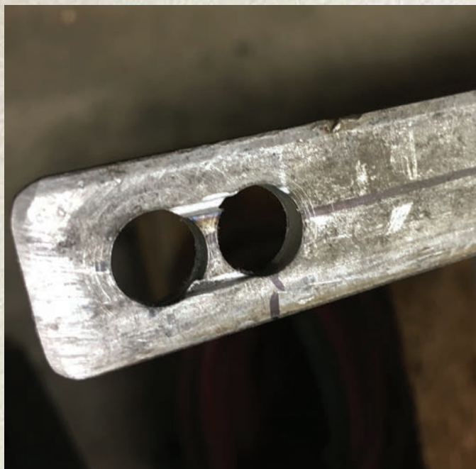
Figure 15. A close-up view of the flat bar slots as they are being cut is shown.
