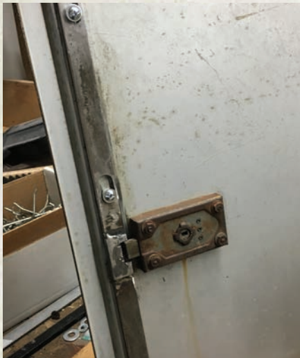
Figure 21. The assembled latch bar unit is shown.
