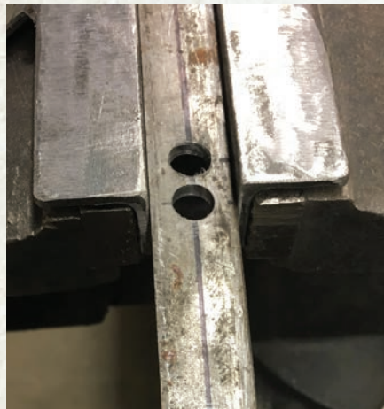
Figure 13. The holes for the top and bottom of each slot have been drilled into the flat bar, which is to become the latch bar.
