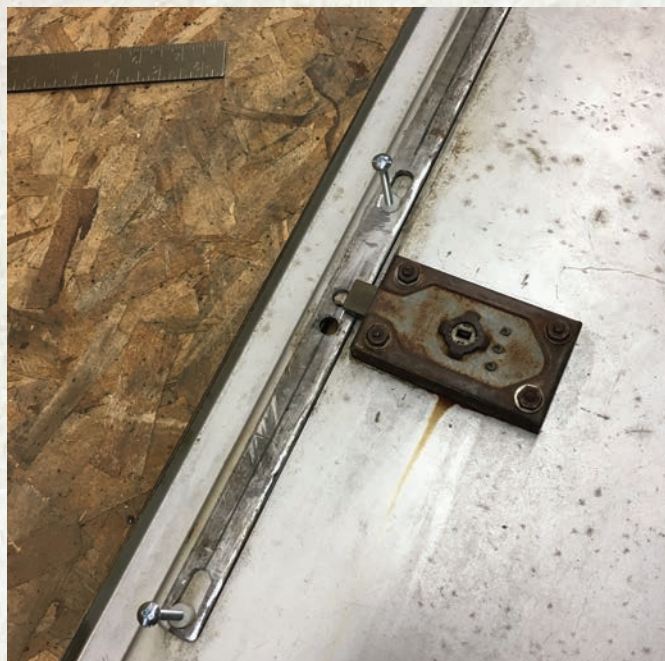
Figure 16. The latch bar was test fitted several times before it was determined that it would operate properly.
