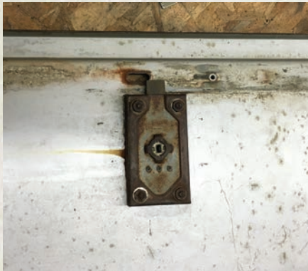
Figure 9. All of the nutserts are installed. An arrow had previously been marked to aid in remembering which way is up.
