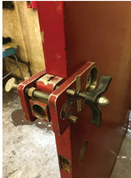
Figure 5. The author's A-1 boring jig is in place on the door.
