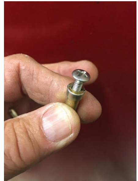
Figure 15. This screw holds on the inside handle.
