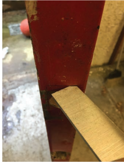
Figure 11. The metal skin of the door can be cut easily with a wood chisel without damaging the chisel.
