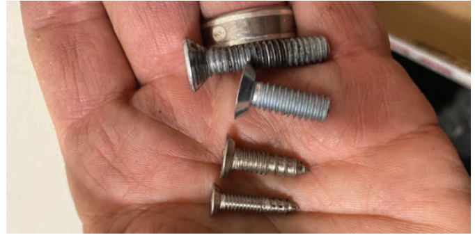
Figure 7. Several undercut screws are compared to a standard screw.
