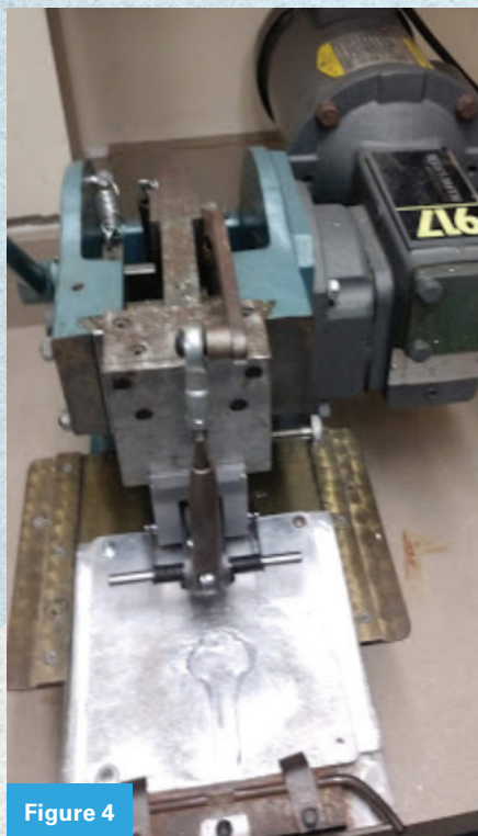
Figures 4 and 5. The Numberall #90 serializes keys with sequentially unique numbers.
