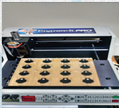
Figure 6. This ILCO engraver (left) saves hours on large master key projects. The stamping dies and tray are shown on the right.
