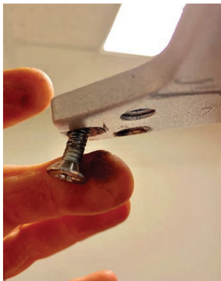
Figure 1. The screws were hanging out of the foot piece when the author arrived.
