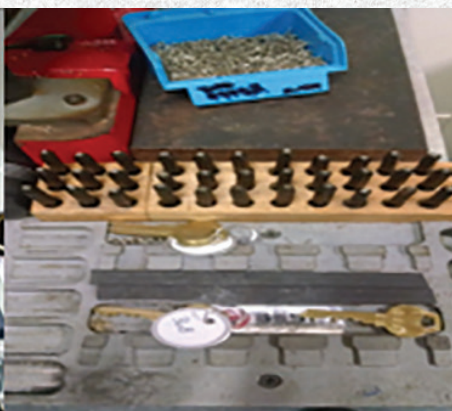
Figure 6. This ILCO engraver (left) saves hours on large master key projects. The stamping dies and tray are shown on the right.
