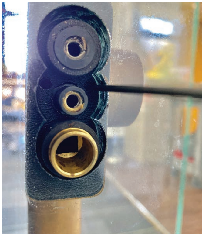
Figure 20. The wrench is inserted through an access hole to get to the set screw.
