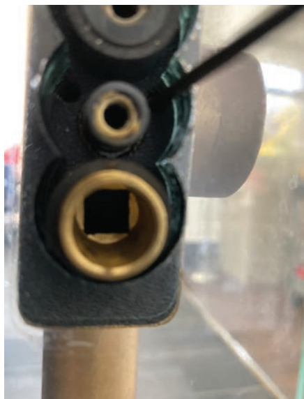
Figure 21. The square hole you see is the guide through which the actuator slides back and forth when locking and unlocking the bolt.
