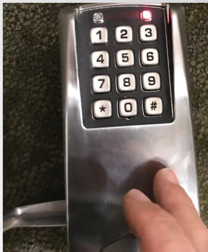
Figure 1. The PowerPlex lock uses a standard 10-digit keypad like you see on most phones.
