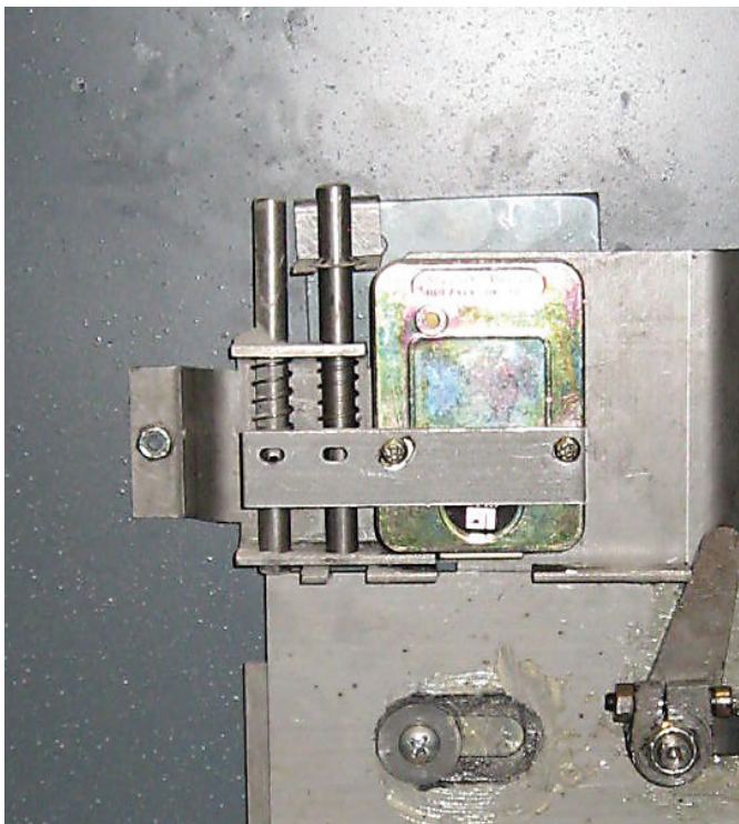
Figure 4. There are two relockers on this safe. The first, closest to the lock, is held back by the glass. The second one is held in place by a plate attached to the back cover.
