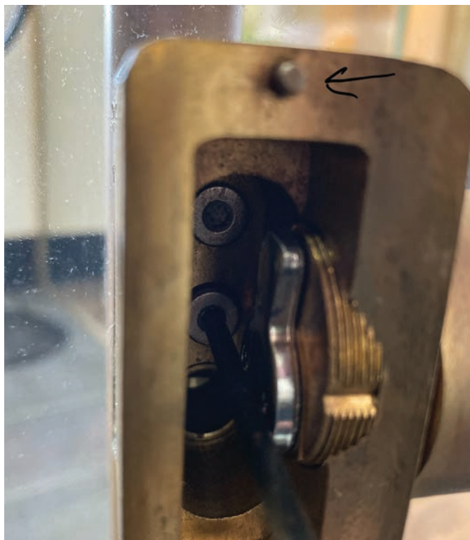
Figure 17. The arrow points to a pin that lines up with a hole in the handle.
