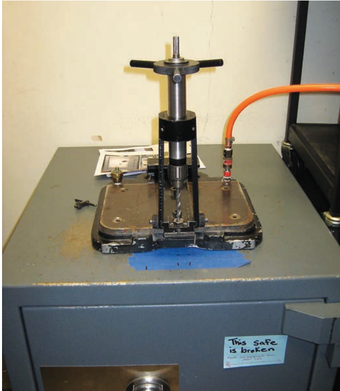
Figure 2. The author measured back and drilled his first hole to have a look around.
