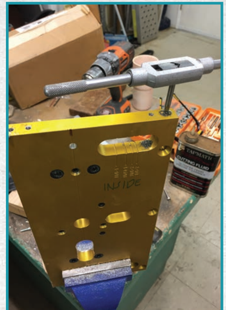
Figure 10. The top edge was drilled and tapped for socket head cap screws.
