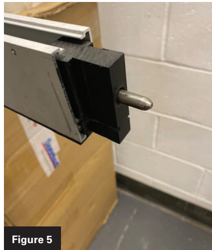
Figures 4 and 5. The rail can be seen in the unlocked and locked position.
