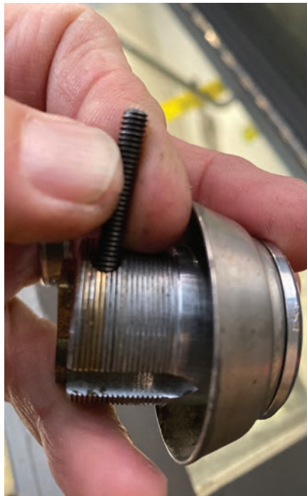
Figure 12. This photo shows how much deeper into the cylinder the screw fits.
