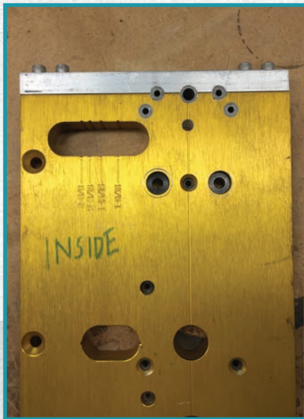
Figure 11. With the extension installed, the author added three hardened steel drill guide bushings.
