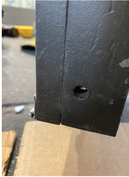
Figure 9. The access hole for the set screw can be seen.
