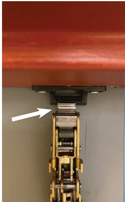
Figure 15. The trigger is on the wrong side of the strike, having slid under it.
