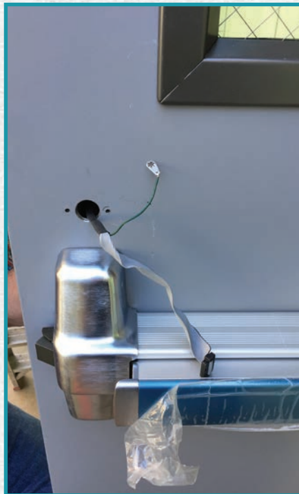
Figure 21. The battery pack and some of the electronics are mounted above the Von Duprin 99. Be sure to chase the threads in the inside base plate too.
