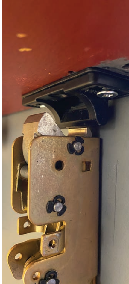
Figure 18. The trigger can't slide under the strike and jam anymore.
