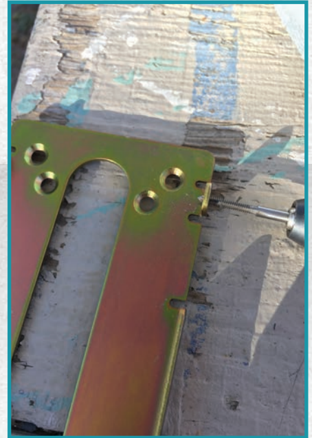
Figure 19. The first thing the author does with the base plates is to run a tap to chase threads in the holes (Alarm Lock plates or coats them after they are tapped). Sometimes the screws don't go in smoothly, and they are so small they break very easily.
