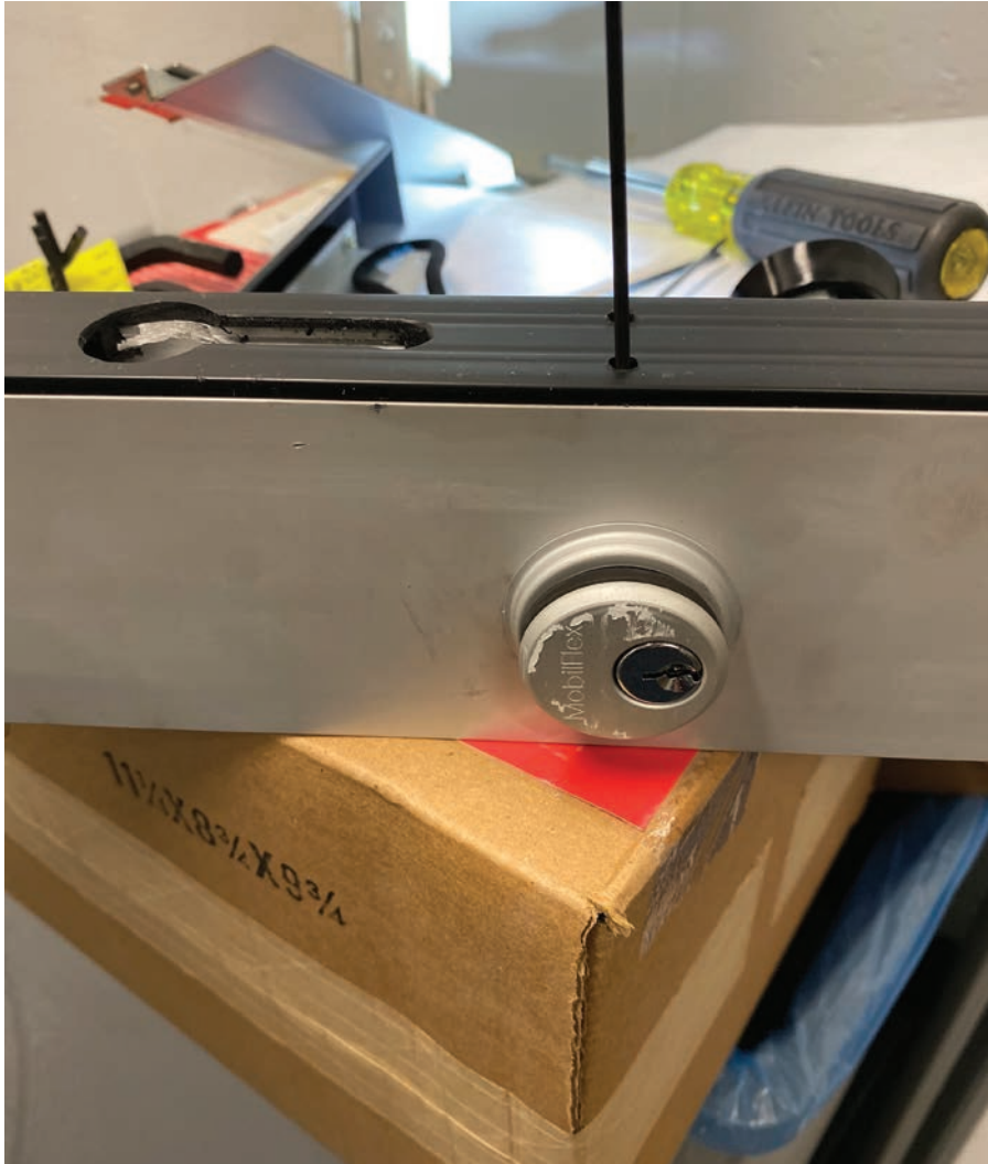
Figure 3. This photo shows the access holes for the set screws and the Allen wrench on the now-upside-down rail.
