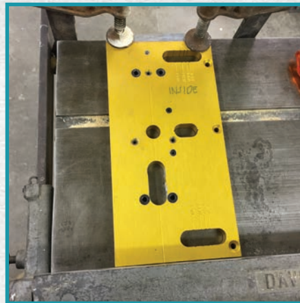
Figure 9. The customer has several locations, and the author expects to install Networkx locks at the balance of their facilities. Since there was a batch to install, the author modified a Major Mfg. Von Duprin 99 install jig to add the additional holes for the Networkx outside trim. He started by adding a section to the top of the inside plate.
