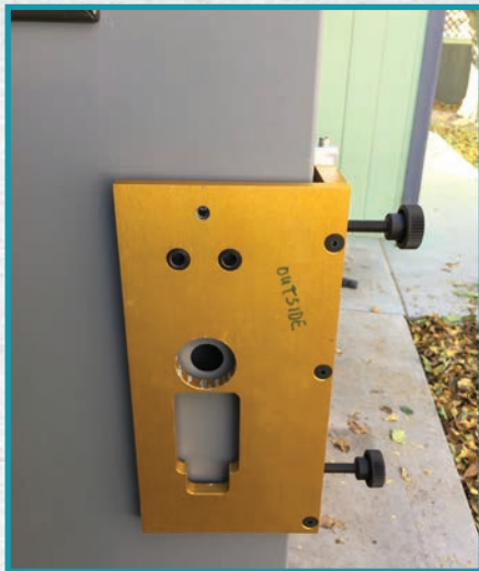
Figure 14. The modified Major Manufacturing drill guide is mounted to the door, centering the guide bushings over the center punch marks. The tool has two thumbscrews to adjust the location of the template on the door.
