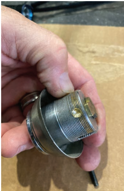
Figure 11. The author drilled a shallow hole into the cylinder where the set screw contacted it.
