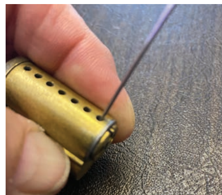
Figure 14. The author is holding the core and pushing a small punch through the bottom into the first chamber.
