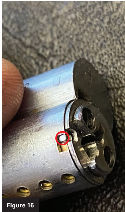
Figures 16 and 17. Figure 16 shows the back of a BEST Coremax or MX8 IC core with a key out, and Figure 17 shows a core with the key in.
