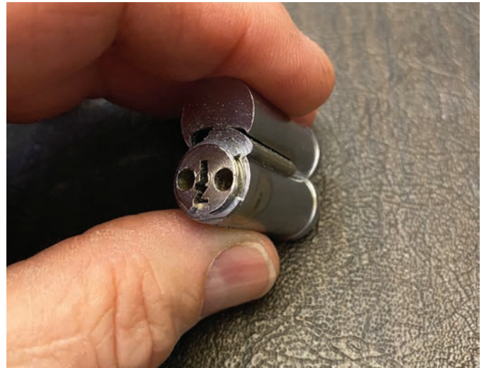
Figure 4. The core is with the control lug as it would be while the core is locked in the cylinder.
