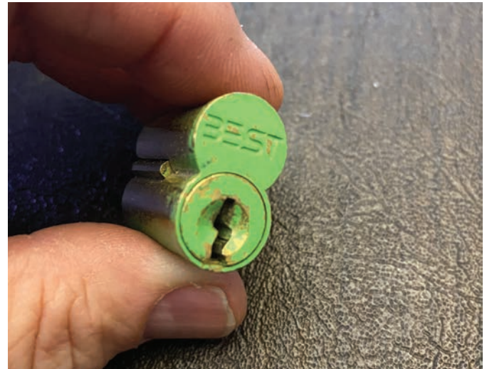
Figure 11. The construction core is painted green to mark it as such.
