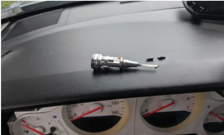
Figure 1. Shown is a broken actuator pin with its pieces retrieved.
