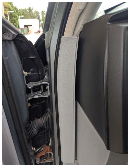
Figure 3. A trim piece in the doorjamb hides a screw for the lower dash cover and snaps in place.
