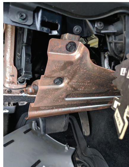
Figure 5. This sheet metal safety plate is held in place by four 10 mm screws and blocks most of your access under the dash.
