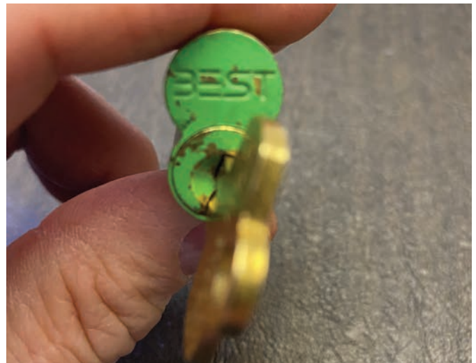
Figure 6. Note that the control key doesn't turn very far — maybe five degrees.
