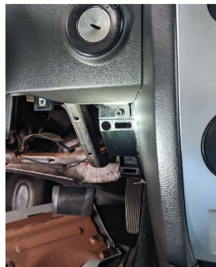
Figure 7. The third screw is shown, as is the beauty ring around the cylinder, which snaps in place. The top of the dash is held by clips as well.
