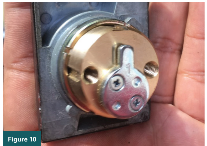
Figures 10 and 11. The new mortise cylinder is shown in the 8650 escutcheon pad.
