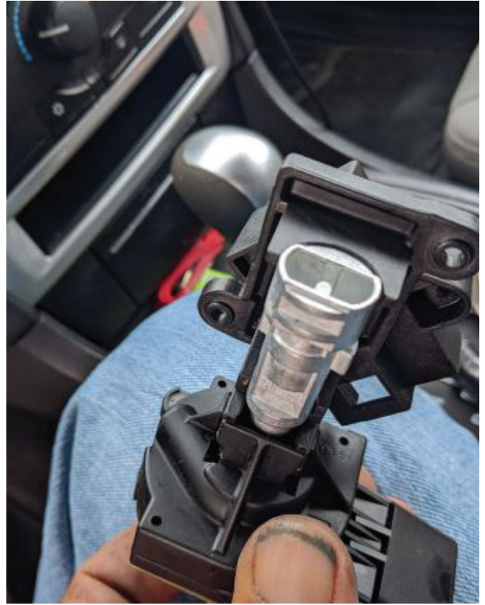
Figure 9. The actuator pin seats into the switch before mounting it back into the assembly. Remember not to seat it in 180 degrees out of sync.
