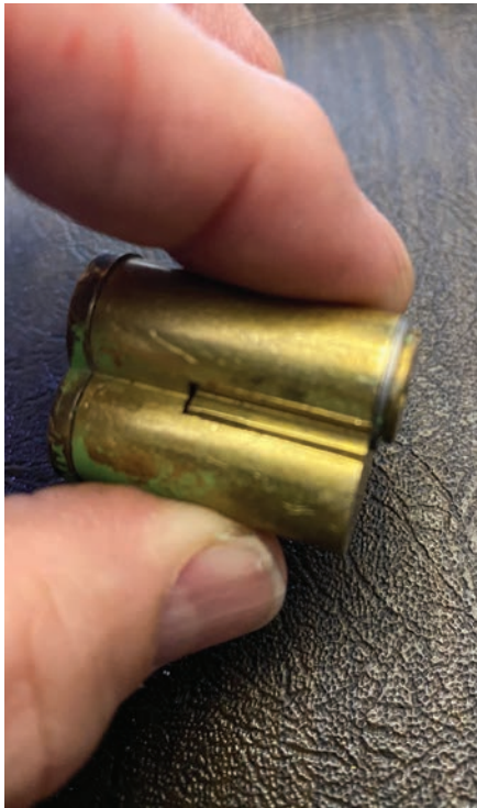
Figure 15. Once you get all the pins to drop, the control lug will slide in.
