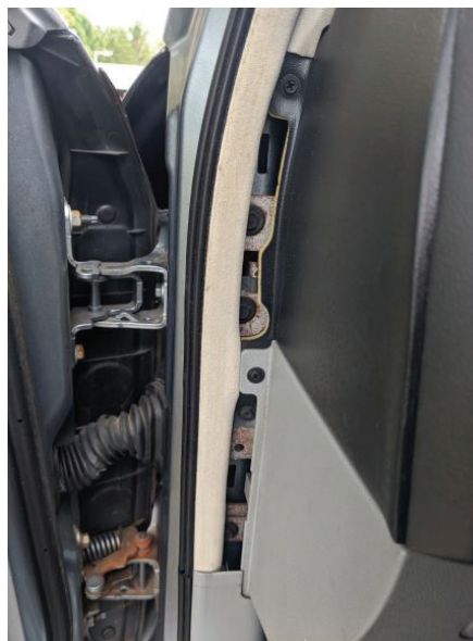
Figure 4. Here is that hidden screw for the lower dash cover.
