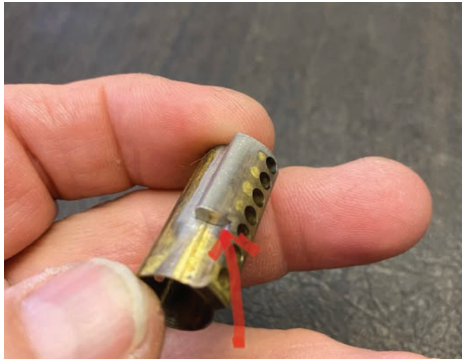
Figure 3. The arrow is pointing to the control lug on the control sleeve.
