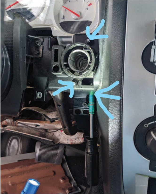
Figure 8. Three 8 mm screws hold the ignition assembly to the dash supports. The two facing you need to be removed, but the lower one you see the socket on only needs to be loosened to allow the assembly to slide out the back.
