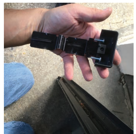
Figure 4. Slide the end cap out and remove it.
