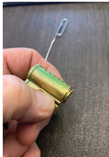
Figure 13. The author is pushing in the control lug with his finger.
