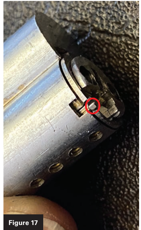
Figures 16 and 17. Figure 16 shows the back of a BEST Coremax or MX8 IC core with a key out, and Figure 17 shows a core with the key in.
