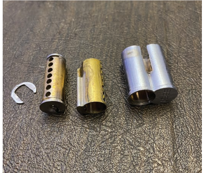
Figure 2. The author disassembled this BEST core.
