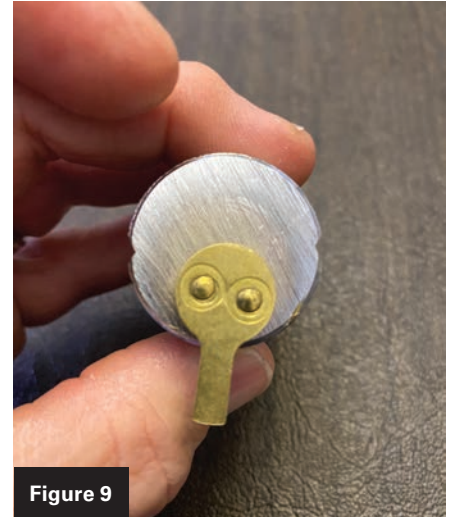
Figures 8 and 9. The back of the cylinder is shown with the cam properly timed ( Figure 8 ) and improperly timed ( Figure 9 ).
