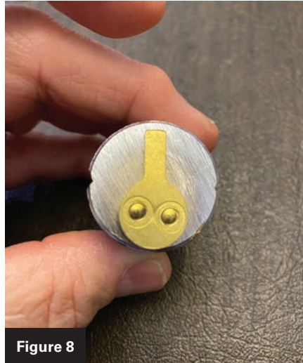
Figures 8 and 9. The back of the cylinder is shown with the cam properly timed ( Figure 8 ) and improperly timed ( Figure 9 ).
