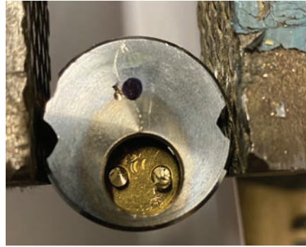
Figure 13. The cam is removed, and the author is tapping the back of the core with a punch to push it out.
