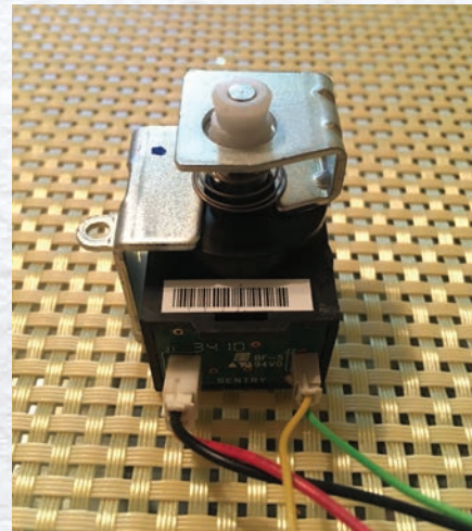
Figure 15. The white plastic tip of the solenoid is designed to bind when pressure is applied to the handle.
