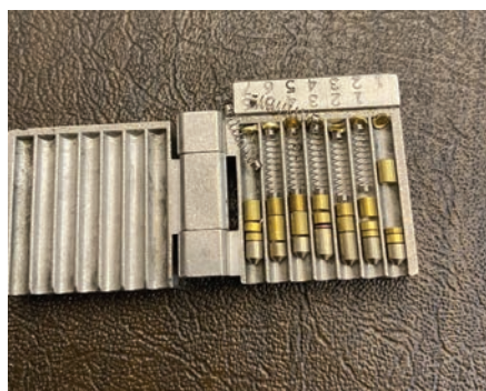
Figure 19. After you insert eject the pins, slide out the insert and carefully open it, you'll see something like this.
