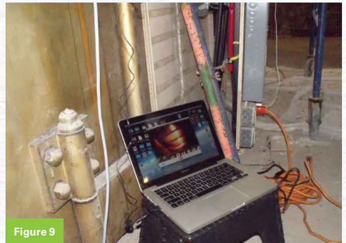
Figures 8 and 9. Finishing the hole with a 3/16" cobalt bit and using the borescope to view the wheels, David dialed and transferred the combination, but it would not open.
