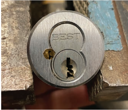
Figure 12. You can see the lug on the right of the hole.
