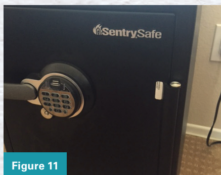
Figures 11 and 12. This is the newest model of Sentry Safe the author has encountered. Take note of the differences in keypad style, secondary lock, etc. The solenoid location is approximately 3 inches below the handle.
