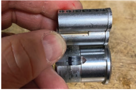
Figure 8. The black mark near the author's thumb in the groove shows where the set screw or yoke would normally bite into the cylinder once it's installed in the lock.
