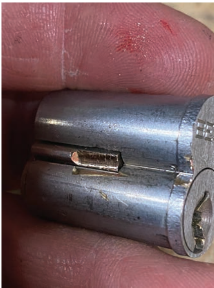
Figure 15. The lug is partially drilled away.
