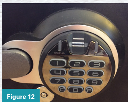
Figures 11 and 12. This is the newest model of Sentry Safe the author has encountered. Take note of the differences in keypad style, secondary lock, etc. The solenoid location is approximately 3 inches below the handle.
