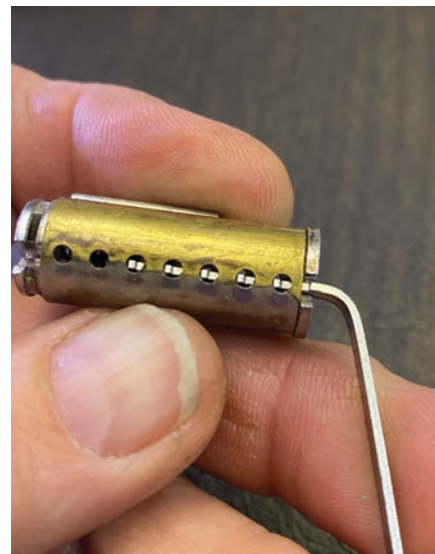
Figure 7. The projections are visible through the control sleeve of the core.
