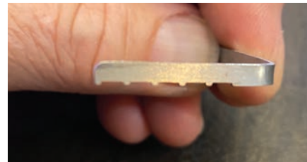
Figure 6. Gerry Finch designs this tension wrench.
