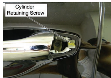
Figure 10. This image shows location of the retaining screw in the handle housing. No other trim needs to be removed.
