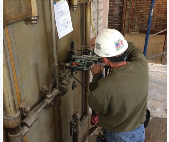
Figure 7. A 1/4" StrongArm drill bit proceeded fairly well.
