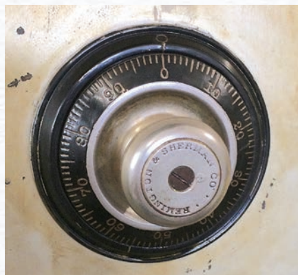
Figure 3. The author examined the dial. Notice the opening index has a circle-type marking and a mark on the dial ring referred to as a LOBC (locked on by combination) index.
