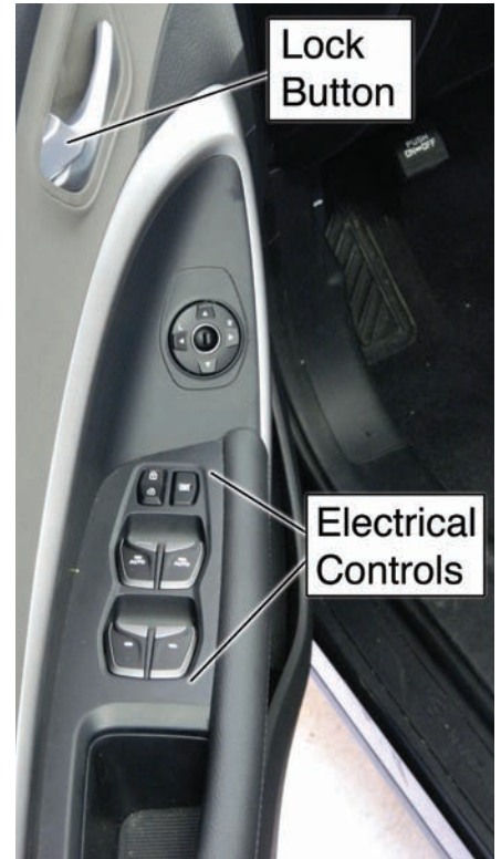
Figure 5. The central locking and window controls are mounted in the armrest of the driver's door.
