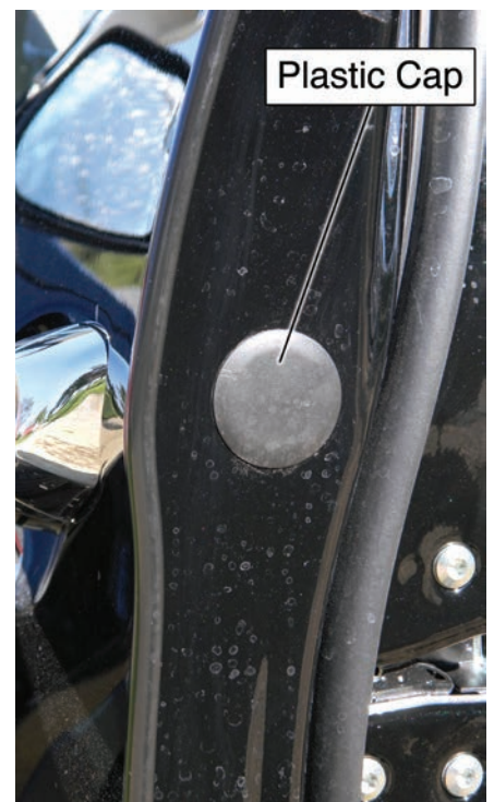
Figure 7. Remove the plastic cap to access the cylinder retaining screw.
