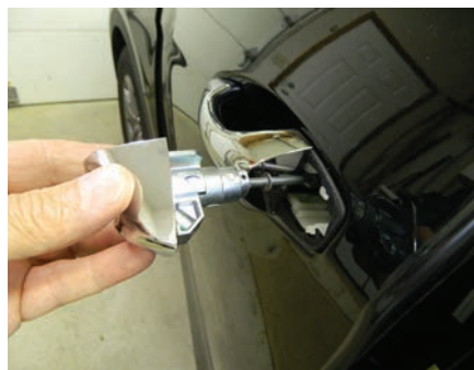
Figure 9. With the screw backed out, the cylinder can easily be removed.
