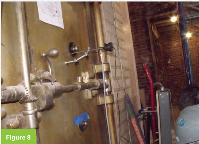
Figures 8 and 9. Finishing the hole with a 3/16" cobalt bit and using the borescope to view the wheels, David dialed and transferred the combination, but it would not open.
