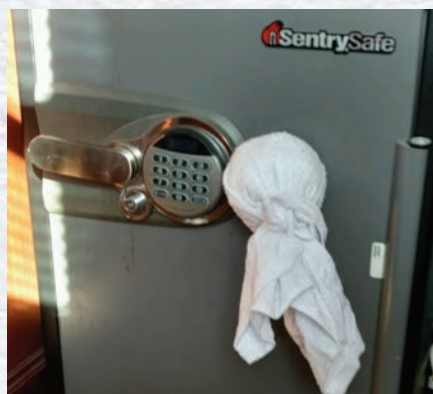
Figure 10. The magnet holds itself to the safe door directly over the solenoid, which is directly to the right of the number three button on the keypad.
