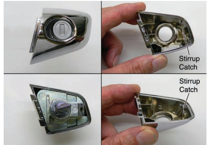
Figure 12. The stirrup catch at the rear of the plastic trim scalp is called out.
