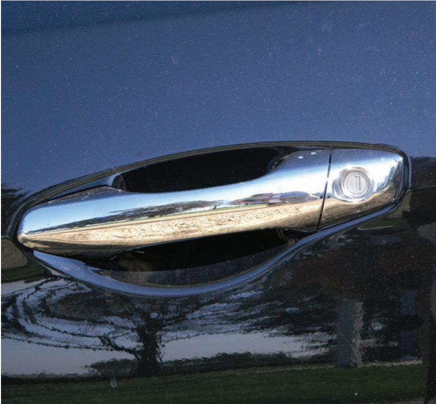
Figure 4. A single screw in the edge of the door retains this cylinder.
