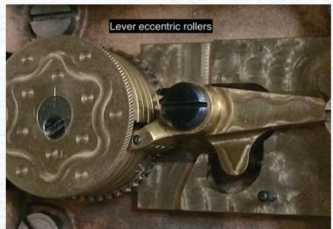
Figure 21. Note the lever's eccentric rollers.
