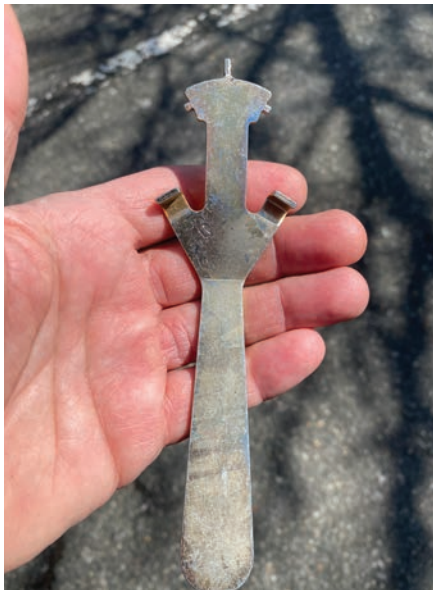
Figure 1. This image shows a BEST KD316 spanner wrench.
