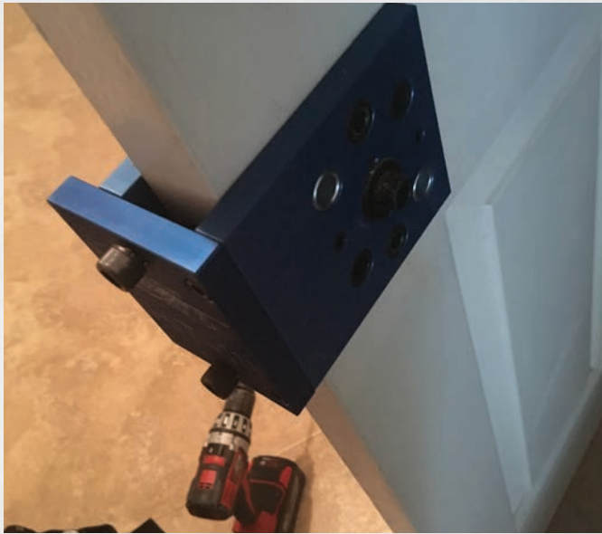
Figure 1. The tool works on 2 \frac{3}{8} " doors as long as you ensure that it is level to the rest of the door.
