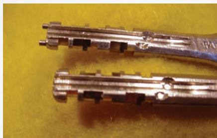
Figure 24. The Protec2 operating key (bottom) is compared to the LFIC control key (top).
