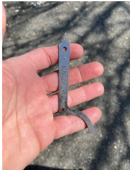
Figure 2. A Unican wrench will work, but it will not apply as much torque because of its shorter length.
