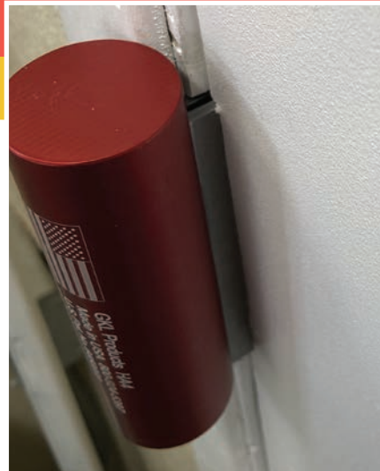
Figure 2. The larger GKL HA4 tool is closed on the end for more strength. The author finds it generally works on all commercial grade hinges.
