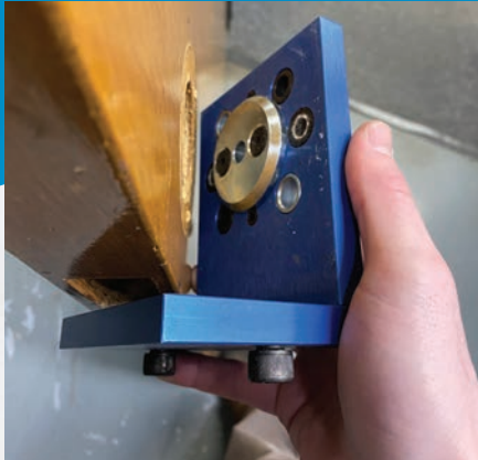
Figure 4. Place alignment washers into the crossbore and align the HIT-111 to the door.
