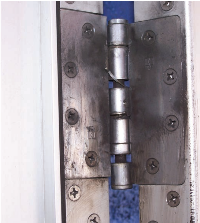
Figure 8. The other door hinge was far worse because the bottom bolt didn't hang below the door bottom. The wear was only to the entire threshold surface.
