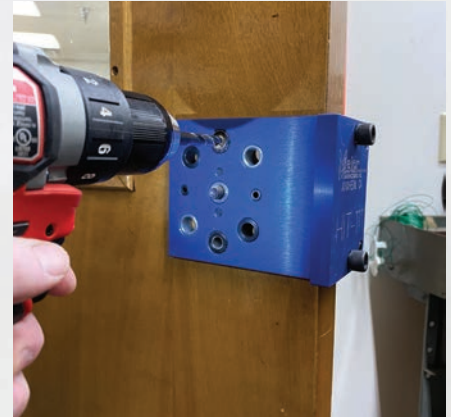
Figure 6. Select the bushing pair you will be drilling and begin by drilling from one side.
