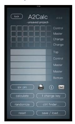
**Figure 1.** A2Calc allows the user to input the bittings of an A2 IC to find the control, master and change keys.
