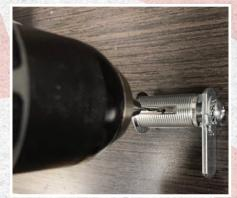
**Figure 20.** The author is drilling a small hole through the retainer in line with a pin chamber.
