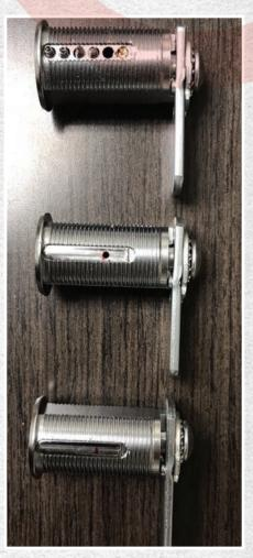
**Figure 29.** A side-by-side comparison shows a lock with the retainer removed, a lock with a hole drilled to remove the retainer and a lock reassembled.
