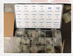
**Figure 19.** This service kit included tumbler chamber covers (identified in the kit as tumbler retainers), the various top and bottom pins, plug retainer pins and tumbler springs.
