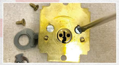
Figure 17. After removing the cam, the back plate has two staked screws that need to be removed.
