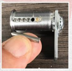
**Figure 25.** The tumbler retainer is a small, tented piece of flat metal designed to fit into a recessed slot on the top of the lock just over the tumblers.
