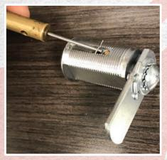
Figure 22. This pin ejector tool is normally used to eject pins from BEST interchangeable core locks.
