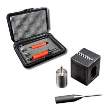
RAMON HAS RELEASED SEVERAL NEW PRODUCTS, including the Safe Deposit Killer Kit. The kit helps quickly drill S&G and Diebold safe deposit box locks when traditional methods can't be used due to a plastic or flimsy door. Simply insert the appropriate guide into the keyway and use a hole saw to drill out the face of the plug. The made-in-the-USA kit comes with three guides and two hole saws in a plastic carrying case.
