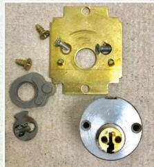
Figure 18. The lock cylinder is now separated.
