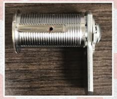
**Figure 21.** The drilled hole allows a narrow tool to be inserted to pry back the tumbler retainer and start peeling it back.
