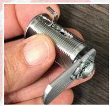
**Figure 23.** The retainer is peeled back most of the way back to expose the pin chambers.
