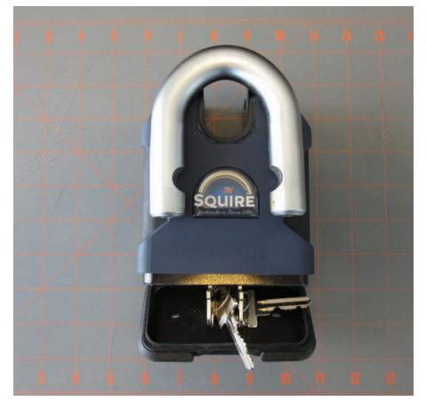
**Figure 8.** The 20 mm shackle has been removed and placed on the face of the lock to show how deeply it rests inside the body in the locked position.
