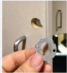
Figure 10. This cabinet is drilled to accept a cam lock.
