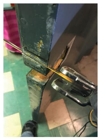
Figure 17. The cut was made with a reciprocating saw.
