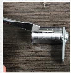
**Figure 27.** The author used a stubby flat screwdriver to flatten the retainer into the slot.
