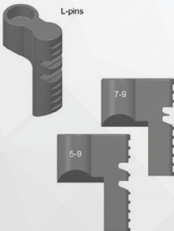
Figure 66. This illustration shows the design of the L-pin and its horizontal “notches.”
