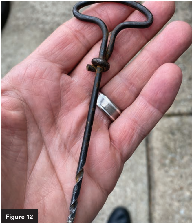
Figures 12 and 13. Gimlets were used to quickly drill pilot holes back when there were no power tools. Figure 13 provides a close-up view of the tip.
