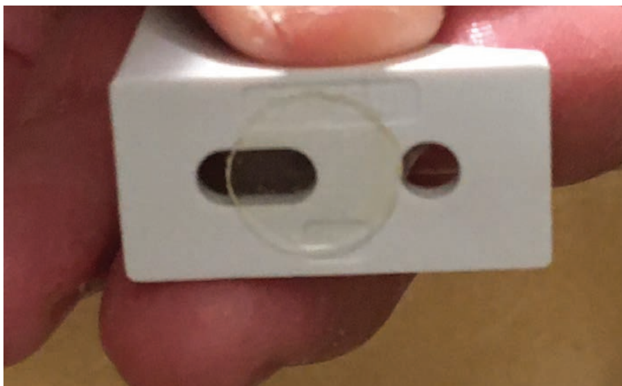
Figures 16 and 17. Using glue dots to temporarily mount the activator, latch and catch to the cabinet allows you to make any necessary adjustments before drilling mounting holes.
