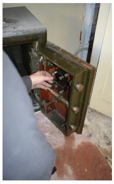
Figure 12. The replacement lock is being fitted.
