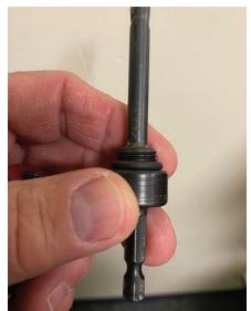
**Figure 7.** Just below the threads, you can see a rubber "O" ring.
