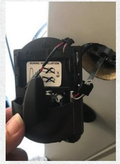
**Figure 16.** The wires have been guided through the rectangular hole.
