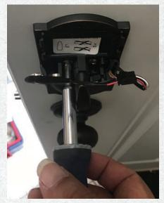
**Figure 19**. The screw on the left is being fully tightened.
