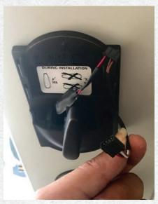
**Figure 17.** The inner assembly has been positioned over the tailpiece.
