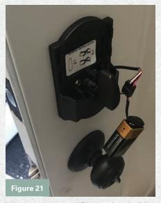
Figures 20 and 21. The author attached the included 9-volt battery (Figure 20) and left it hanging (Figure 21).
