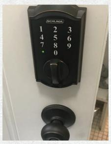
**Figure 24**. After you touch the "Schlage" button, the LED should light up.
