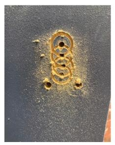
**Figure 5.** The series of shallow drilled holes are shown.
