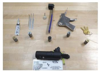
**Figure 2.** Shown from left to right are: the KW1 Lishi tool, rake and pick, bump key, snap gun and force keys.
