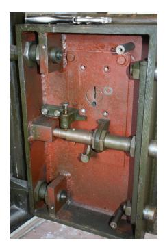
**Figure 9.** With the lock removed, you can see the drilled hole.
