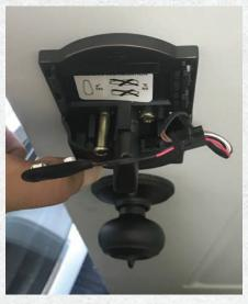
Figure 18. The wire connection has been made, and the two mounting screws are being attached.
