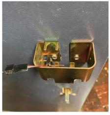
Figure 13. The battery bracket is screwed into the top two posts. The battery connector is visible to the left.
