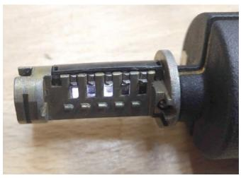
Figure 3. The LockTech decoder is fully inserted into a SmartKey cylinder, with sidebar and wafers removed.
