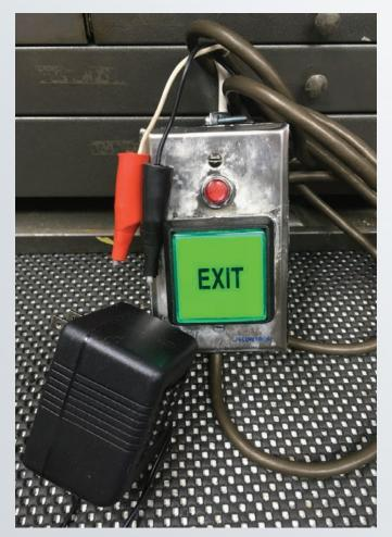
**Figure 24.** This power test kit is made from an old Securitron PB-2 and a Securitron plug-in 12-volt DC transformer.
