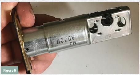
Figures 4 and 5. Twisting and rotating the tube of the latch bolt (*Figure 4*) lengthens the bolt, and after full rotation (*Figure 5*), the backset is now 2¾".
