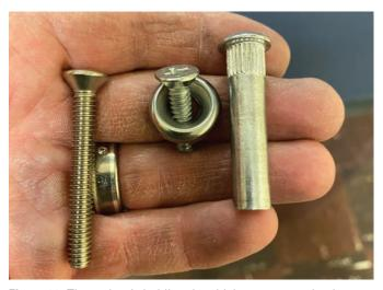
Figure 22. The author is holding the old, longer screw that he didn't use, the old finish washer plus a shorter  $\frac{1}{4}$ -20 screw and a door closer sexbolt.
