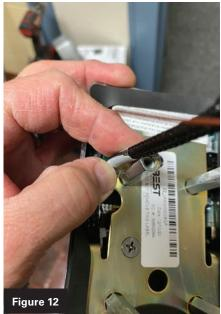
**Figures 11 and 12.** The wire is positioned it to pass through without pinching it when the screws were tightened.
