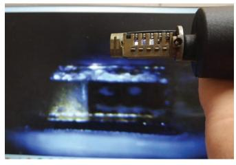
**Figure 1.** The LockTech decoder is fully inserted into a Kwikset SmartKey cylinder, and its corresponding view is on the computer screen behind it.
