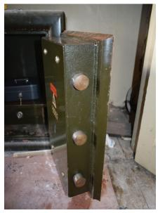
**Figure 6.** You can see the door thickness here.
