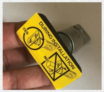
Figure 6. The bolt should not be extended when you start the lock installation.
