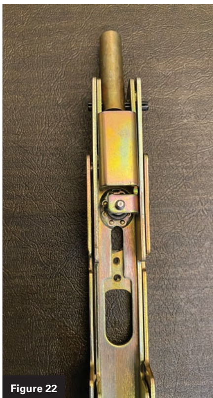
Figures 22 and 23. These images show what the carriage looks like when locked and unlocked.
