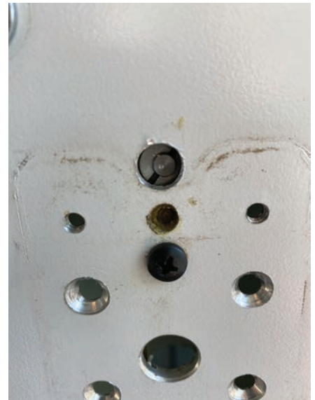
Figure 12. There should be two holes drilled above and below the head of the bar to access a pair of micro-adjustment screws.
