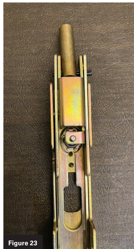
Figures 22 and 23. These images show what the carriage looks like when locked and unlocked.
