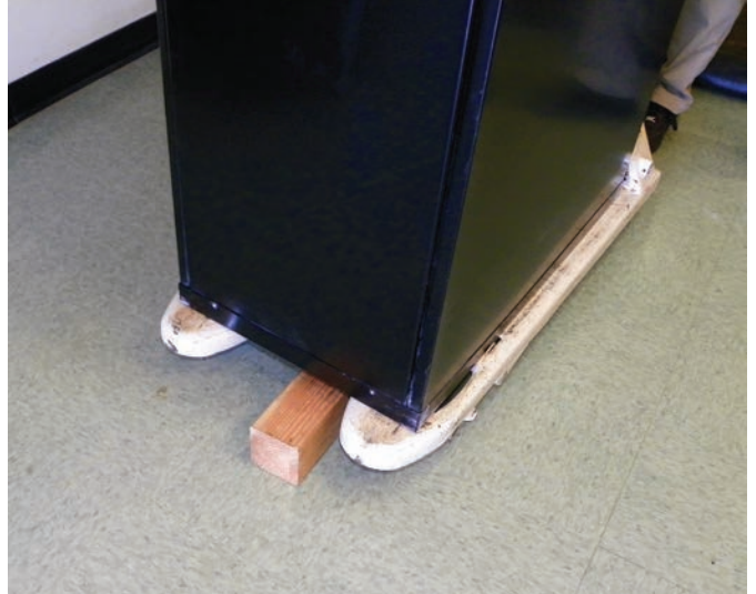
Figure 3. We see the pallet jack being driven over the block of wood. It is important to note that the block needs to be centered under the cabinet as much as possible. This allows for proper and safe balance, as we will demonstrate.
