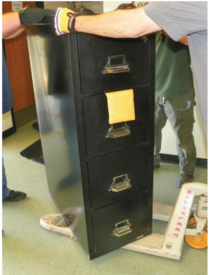
Figure 5. As one person continues to balance the cabinet, the other person will slowly swivel the cabinet the desired direction. Here, we see the cabinet at a 45-degree angle to its previous position.
