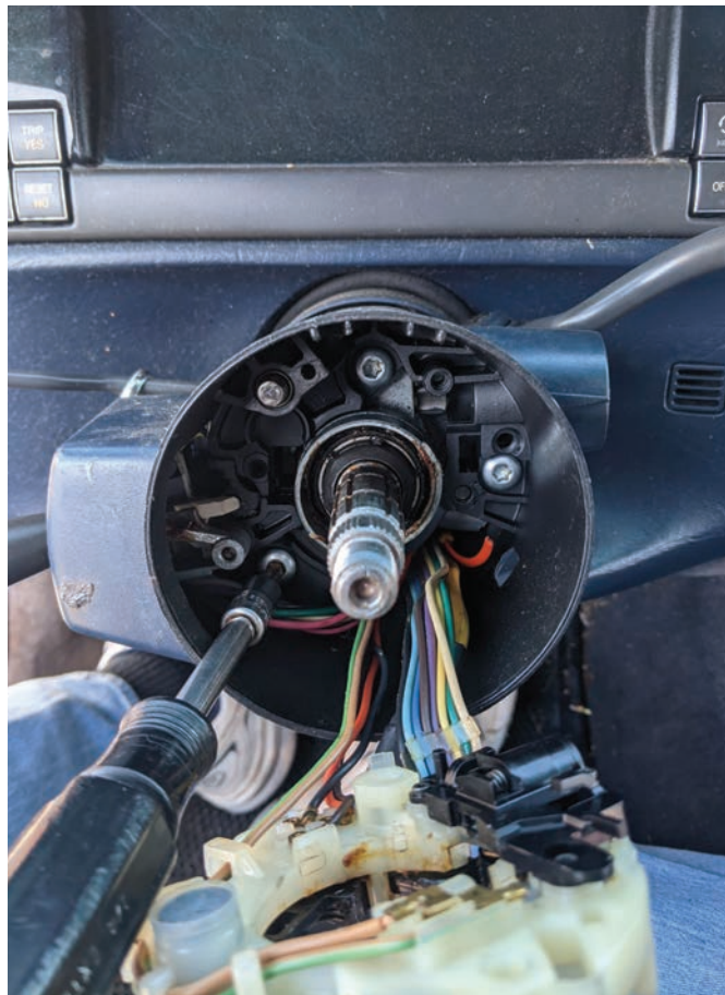
Figure 4. The first step of the journey involves removing these three screws and moving the cylinder out of the way.
