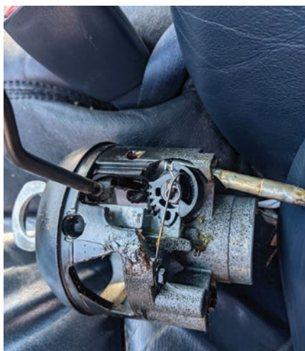
Figure 8. This side view of the workings shows where the gear moves the rack and retracts the steering wheel locking pin.
