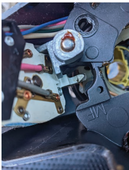
Figure 6. This shows the hole in the upper cover that the high/low beam actuator sits in during reassembly.
