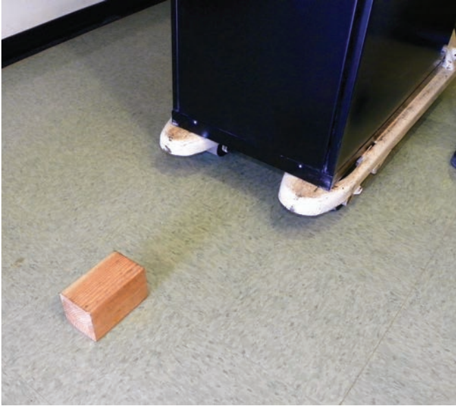
Figure 2. This photo shows the placement of the block on the floor directly in front of the pallet jack with the load.
