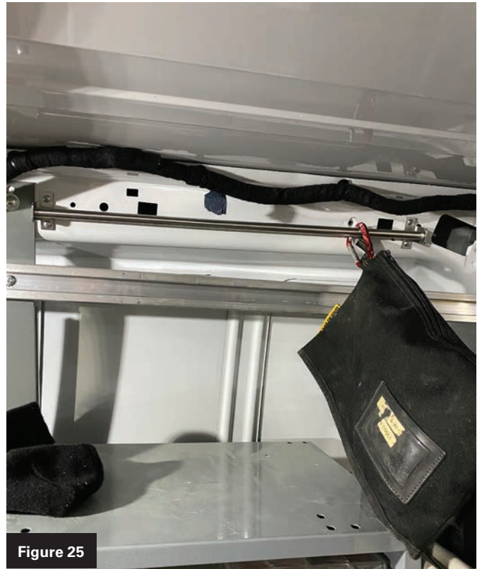
Figures 25 and 26. This round steel rod from IKEA costs $4. The author screwed it into a channel in his truck (Figure 26).
