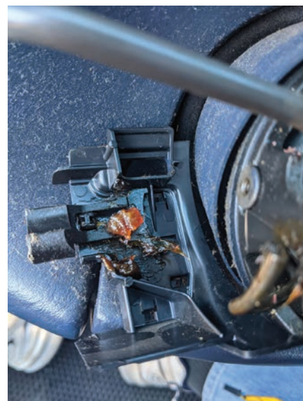
Figure 5. The high/low beam actuator rides around a pin in the back cover and stays in place by virtue of the heavy grease that keeps it lubricated.
