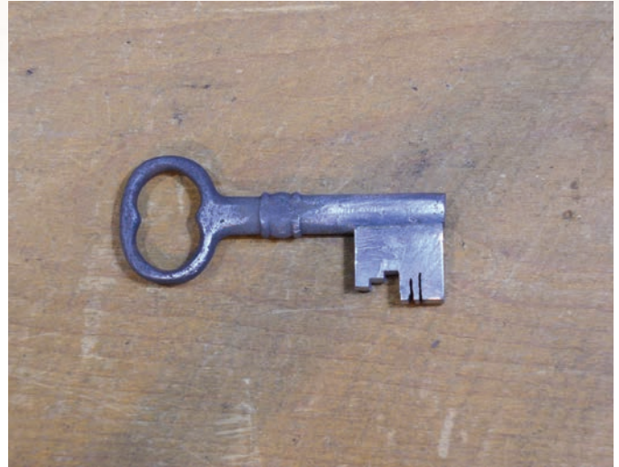
Figure 10. The old bit has been sawed off, and the stem has been filed.
