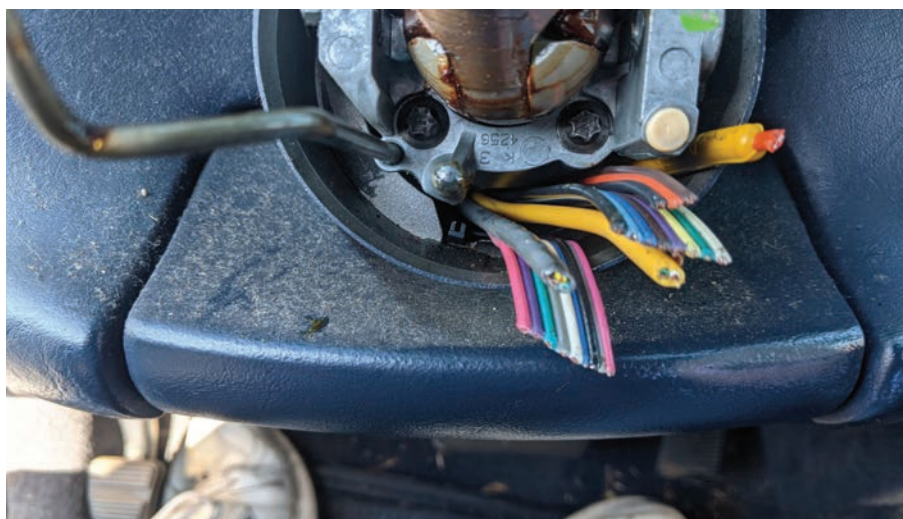
Figure 12. You can see two out of the four screws that hold the lower housing tight to the tube. Note: In a normal setting, you would not cut all of these wires.
