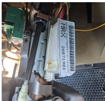
Figure 13. The ignition switch is mounted down the column past the column-mounting bracket.
