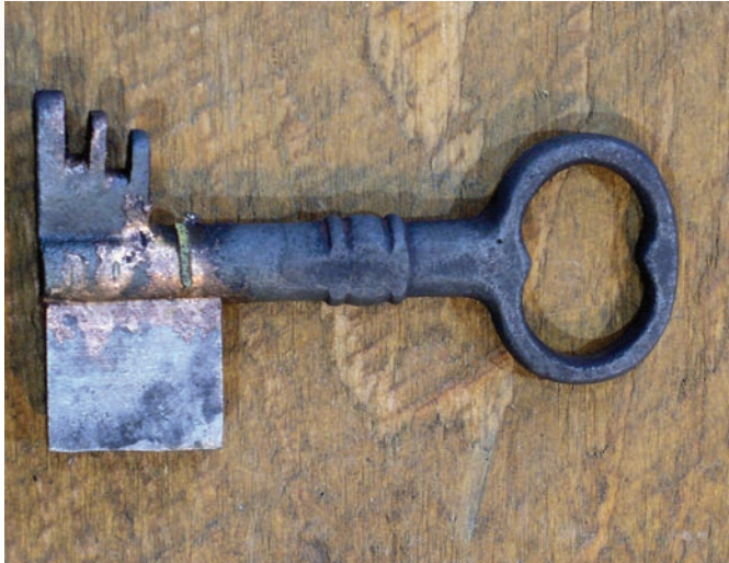
Figure 9. The old key has had steel for a new bit brazed on opposite the old bit.
