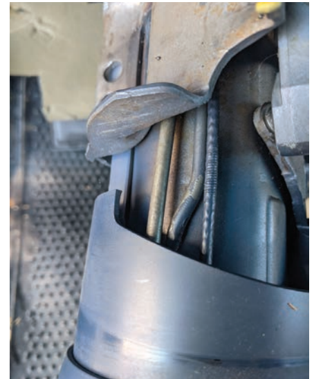
Figure 15. The linkages for the ignition switch and dimmer switch are running parallel down the left side of the column. You can also see the wire harness for the accessories added to the turn signal stick.
