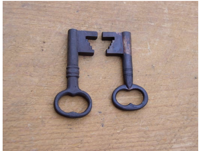
Figure 12. The second key had a broken bow that had been unevenly reattached with poor gas welds, so a new bow was made.
