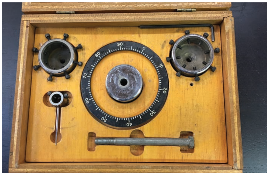
Figure 10. The SDR Tool Set from Dib's Safe and Lock can be used to dial open a safe.
