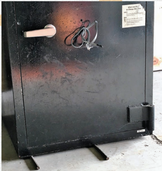
Figure 5. As the roller closest to the leading edge reaches the center of the safe and the roller that was in the center reaches the trailing edge, stop forward progress.
