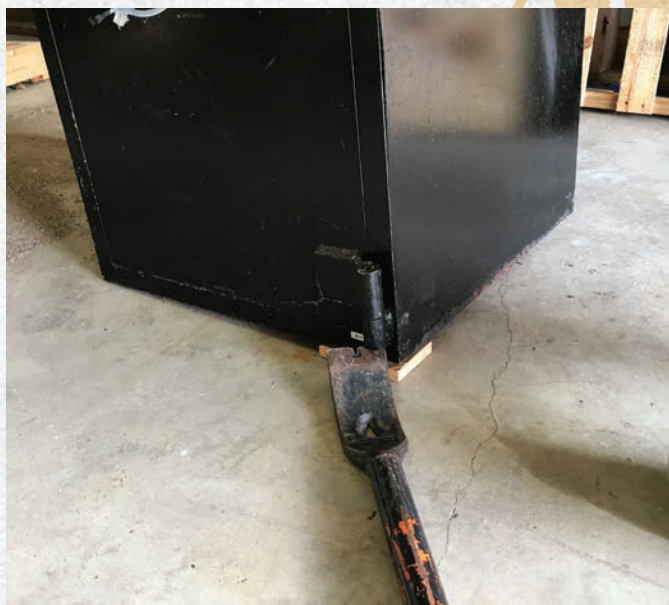
Figure 2. The first step is to lift the leading edge high enough to place a wedge or short block of wood under the safe to lean it toward the trailing edge.
