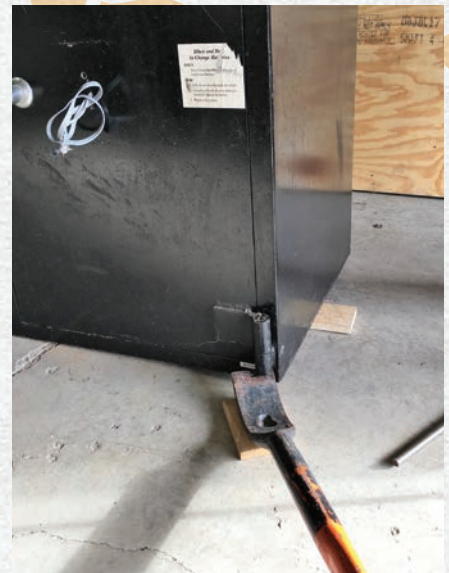
Figure 10. Use the wedge or block of wood to lift the safe high enough to remove the remaining roller. Then remove the wedge or block.
