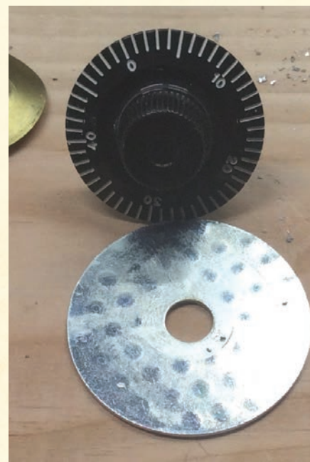
Figure 4. Not unlike some high-security safe locks available, there seems to be an additional piece of steel behind the dial to discourage drilling.
