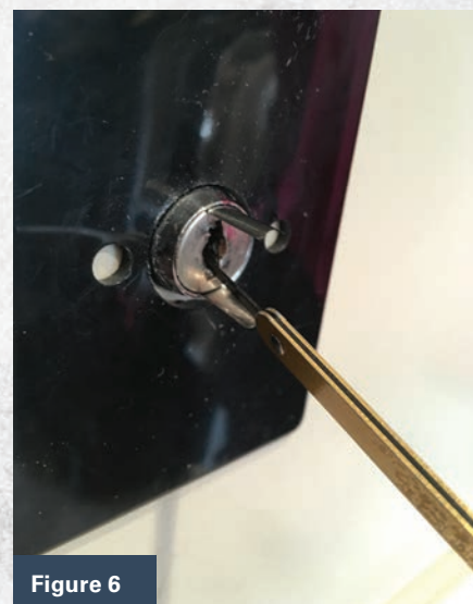
Figures 5 and 6. There is enough of a gap between the plug and the shell to insert curved shims.
