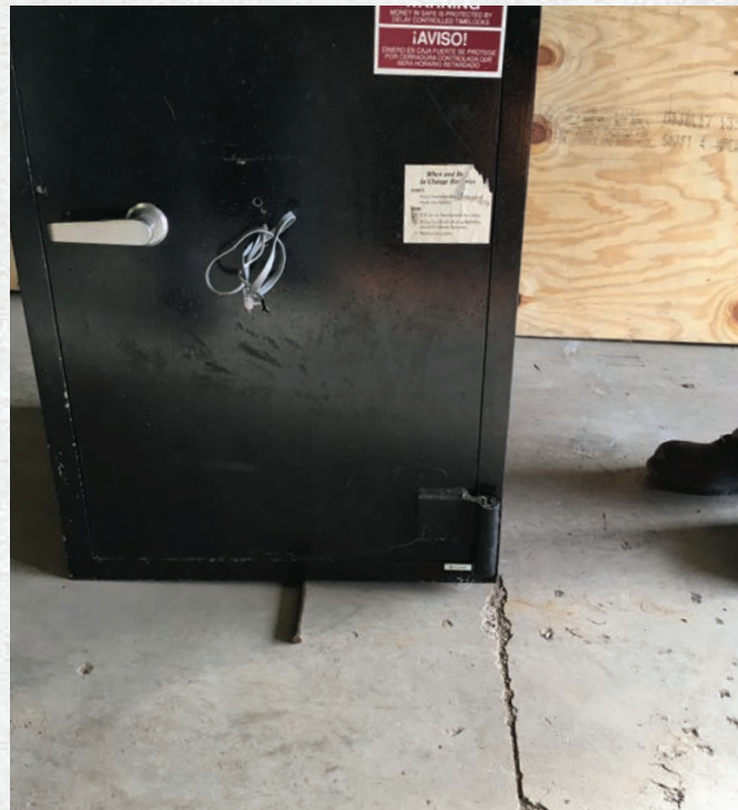
Figure 6. Remove the roller from the trailing edge and rock the safe back, exposing the leading edge.
