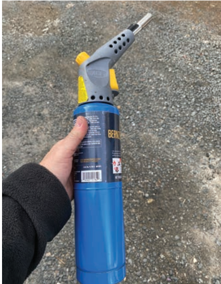
Figure 6. The author tried using this torch to melt thread locker.
