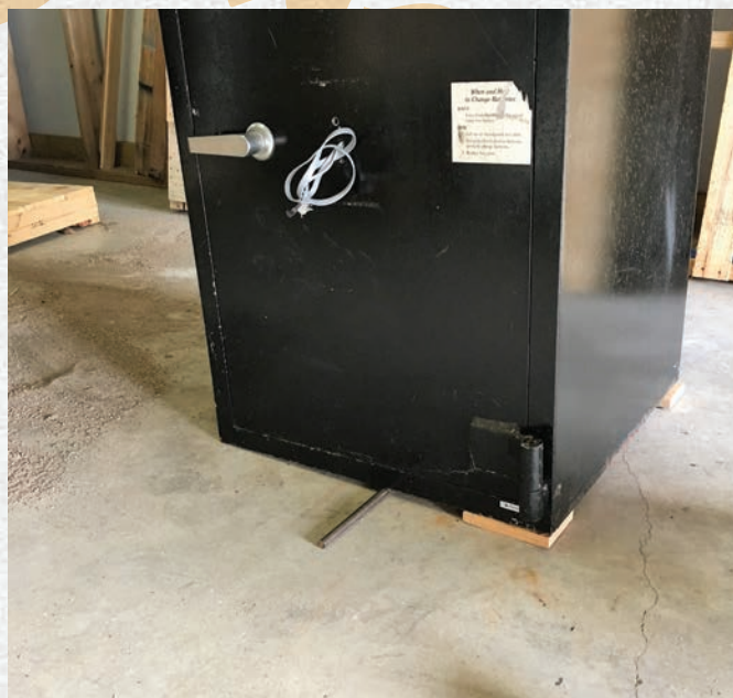
Figure 3. Allow the roller to stick out past both sides and slide it as far away from the leading edge as possible.
