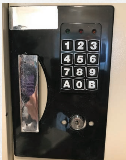
Figure 1. This style of AMSEC wall safe has thin walls and simple electronics.
