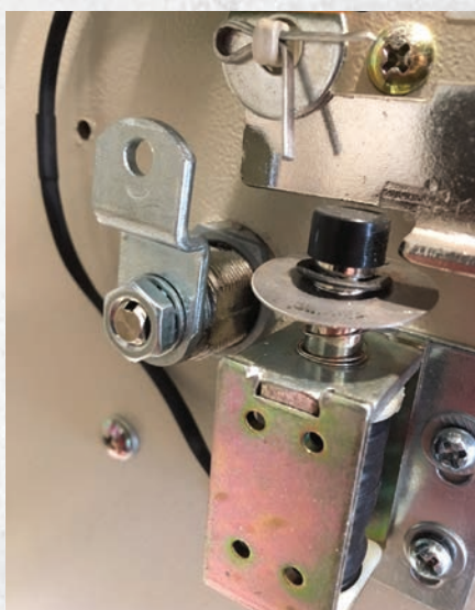
Figure 2. The cam is in the home position.
