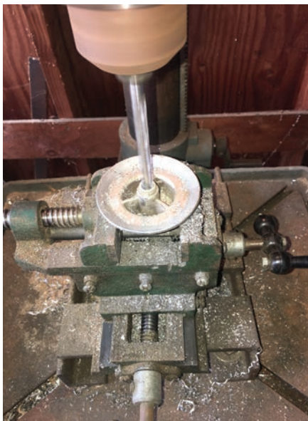
Figure 4. The author is drilling a \frac{23}{64} " hole in the dial.
