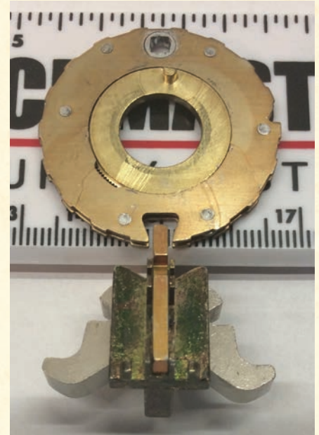
Figure 7. If you need to try dialing high or low to open a stubborn lock, use half-number increments. Sometimes these slight adjustments make the difference between success and failure.
