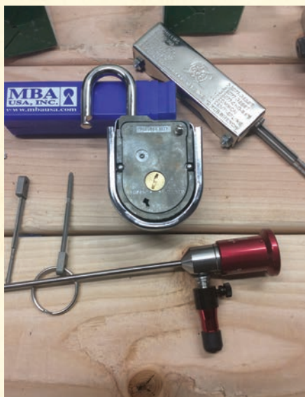
Figure 2. Scoping through the CKH between change key cams adjustments ensured they were aligned, but the author could not see where the inner arm teeth made contact with the inner hub on anything besides the closest wheel.
