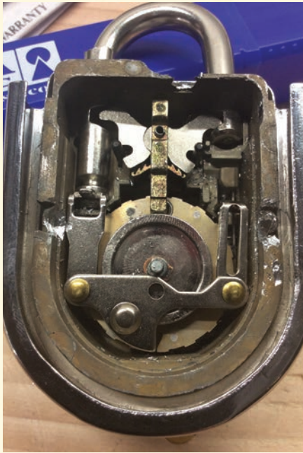
Figure 5. The lock's internals are generally of a straight-tailpiece design. It's all cantilevered and fancy but still a direct-entry lock.
