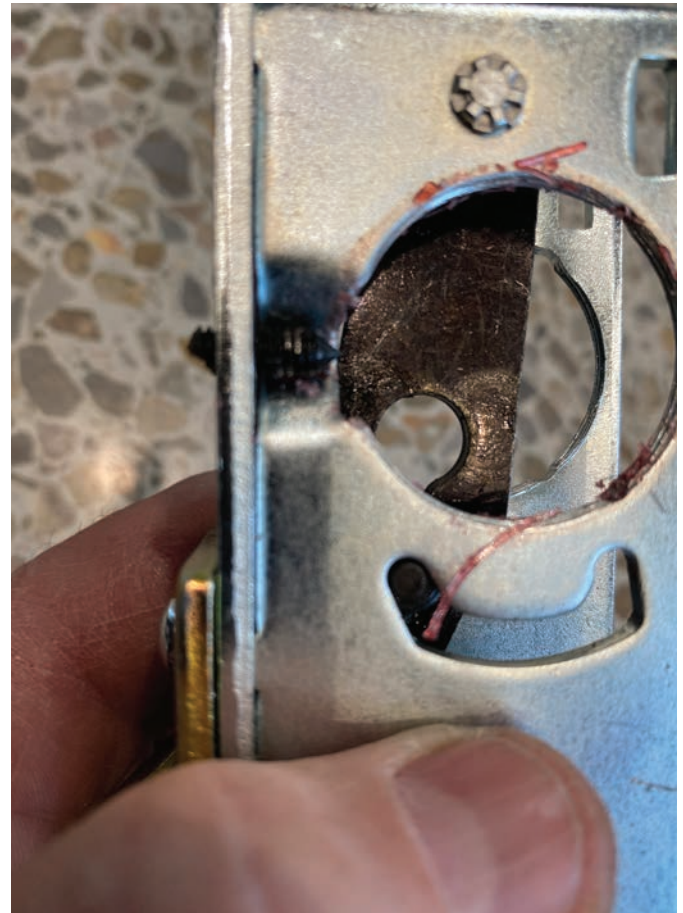
Figure 5. Whoever installed the cylinder deemed it necessary to load it all up with thread locker.
