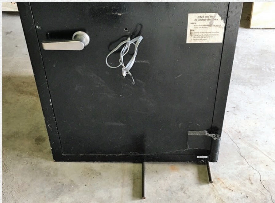
Figure 4. The author has inserted a second roller about an inch or two from the leading edge.
