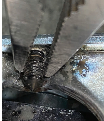
Figure 7. The author alternated heating with sticking the lock into a nearby pile of snow to cool it and then turning the set screw with pliers.
