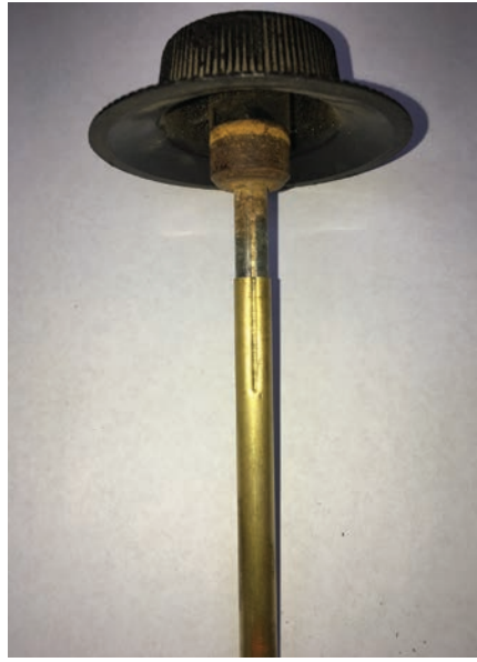
Figure 2. The brass tube is formed on the Major steel spindle.
