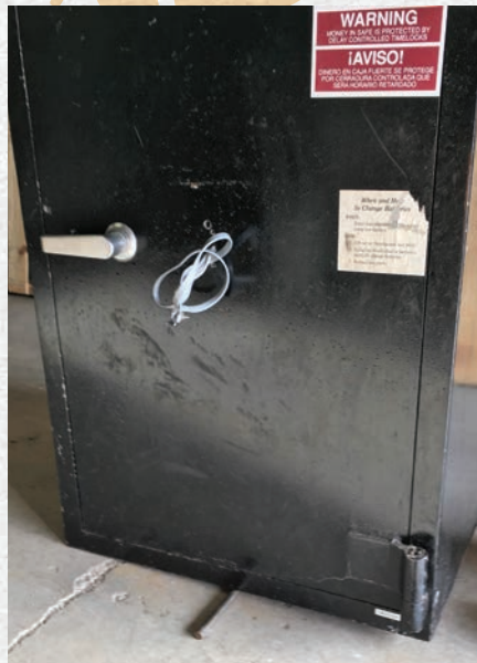
Figure 9. The safe has been rocked onto its leading edge so the author can remove the roller from the trailing edge.
