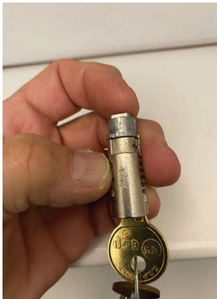
Figure 16. Here, you can see the small cast part fitted onto the plug.
