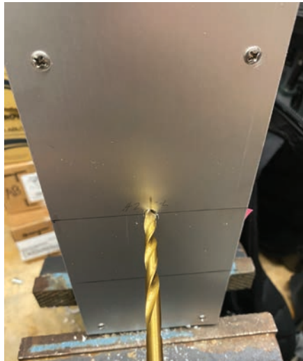
Figure 7. The author is drilling the pilot hole for the 2½" hole.
