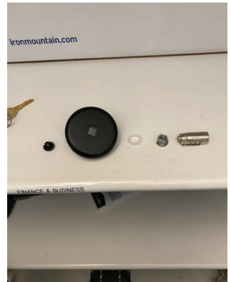
Figure 11. The screw that held everything together had loosened and fallen out.
