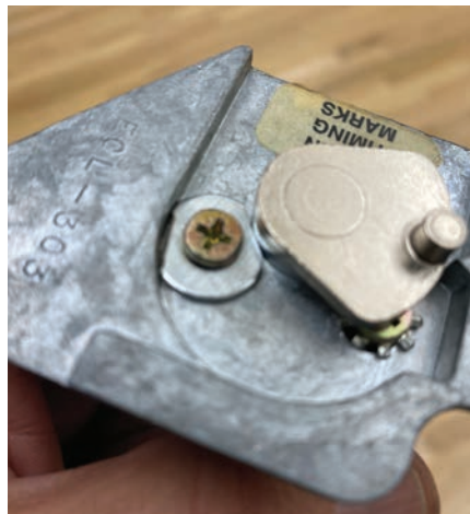
Figure 24. This is the part in a Detox ECL-230 exit alarm that holds the rim cylinder used to lock and unlock the device from the inside.
