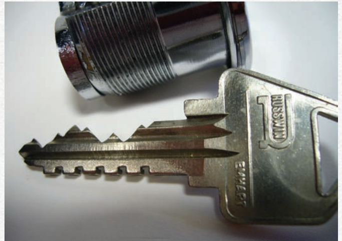
Figure 2. Notice the unique bow shape and the undercut grooves on the Emhart key, pictured with a mortise cylinder.
