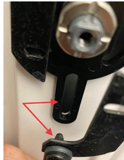
Figure 17. The arrows point to the tip of the screw and the slot it slides up and down in when the plug is turned.
