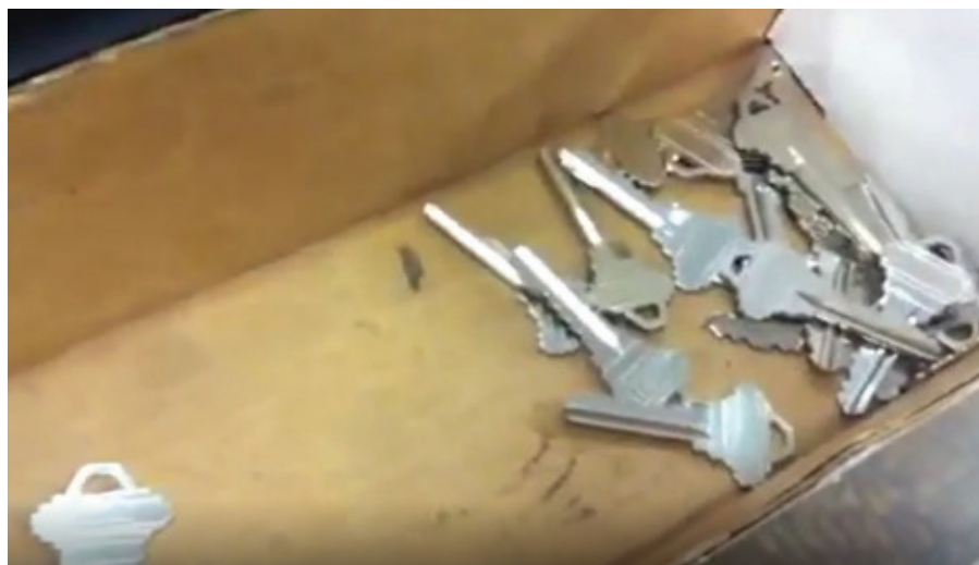
Figure 1. Unfortunately, shoeboxing uses more master pins than necessary, and it relies on luck to avoid key interchange.
