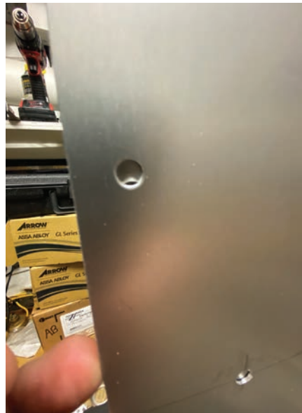
Figure 6. Notice that the holes on the plates don't line up.
