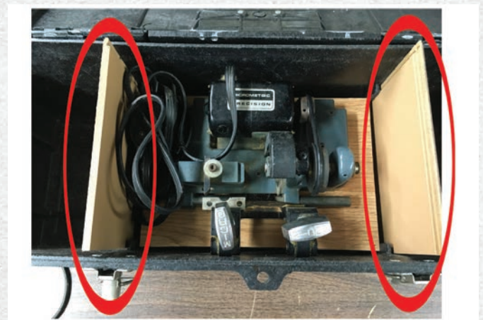
Figure 21. A couple of side panels made from some of the left-over laminate flooring help isolate the key blanks away from the key machine.
