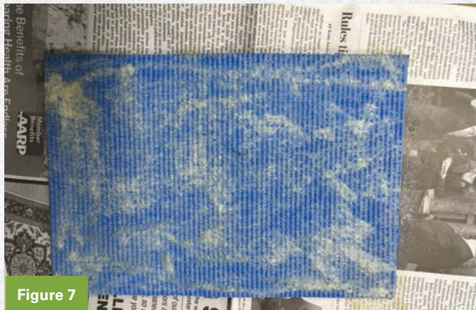
Figures 7 and 8. The adhesive was applied to both the OSB and the mat.
