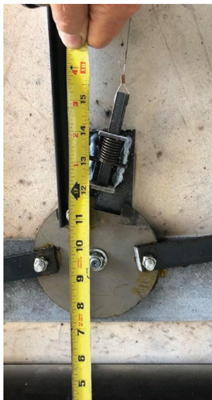
Figure 8. This shows the bottom external relocker. The attached cable goes under lock body and ricochets off a top brace before going to the bottom of door. All this routing is done to avoid the cables being tangled in the handle cam, I would guess.
