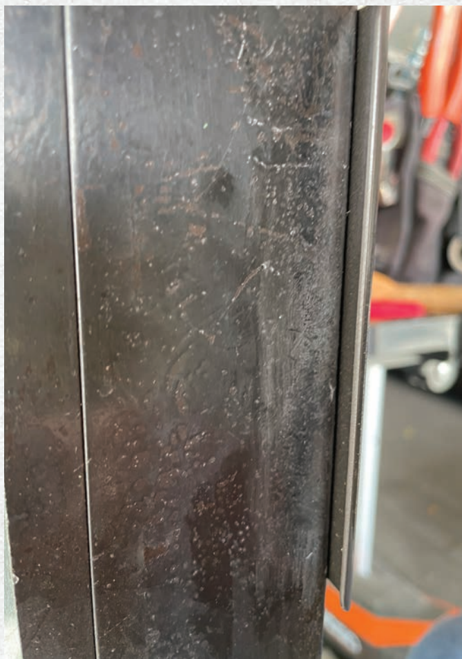
Figure 21. Here is the back, or underside, of the strike. The router creates a nice finished edge for the strike to sit against.
