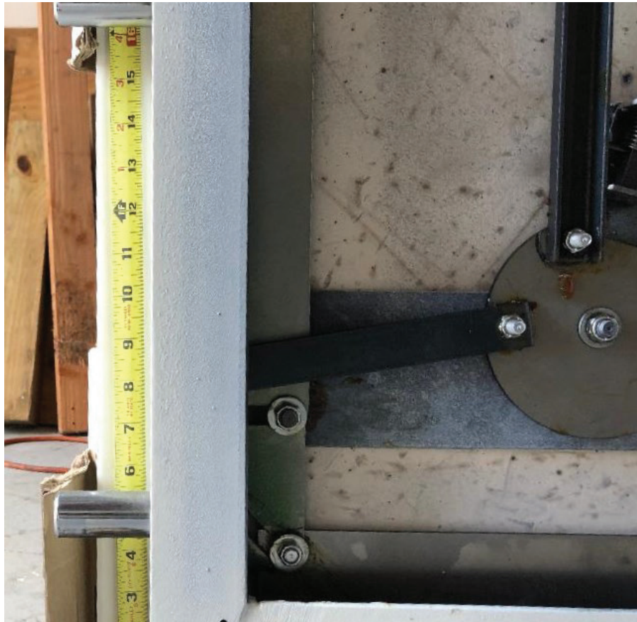
Figure 12. In this photo, you can see the bottom of the door and the distance to the bolts. You could use this measurement to punch the bolts back.
