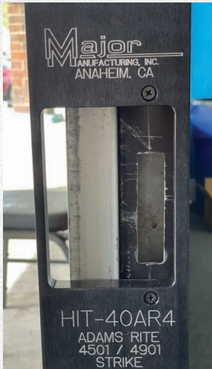
Figure 16. The template is mounted to the door with two screws. These holes are repurposed for mounting the strike support bracket.
