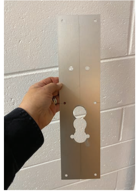
Figure 5. This is one of the three plates the author made for the inside holes.
