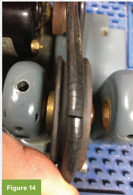
Figures 14 and 15. The old belt was a little sketchy (Figure 14), so the author installed a new one (Figure 15).
