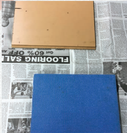
Figure 11. The laminate and the mat are shown prior to being sprayed with the contact adhesive.
