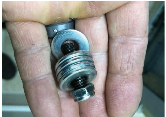
Figure 6. This bolt fell out and got jammed inside the boltwork, locking up the safe.
