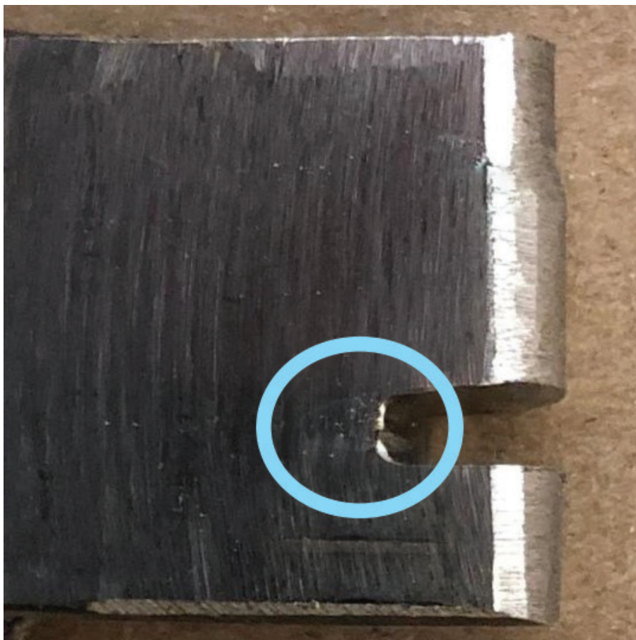
Figure 18. The impression marks are circled.
