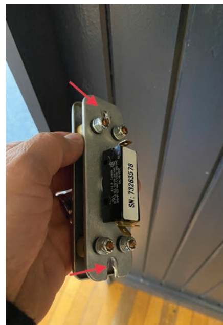
Figure 25. The red arrows point to the keyhole where the loosened screws pass through.
