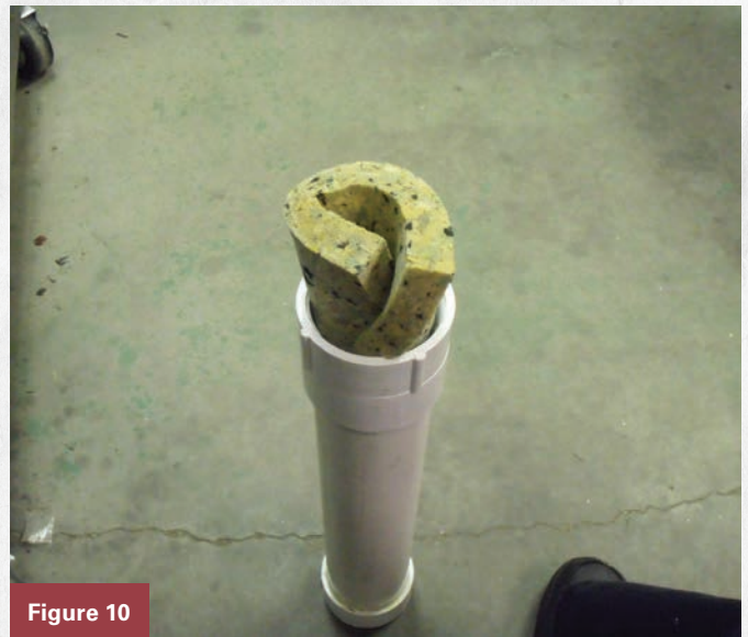
Figures 9 and 10. The author used this material in the pipe to stop the magnet from moving.
