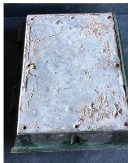
Figure 8. The screws are removed, and you can see the plaster of paris.
