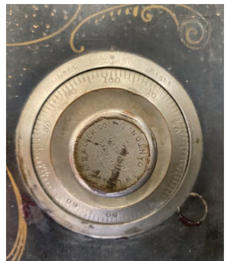
Figure 29. The drilled hole at 65 is repaired.
