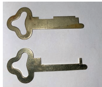
Figure 22. The top key is a prepped blank, and the bottom key is a pick key.
