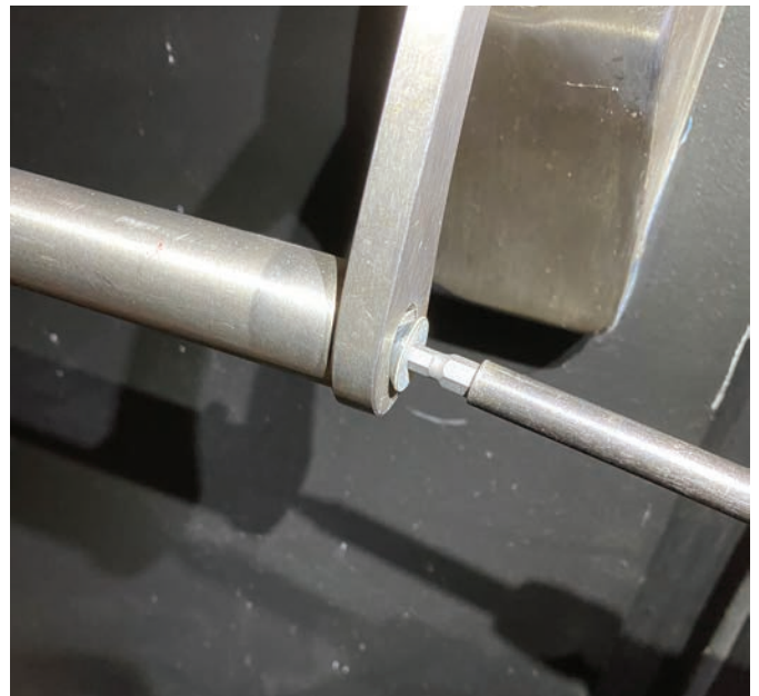
Figure 6. The author is removing one of the screws that holds the “drop bar” on.
