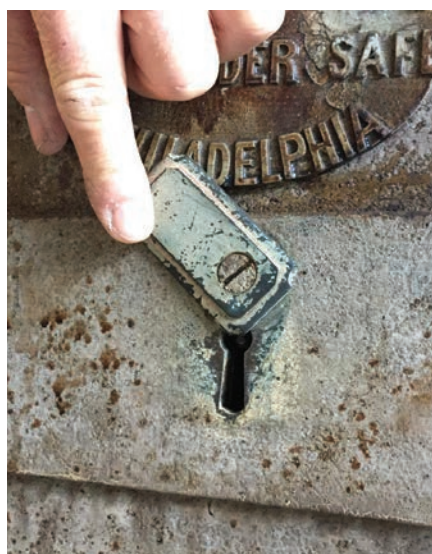
Figure 7. The cover plate is rotated to reveal the keyhole.
