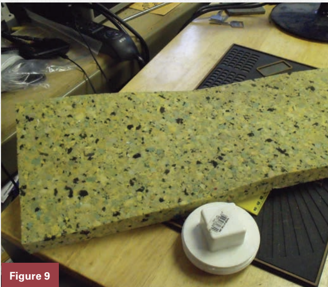
Figures 9 and 10. The author used this material in the pipe to stop the magnet from moving.
