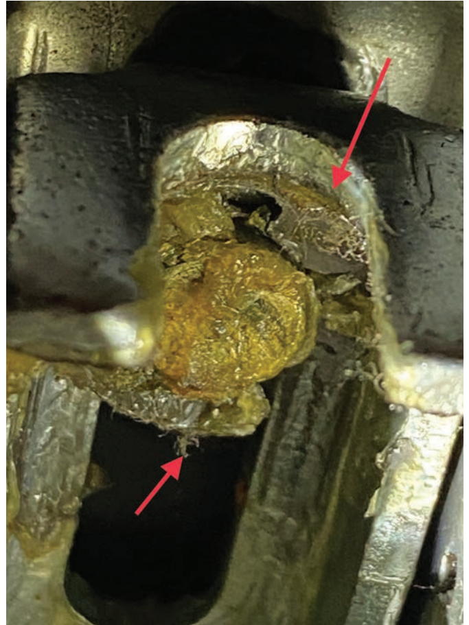
Figure 8. The two red arrows point to either side of the "E" clip that attaches the head to the two rods.
