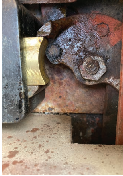
Figure 15. The lock bolt is extended.
