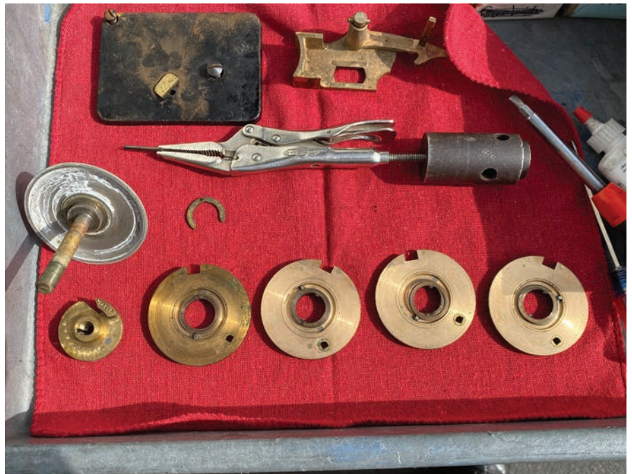
Figure 18. The lock is in exploded view, showing the 2.5" wheels.
