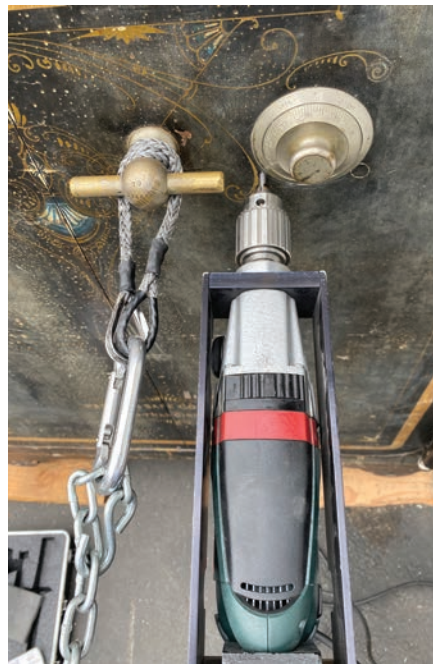
Figure 8. The author is using the Adams rope with lever rig to drill the scope hole.
