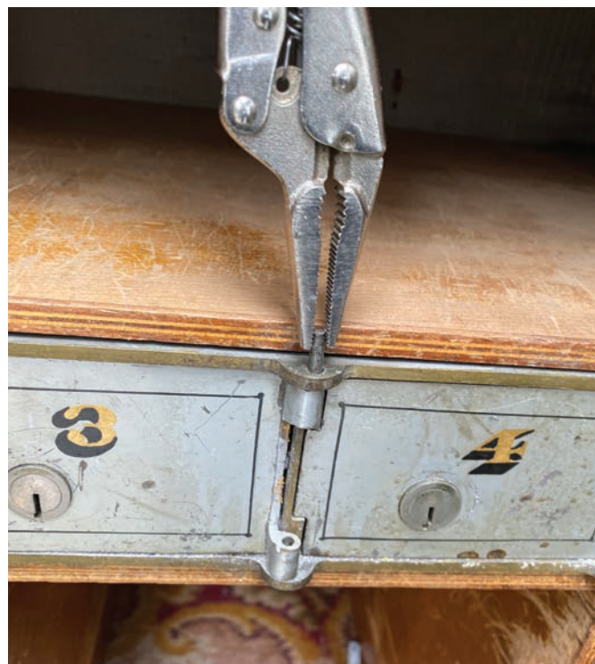
Figure 20. The modified Vise-Grips from Figure 18 are removing the hinge pin.
