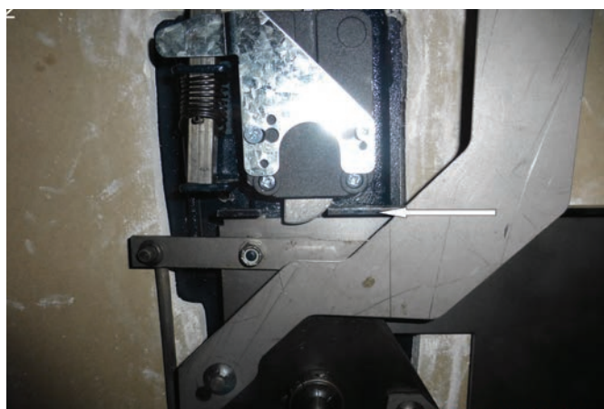
Figure 2. The arrow shows the direction the carrier bar needs to move to unlock the safe. Because the carrier bar is contacting the curved side of the swing bolt, it cannot push the bolt into the lock case. The do-it-yourself customer violated rule No. 1: Always test the lock while the door is in the open position.
