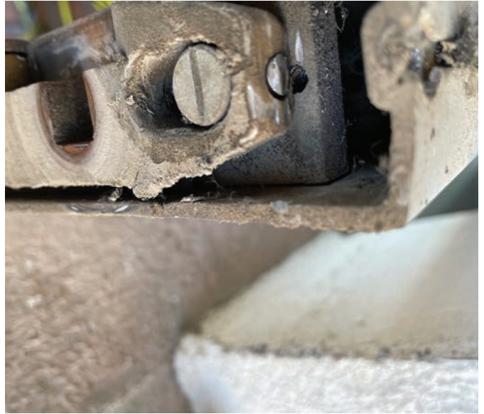
Figure 6. This one had damaged threads on the top centering adjustment screw. I used a Dremel with a cutoff disk to cut the screwhead off. Damaged threads happen from time to time when someone doesn't loosen the holding screw and then tries to adjust the horizontal adjustment with the screw.
