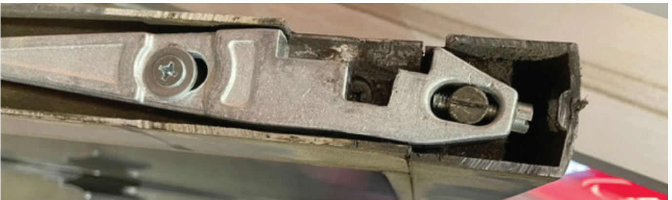
Figure 9. This arm was damaged during a high-wind event, pushing the door open beyond 105 degrees. It broke the closer arm bracket and bent the arm.
