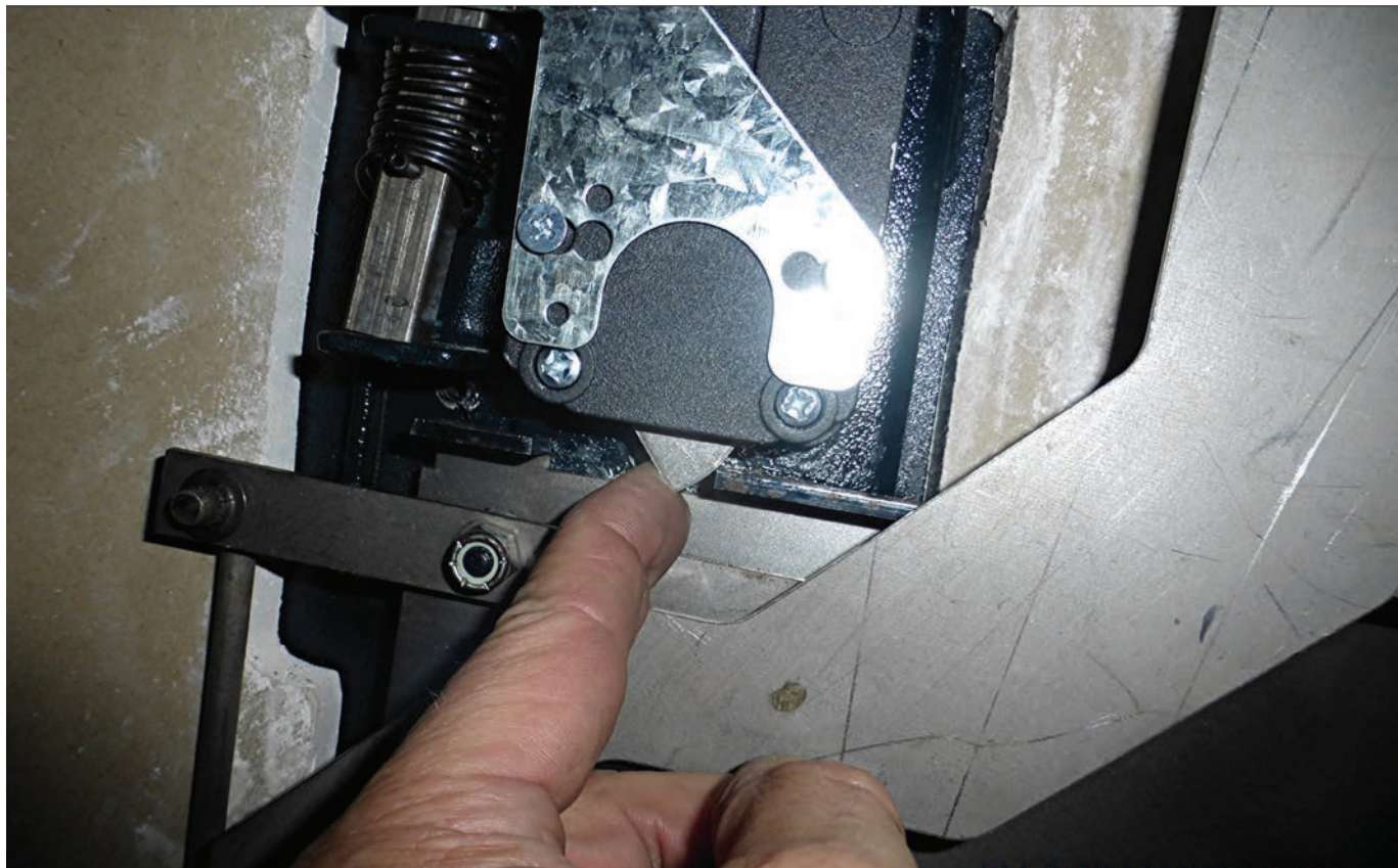
Figure 6. The author was perplexed about how the customer unlocked the safe after installing the new lock. The only way possible was the swing bolt was deliberately pushed in with a finger or tool, which should have alerted the customer that he didn't install something correctly.
