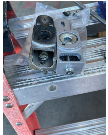
Figure 14. The same winds that bent the closer arm in Figure 9 caught a different door and broke the end of the bottom pivot that controls vertical adjustment of the pivot. The screw is accessed through a hole on the edge of the door. It tightens a wedge to move the bearing up or down.
