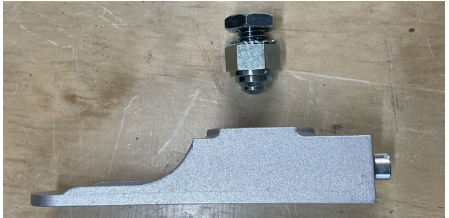
Figure 12. This bottom half of this pivot is installed in an aluminum threshold. The door portion is also shown for reference.
