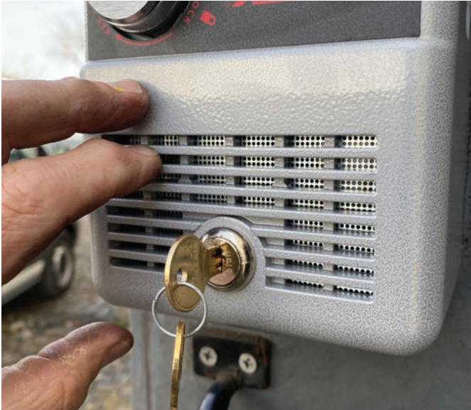
Figure 29. The key cylinder that holds the cover on is tightened.
