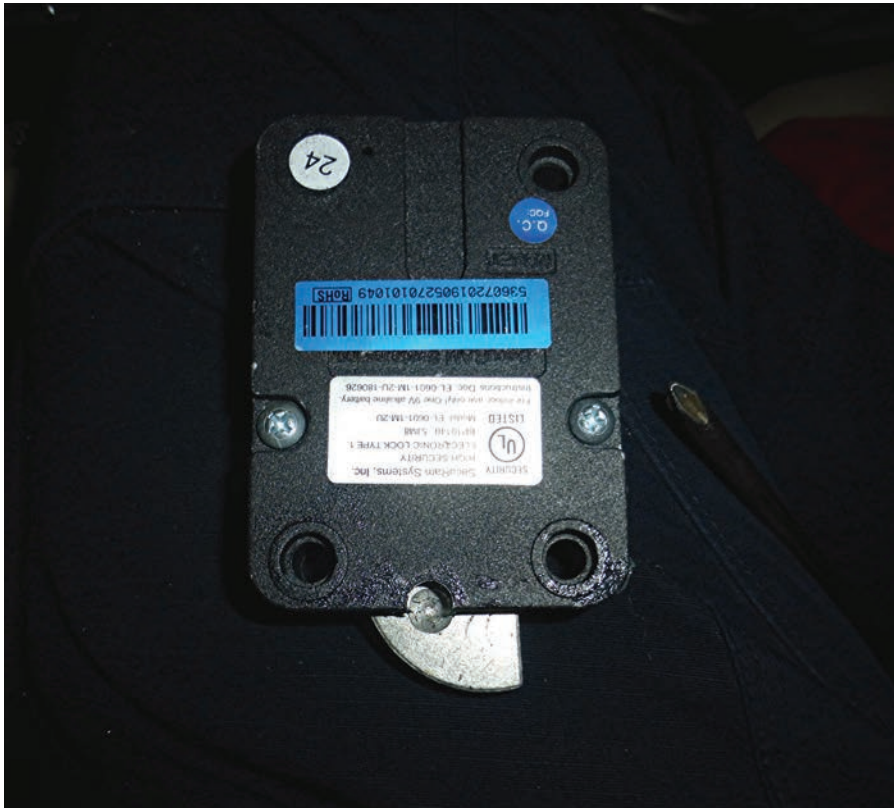
Figure 5. This photo shows where the drill contacted the swing bolt. The author could have drilled 2½" down from the dial center and still had plenty of swing bolt to probe with an ice pick without hitting the lock case.
