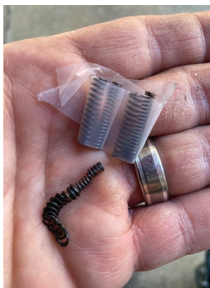
Figure 6. A damaged spring is shown with a pair of new springs.
