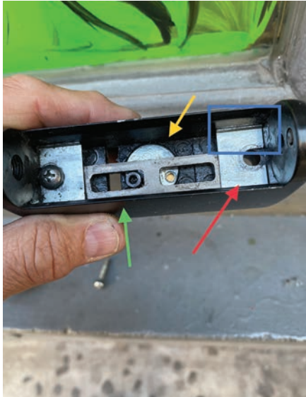
Figure 11. The red arrow is pointing at a thin metal plate that covers the springs and keeps them place.
