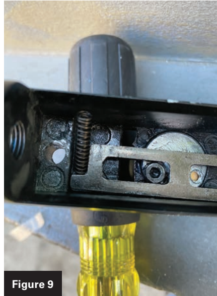
Figures 9 and 10. The double springs are being inserted into the escutcheon and then pushed down.
