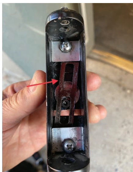
Figure 5. The driver plate's appearance means that the springs are crushed, broken or out of place.
