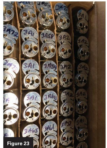
Figures 22 and 23. The author uses a fine pen-like Sharpie to write the core mark on the back so it’s easily readable.
