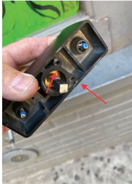
Figure 12. The two red arrows point to the holes that fit over the pins projecting out of the cam in the lock that retracts the bolt.
