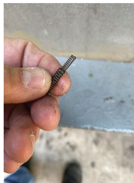
Figure 7. The smaller spring fits inside the other right before installation.
