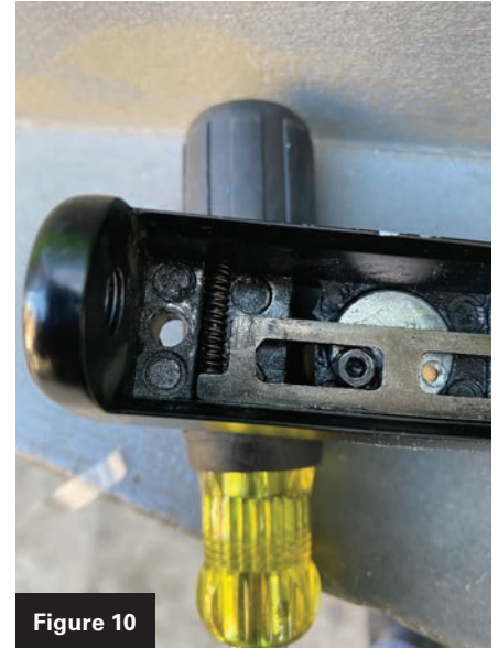
Figures 9 and 10. The double springs are being inserted into the escutcheon and then pushed down.
