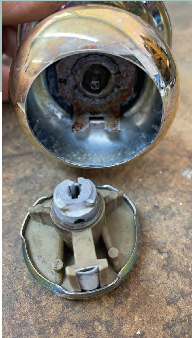
Figure 14. The cylinder was still retained in the same way as the older version: Pull the inner spindle and turn the key, or pick it to release the cylinder.
