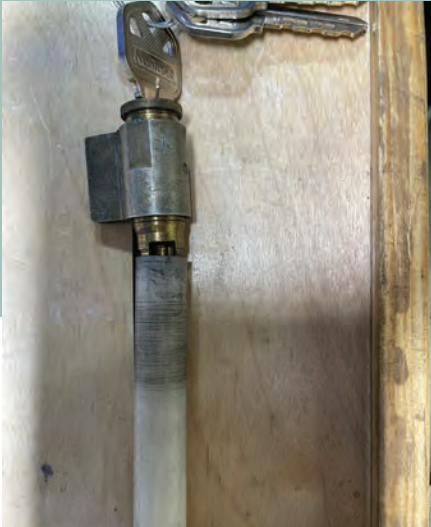
Figure 5. The back of the plug will not allow a standard follower to push the plug out without dropping the top pins. Instead of finding a hollow follower that might fit over the back of the plug, the author chose to use a shim to bridge the gap between the standard follower and the plug.
