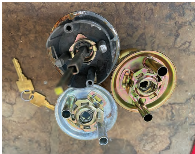
Figure 13. The back side of the knobs shows the inner spindle on the newer-style lock and the two different knob styles. This lock and both knobs were sent to the author by Jerry Cartmill.
