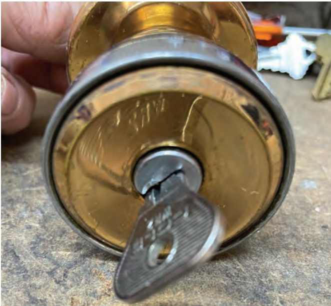
Figure 8. On to the next lock. This is an older Weiser lock loaned to the author by Anthony Leonardo of the Acme School of Locksmithing via Michael Bronzell for this article. In normal operation, the key only turns about 20 degrees to unlock. To lock the outside, push in and turn the entire knob. These locks were produced when Weiser was in still in South Gate, CA, back when they produced every part of the lock in the factory, including the screws. Somewhere around the late 1970s, they moved their factory to Huntington Beach, CA. In 1988, they announced they were closing the Huntington Beach factory. They have made them in other parts of the world and are now owned by the same corporation as Kwikset.
