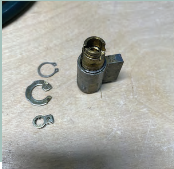
Figure 4. The back of the plug has an external retaining ring that must be removed. Then the retaining cam and a pair of cams are removed. It also has the typical retaining clip to hold the plug at the cylinder.
