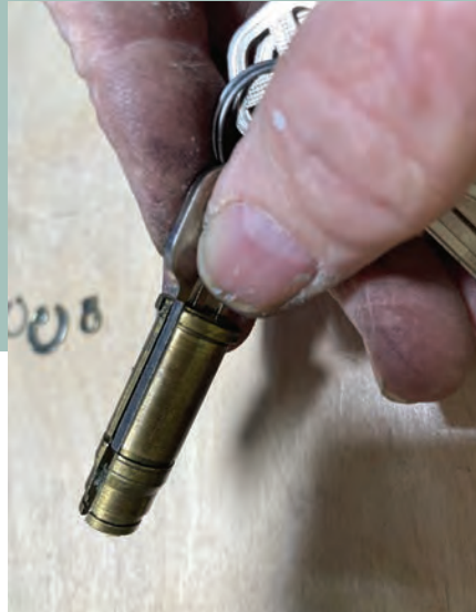
Figure 6. Keying the plug with standard pins lengths did not work; the author needed to drop the pin length by .015 to operate correctly. The key does not sit all the way to the bottom of the plug as seen in the photo.
