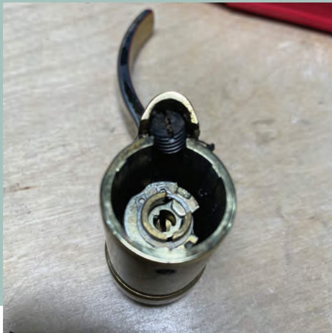
Figure 3. The cylinder is inside the lever. You can see the slot or cutout in the cam on the back of the plug. There is a set screw that retains the cylinder in the lever.
