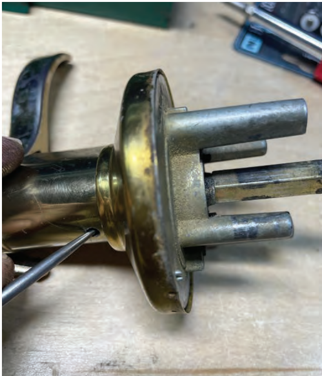
Figure 1. There is nothing special; just your typical retainer push-in tab. It goes in when the lock is unlocked and does not go in when the lock is locked, just like you might expect.
