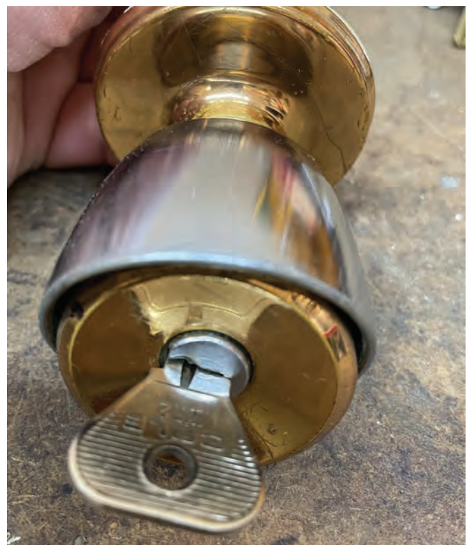
Figure 9. Pulling out the inner spindle allows the key to turn farther, allowing the cylinder to come out. When this lock model was still being produced, Weiser made a shim that slid alongside the key to push the inner spindle without having to take the lock off the door.
