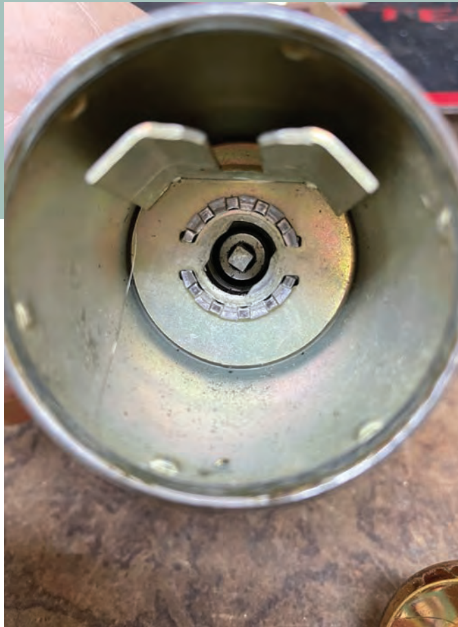
Figure 10. There's a view of the retaining plate inside the Weiser knob.
