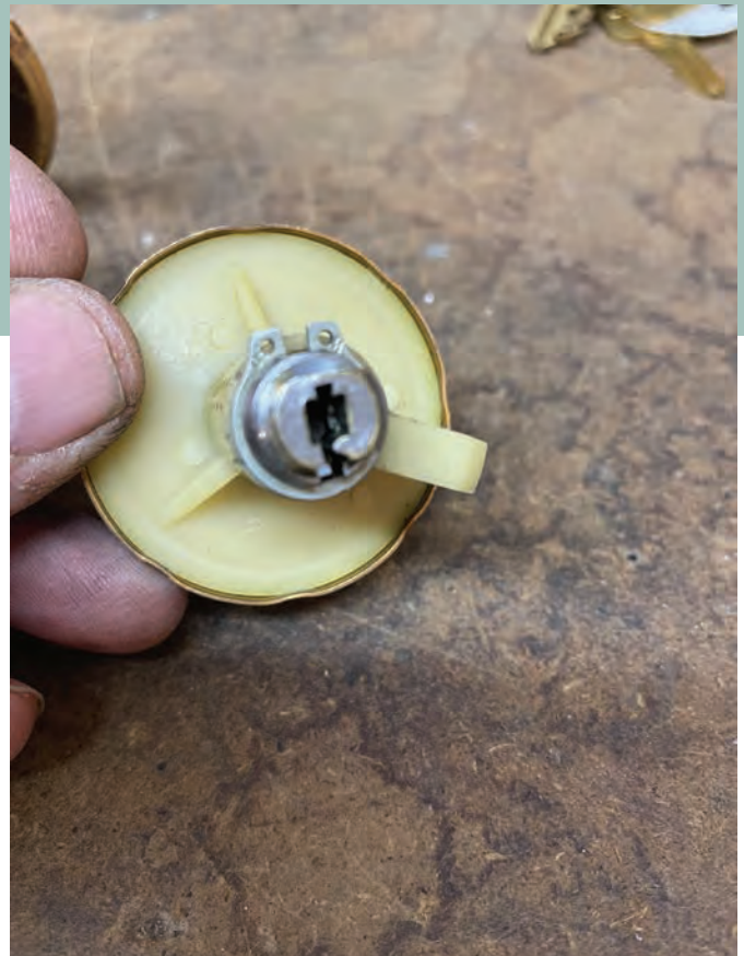
Figure 11. This is the back of the plastic cylinder with the flats on the back of the plug that need to align to remove or install the cylinder.
