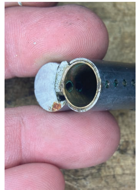
Figure 3. You can see how gummed up the core is.
