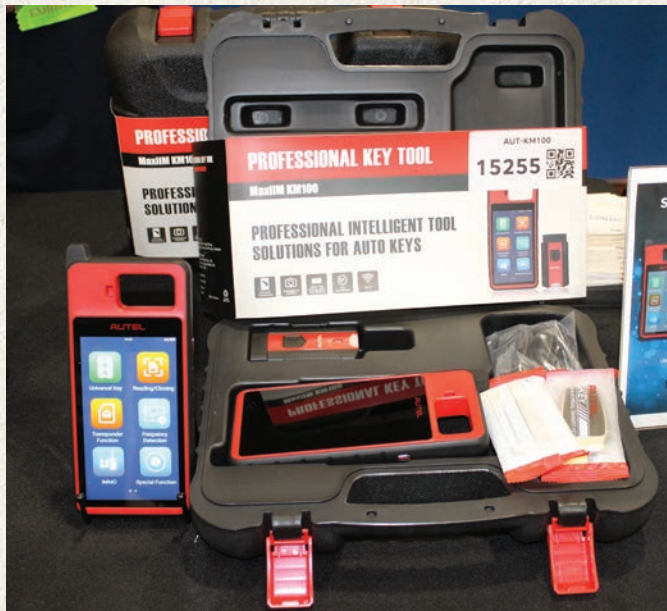
Figure 30. Autel is now shipping the KM100 tool, which is not only an OBD programmer but also a cloning tool. It was the talk of the show for the automotive locksmiths. Go to Autel.com or your favorite distributor for more information.
