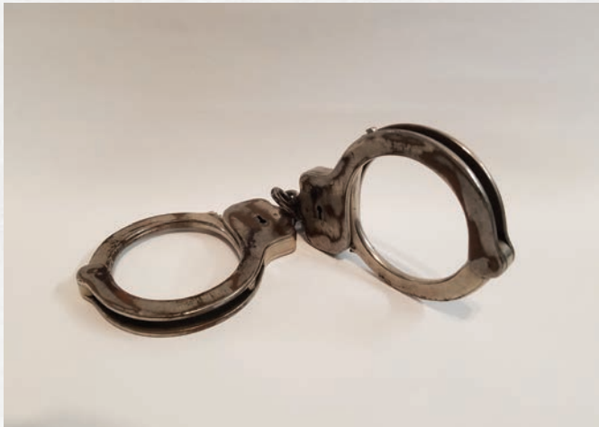
Figure 4. The Carney patent acquired by Peerless effectively changed everything with the adjustable swing through design and streamlined shape of its handcuff. This model double locks through the keyhole, while later models used a more convenient external plunger.
