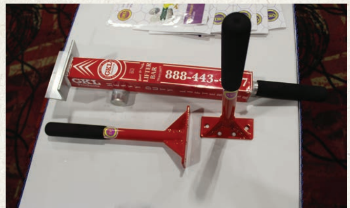
Figure 20. GKLI Products offers some great time-saving tools. This year, the company showed the latest product for moving or realigning the hinge mounting plate inside the hollow metal frame. Next to it in the picture is another great tool for lifting doors. More info can be found at gklproducts.com .
