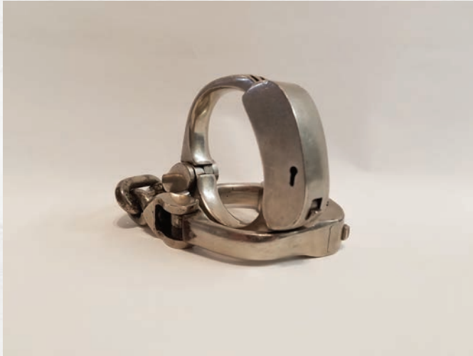
Figure 2. The Bean handcuff had double latches (although no true levers) that offered better security, was adjustable and had arming buttons to keep the handcuff ready until the officer needed them.
