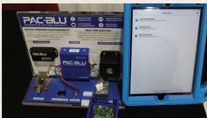
Figure 6. Pac-Blu is a new access control system from Pacific Lock. This is a small Bluetooth module that is programmed with your server or computer, then transferred to your phone for the next time you connect to the Pac-Blu module. It offers you the ability to earn some recurring revenue from your customer with the annual subscription. Paclock.com is the web site.
