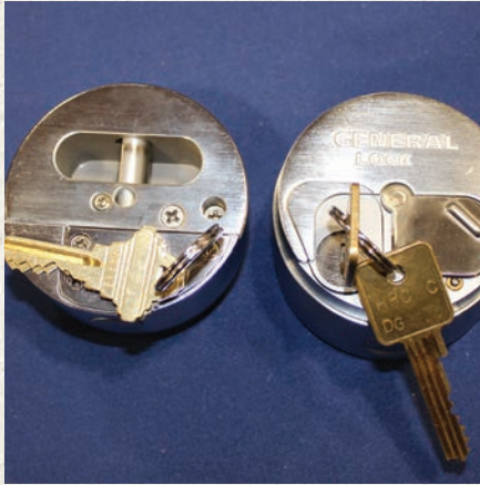
Figure 8. General Lock has a new padlock in its line. These are hockey-puck-style locks — one that accepts the cap-nut-style, six-pin KIK cylinder and a second that accepts six- or seven-pin SFIC cylinders. Both have shrouds to better protect the cylinders from being pulled with a slam hammer. They have an easy web site address: generallock.com .
