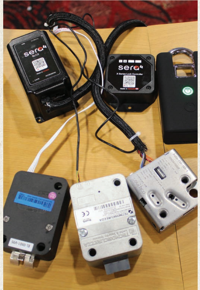
Figure 22. The Sera4 can control safe locks, padlocks or door locks via Bluetooth with a single interface module. You can find more information at mbausa.com.
