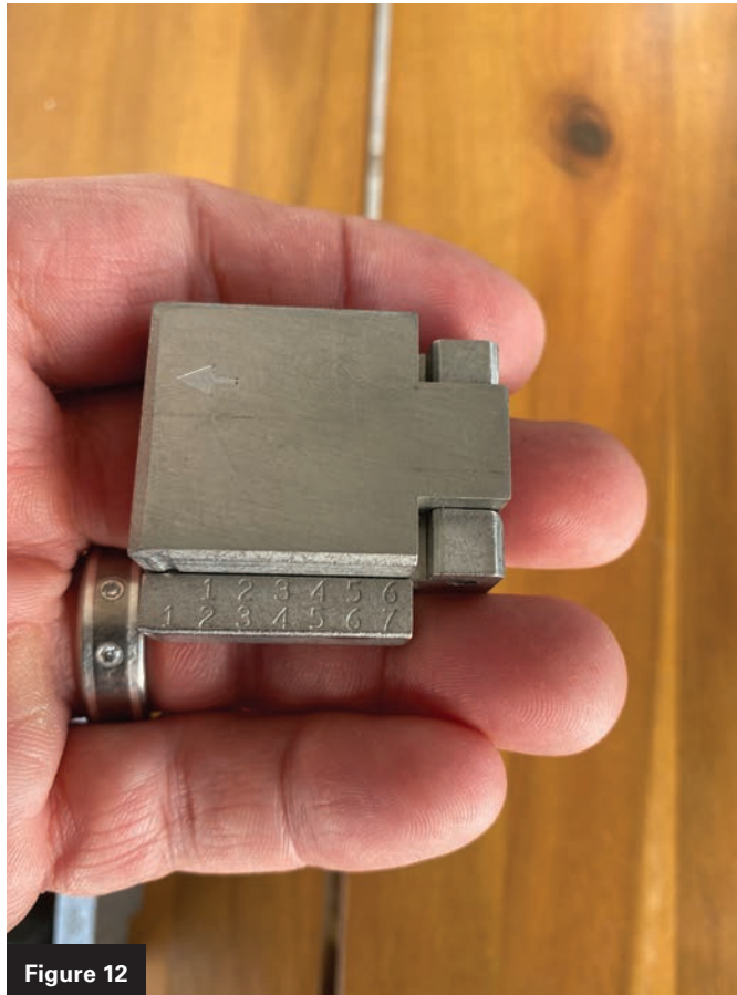
Figures 12 and 13. The pin stacks can be unloaded into a “book,” shown closed in Figure 12 and open in Figure 13 .
