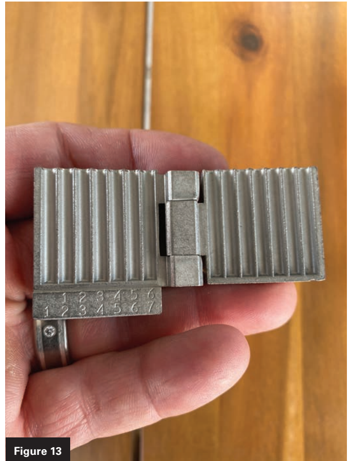
Figures 12 and 13. The pin stacks can be unloaded into a “book,” shown closed in Figure 12 and open in Figure 13 .
