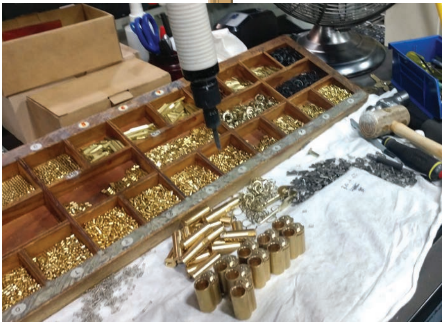
Figure 1. This is a pinning bench at the plant, shown with cores.
