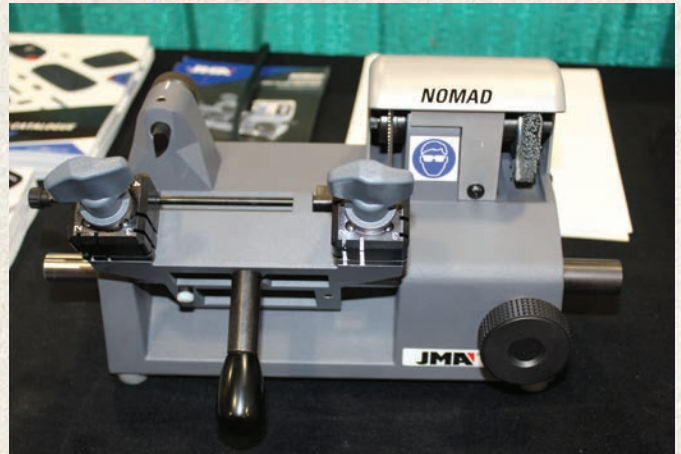
Figure 34. The JMA Nomad is designed to be portable and is simple to operate in a very small footprint. JMA offers a wide range of other key machines on jmausa.com
