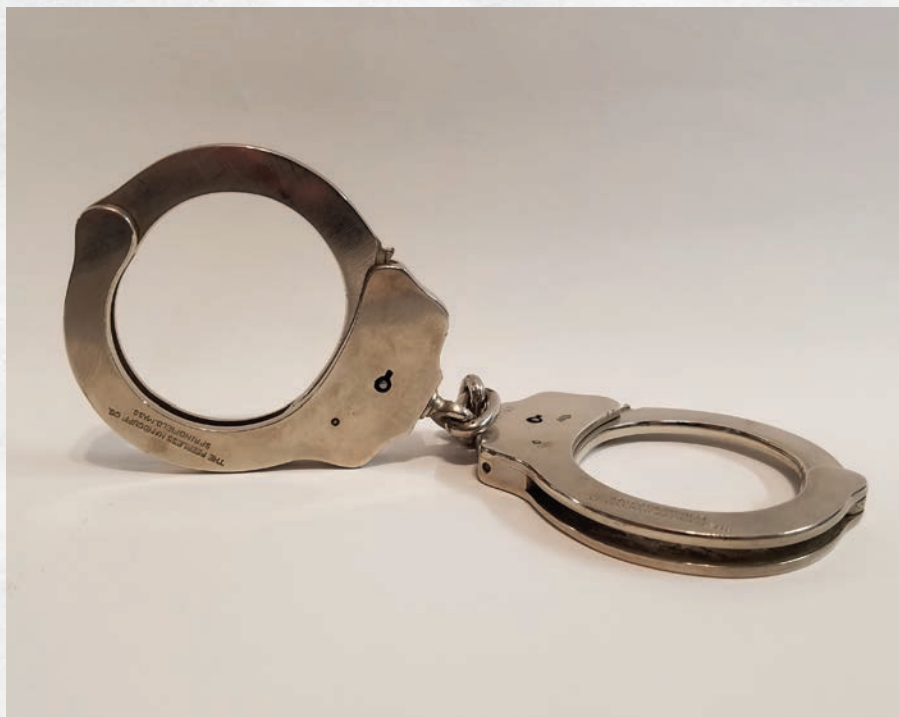
Figure 7. While still susceptible to shimming in single lock and picking in double lock, modern Peerless handcuffs rank high for ease of carrying and quick effective application to the detained. This model double locks externally with a plunger by the key, not through the keyhole.
