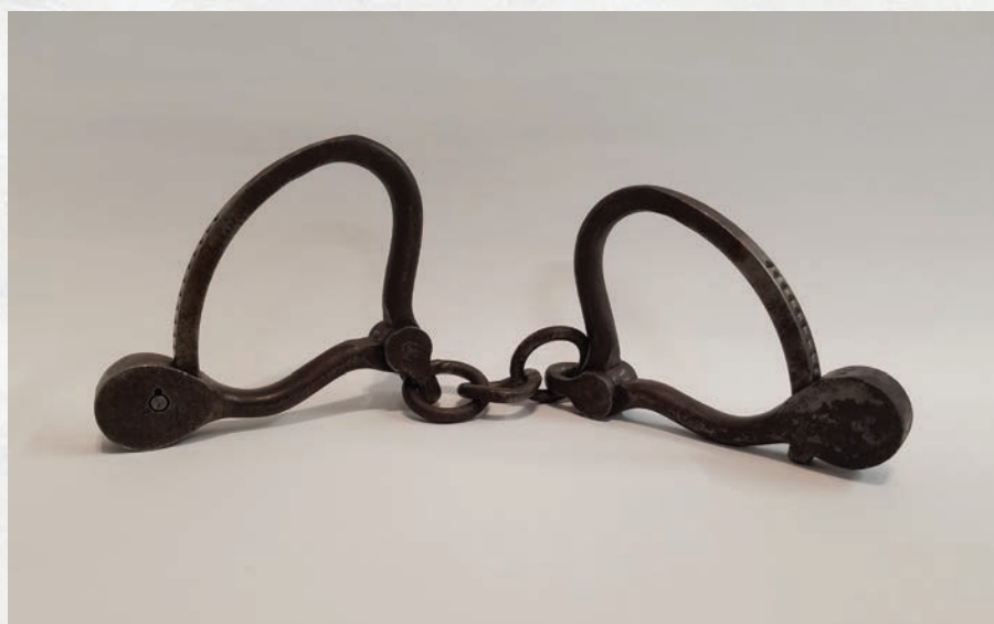
Figure 1. The Adams handcuff was America’s first adjustable model. It was single locking (could not deadlock the bow) and gained security from its very narrow keyway, which helped protect its simple mechanism.
