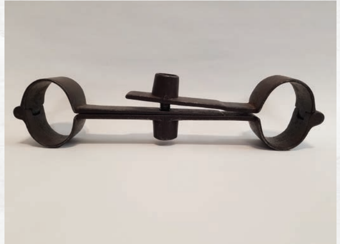
Figure 11. Famous for the pictures that depict its use on the Lincoln conspirators, the screw locking Lilly iron handcuff was nonadjustable, large, heavy and devoid of springs.
