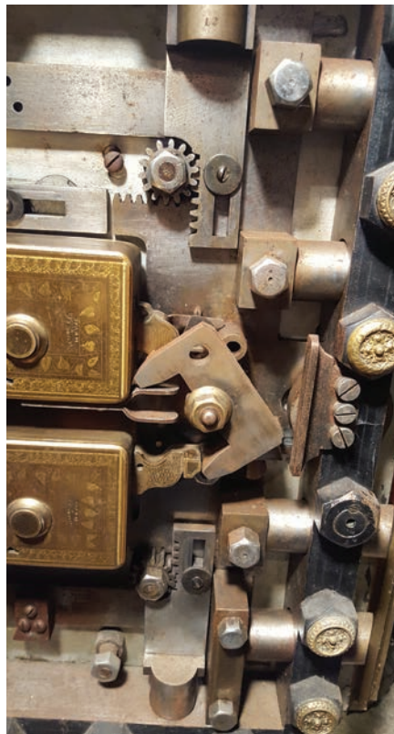
Figure 17. The top lock is unlocked, and the bolts are retracted.
