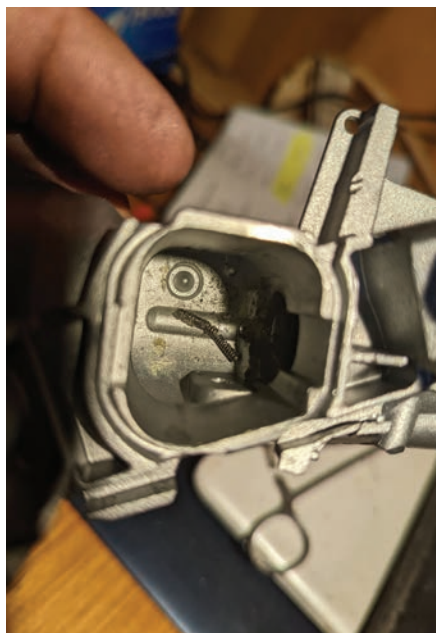
Figure 17. The offending spring is just hanging out after shooting the pin through the housing.
