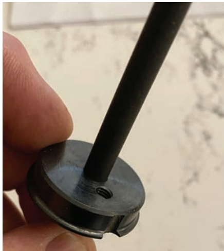
Figure 5. The lip on the outside part of the disc keeps it from falling into the chassis of the lock.
