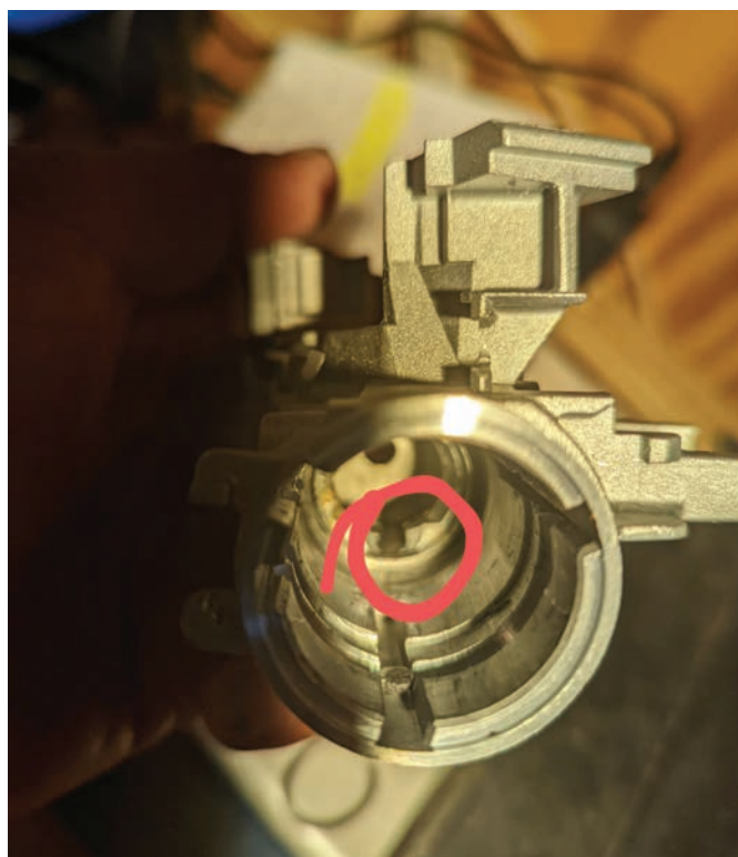
Figure 2. This is the spot in the housing where the pin breaks through.
