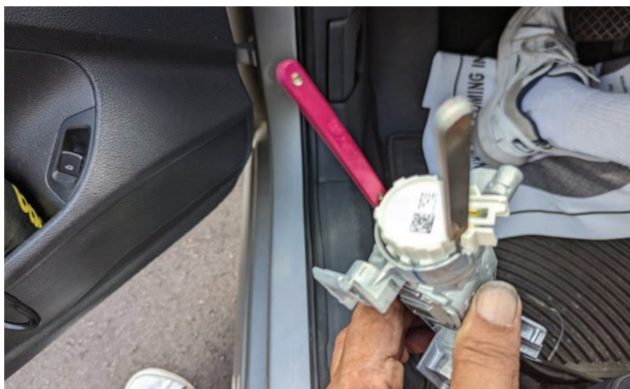
Figure 11. You can see the author using two broken picks to push the clips holding the switch in the back of the housing.
