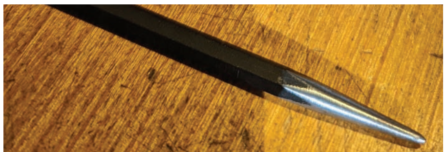
Figure 8. This is the author's preferred punch for removing the shear-headed bolts: one hit straight down to create a divot in the soft metal. Then change the angle and hit again to start it turning.
