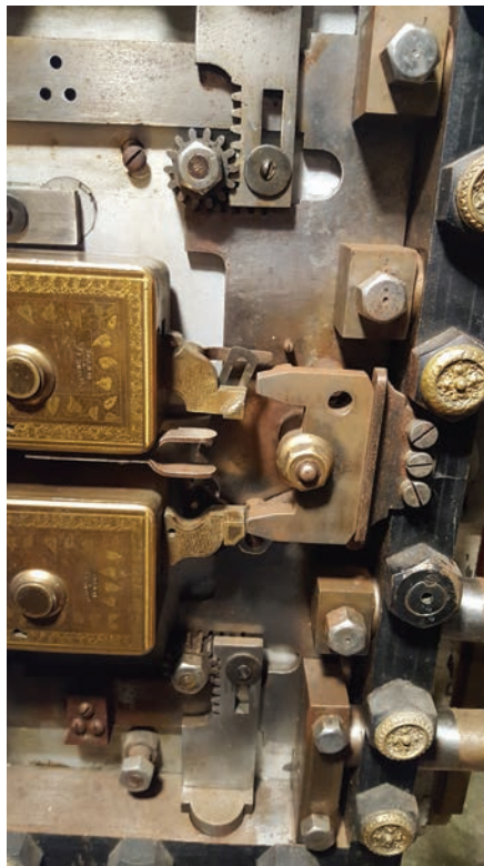
Figure 16. The front door locks are locked, and the bolts are thrown in the locked position.
