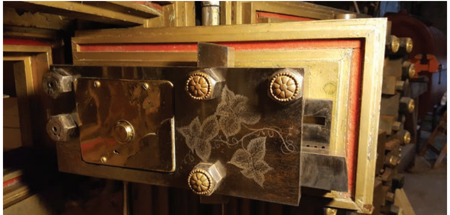
Figure 13. The inner door is shown, with the bolt thrown.
