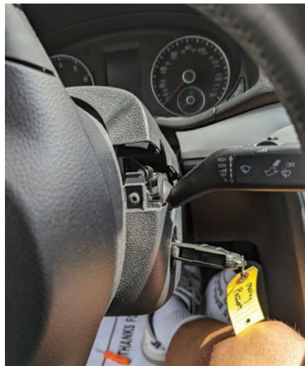
Figure 6. This is the right Torx screw behind the steering wheel.
