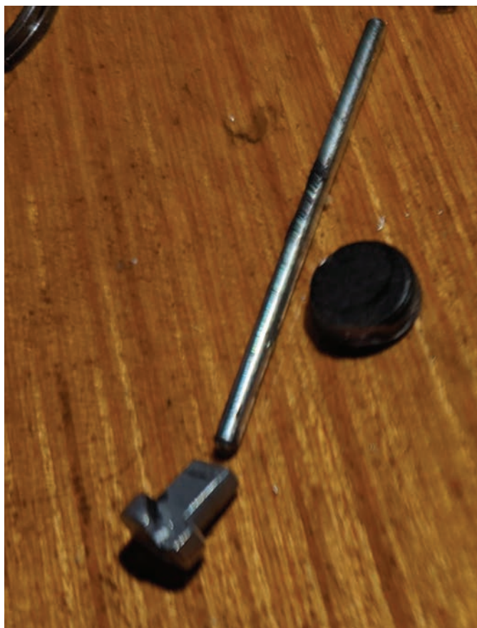
Figure 13. This is a close-up view of the relocker pieces to remove.
