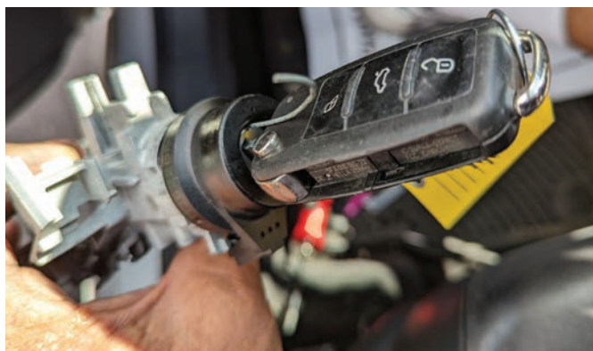
Figure 10. The ignition turned on, so the retainer can be accessed. The author's wire of choice is simply a straightened giveaway keyring, as it is a stronger metal than any paper clip, yet perfectly sized.
