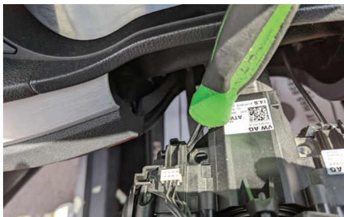
Figure 9. The author is sliding the screwdriver above the bracket and under the plastic to push the clip holding the housing in place.
