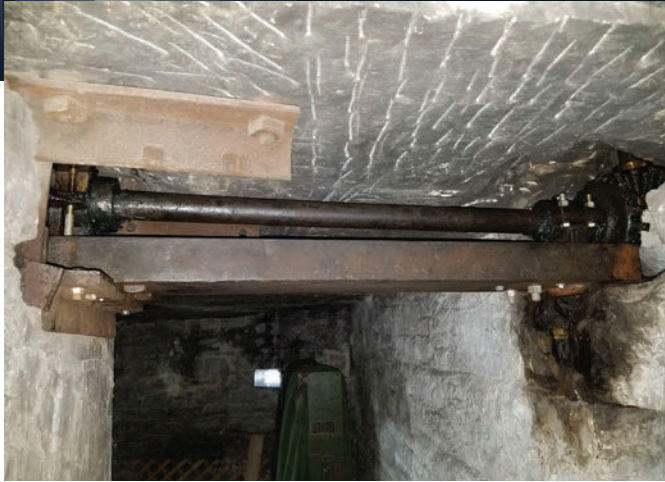
Figure 14. The horizontal drive shaft spans the corridor, linking the crank to the cells.
