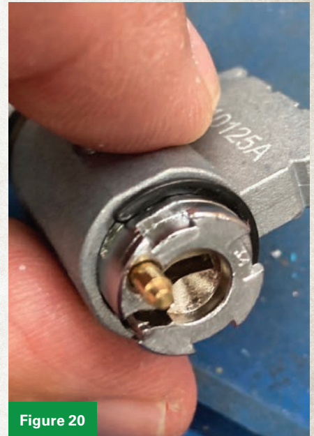
Figures 19 and 20. You can see the notches on the cylinder cap cam (Figure 19) and in the cylinder (Figure 20).
