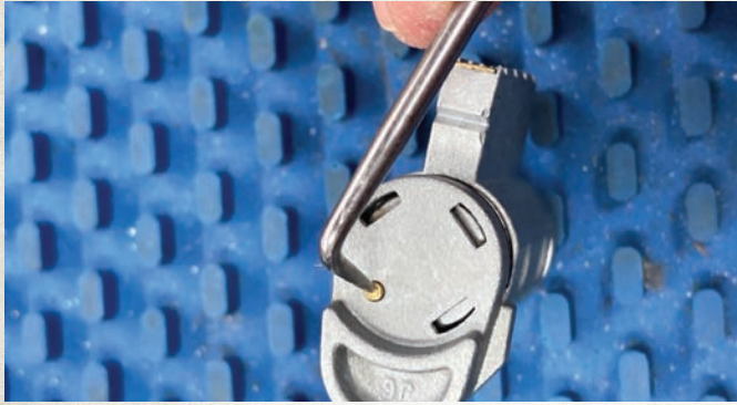
Figure 16. Press and push in on the retaining pin, as shown here.
