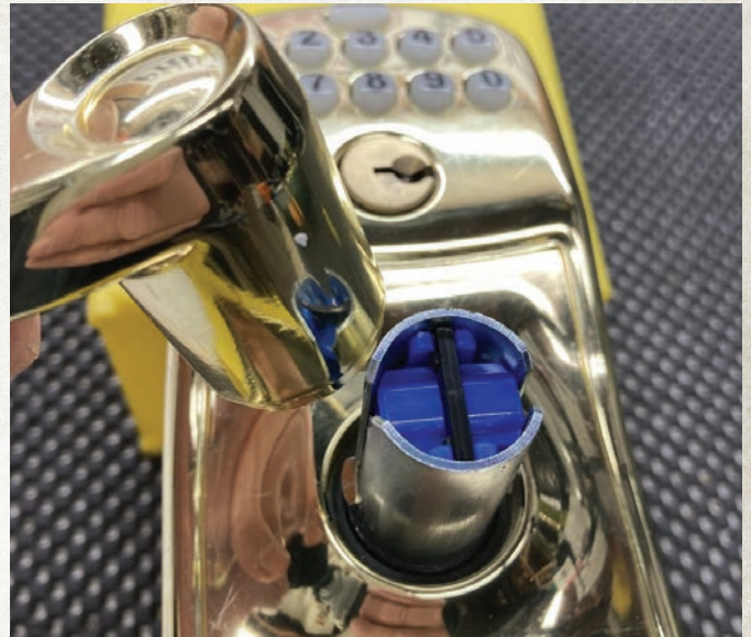
Figure 22. The author is removing the outside lever.
