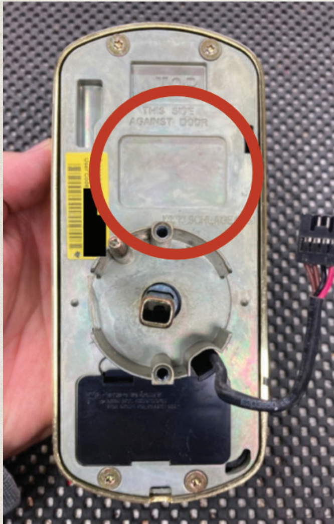
Figure 21. There's no back cover plate on this version.
