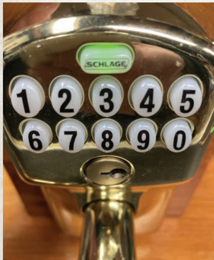
Figure 4. The green light means you've entered the correct code, or the programming is complete.
