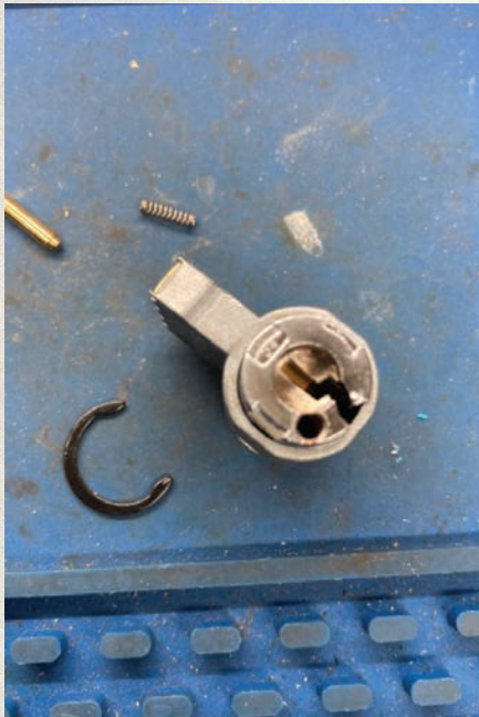
Figure 18. The retainer clip is removed.
