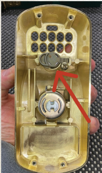
Figure 28. The cylinder is attached to the faceplate.
