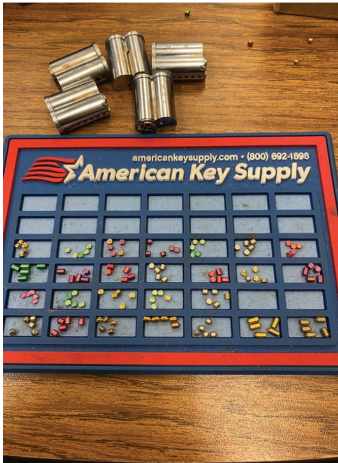
Figure 15. There are five pins in each slot — enough to pin the five cores.
