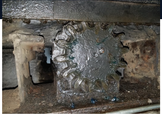
Figure 15. This close-up view shows the gear mating with the circular rack beneath the cellblock.
