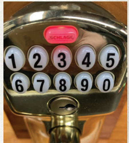
Figure 6. The red light indicates that the wrong code has been entered, there has been an error in the programming, or the battery is low.
