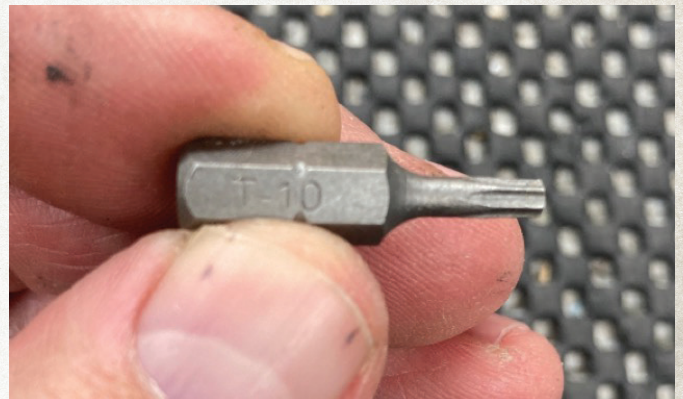
Figure 23. This photo shows a T-10 bit.
