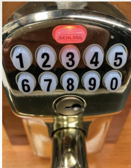
Figure 5. The orange light means the lock is in programming mode.
