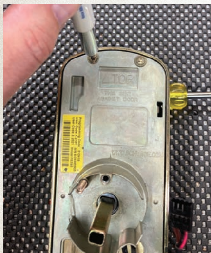
Figure 24. There are four T-10 screws to remove.
