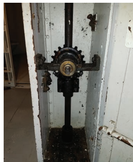
Figure 6. This close-up view provides a look at the shaft that receives the crank and the bevel gears.
