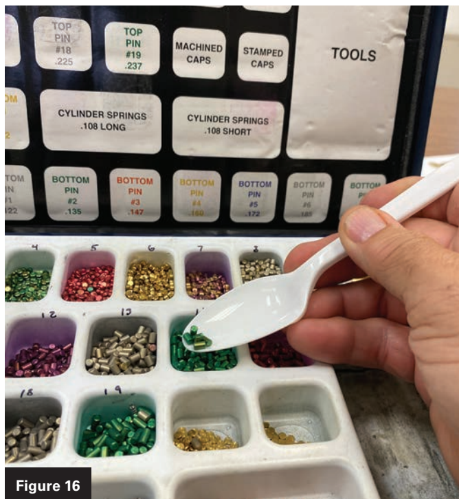
Figures 16 and 17. Using a plastic spoon to fill pinning mats can be more precise than using your fingers.
