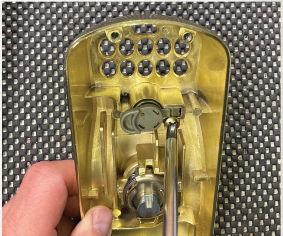
Figure 29. Finally, remove the cylinder.
