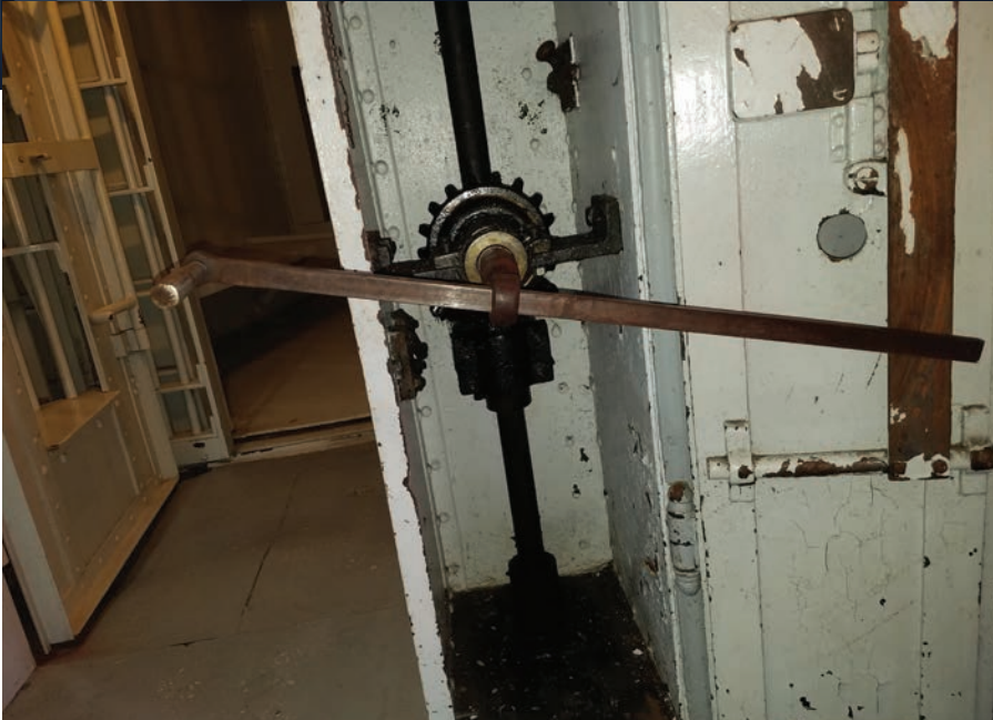
Figure 7. The 34" crank is used to move 30 tons of steel.
