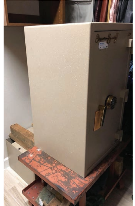
Figure 7. This image shows the safe being transferred to the pedestal. The author could not get the table to go down quite as low as the pedestal, so he used the 4x4s.
