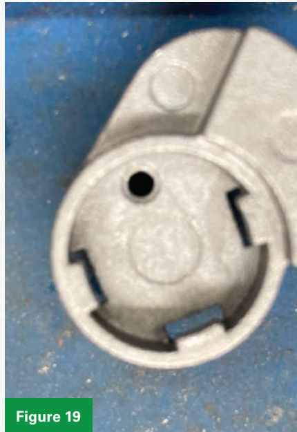
Figures 19 and 20. You can see the notches on the cylinder cap cam (Figure 19) and in the cylinder (Figure 20).
