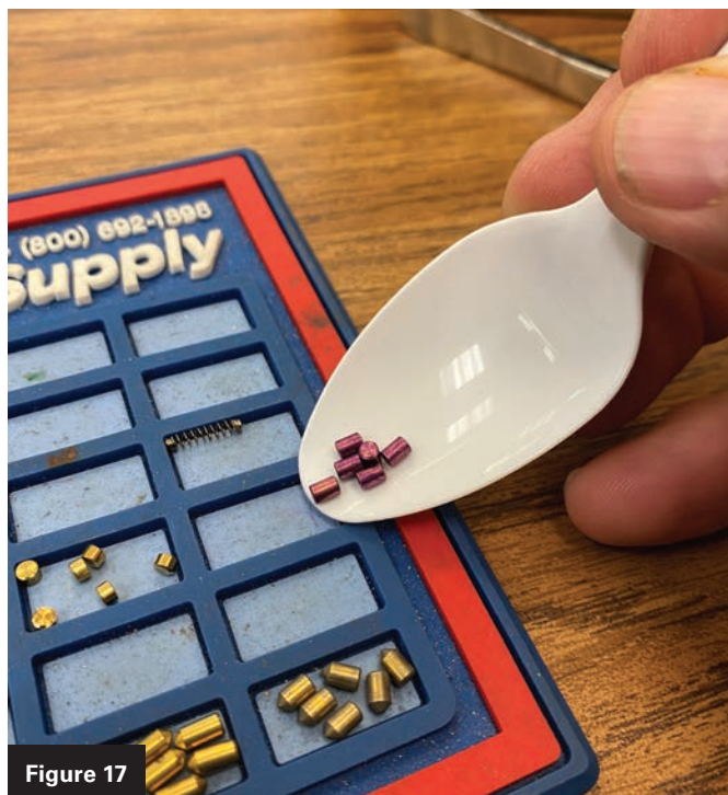
Figures 16 and 17. Using a plastic spoon to fill pinning mats can be more precise than using your fingers.
