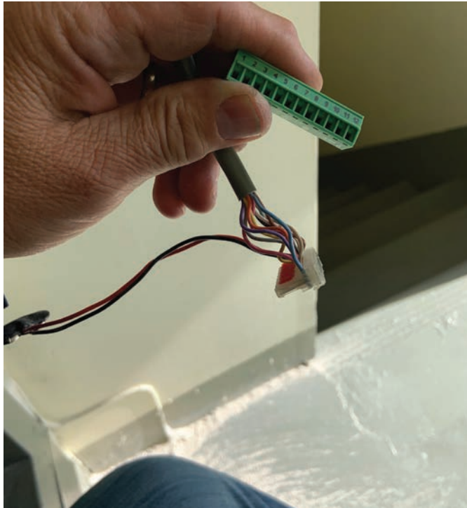
Figure 12. The newer model uses a green Molex connector.
