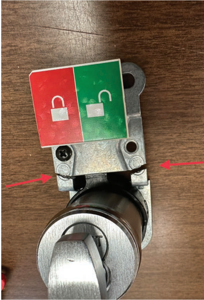
Figure 24. The arrow points to the cracks in the broken unit.
