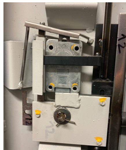
Figure 13. The locking screws have just been removed.
