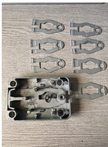
Figure 23. The levers have been removed.
