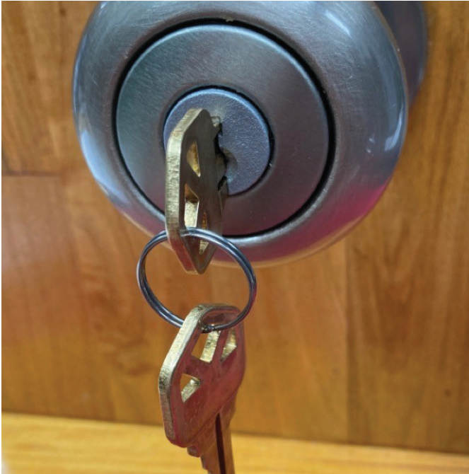
Figure 9. Turn the key to 12 o'clock and pull the key out of the cylinder. Then test the SmartKey to make sure that it operates properly.
