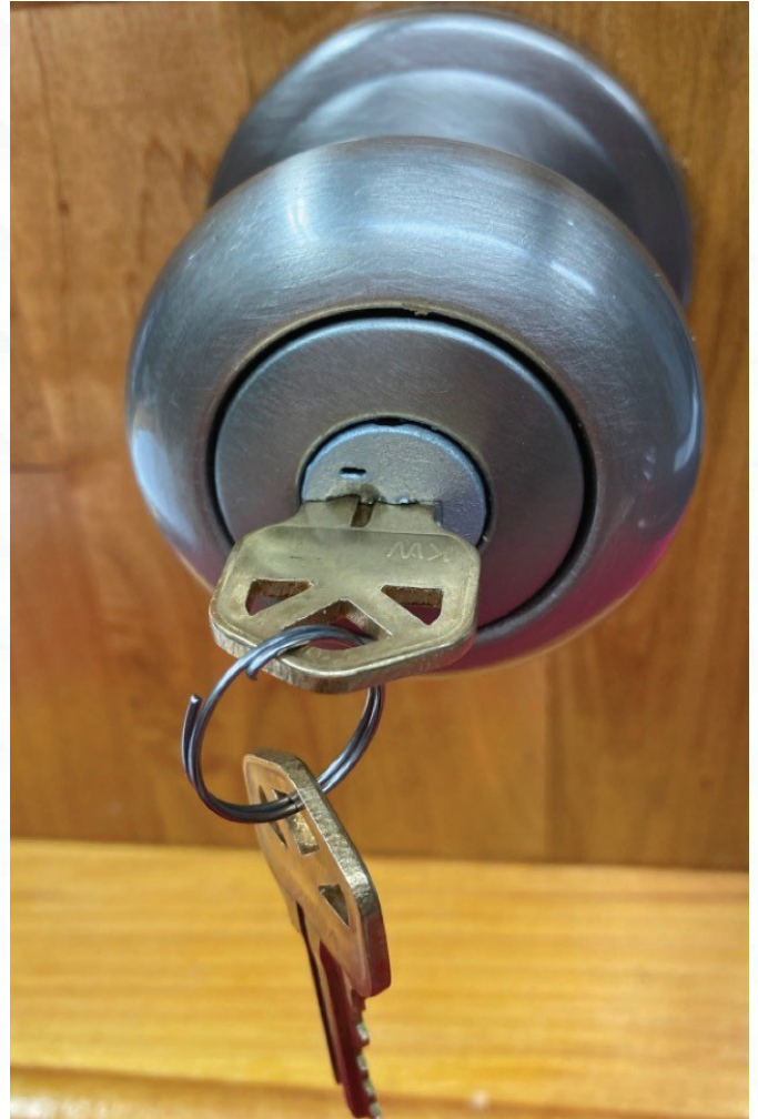
Figure 7. Insert the new key that you would like the lock to operate.
