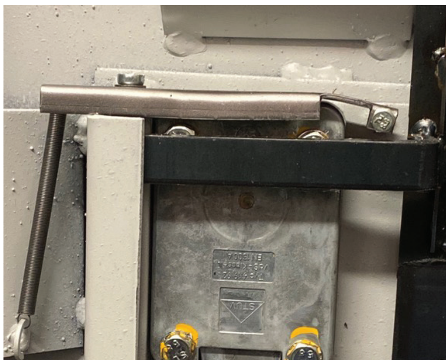
Figure 11. The lock boltwork covers the lock-fixing screws.
