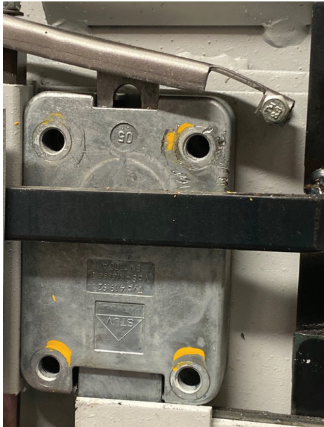
Figure 14. The original lock is open, and the bolt extends out of the back to lift the relock arm.
