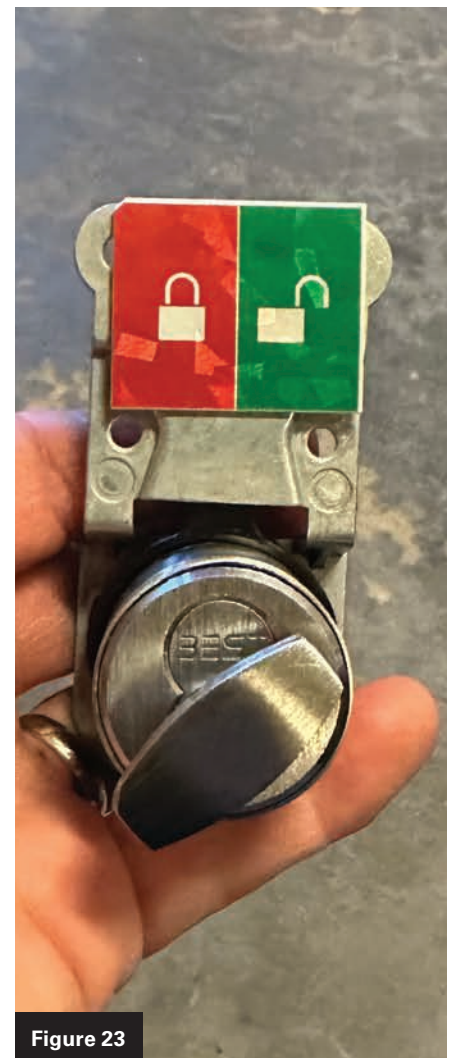
Figure 21. The part that moves over the finger lift to prevent it from moving upward is in the locked position.
