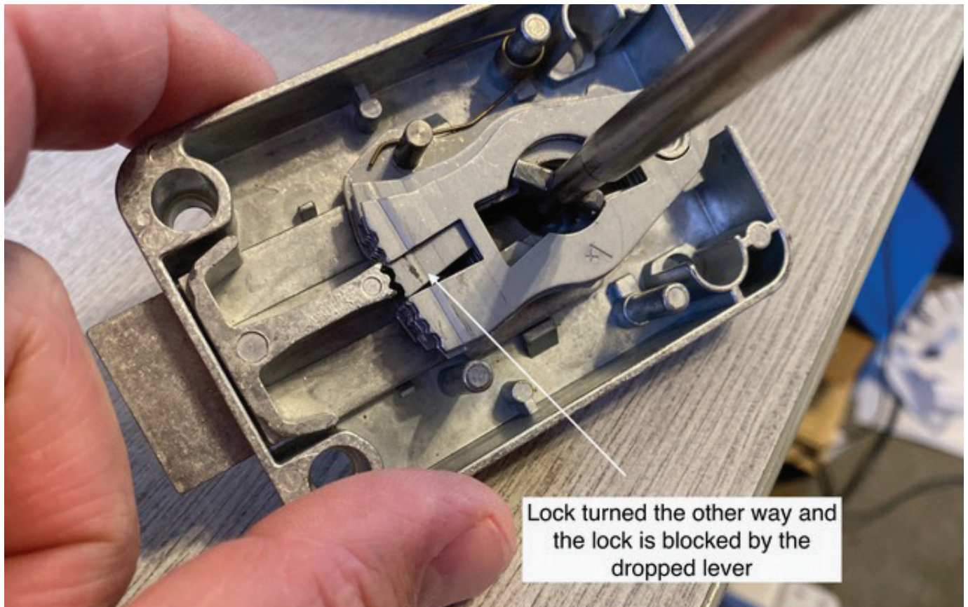
Figure 19. The lock is turned the other way with the customer's key, and it will not open.
