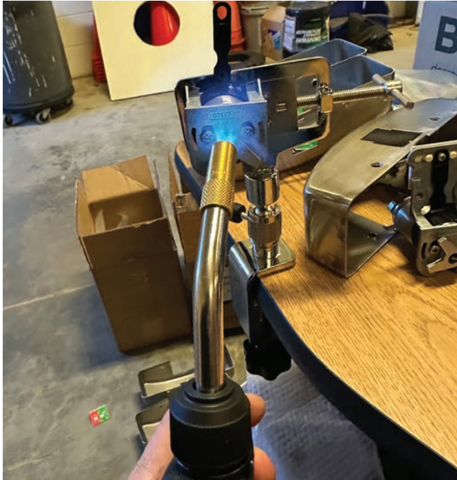
Figure 26. The author used a MAPP gas torch to break down/melt the thread locker.
