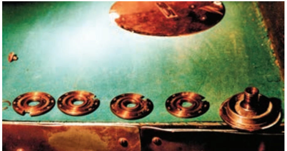
Figure 17. This lock is a Yale OB with four hand-change wheels. The author didn't take pictures of the other side of the wheels, but he doesn't believe they had dates on them. 🤖
