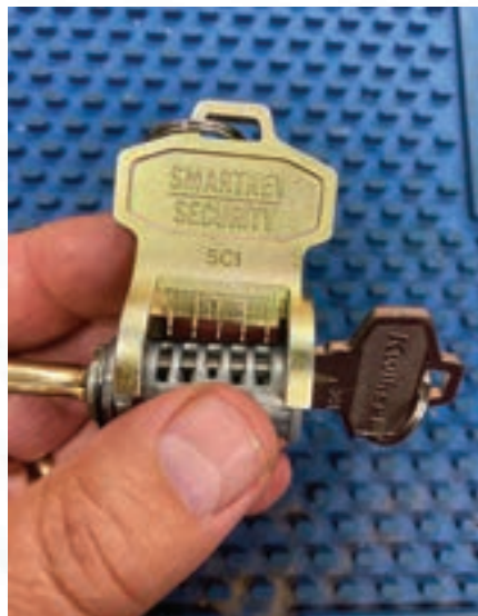
Figure 18. Align the five prongs with the five slots in the cylinder.
