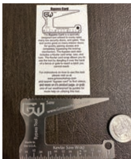
Figure 33. The Bypass card is designed to pull back latches in either direction on simple latches.
