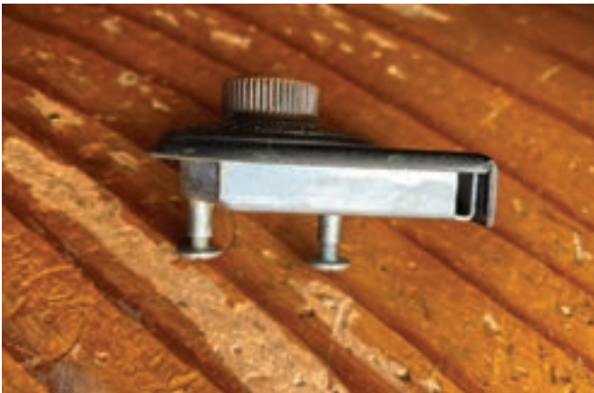
Figure 3. The lock is held onto the cabinet with two screws.
