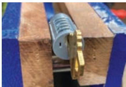
Figure 30. The author has inserted an uncut SC1 key blank.
