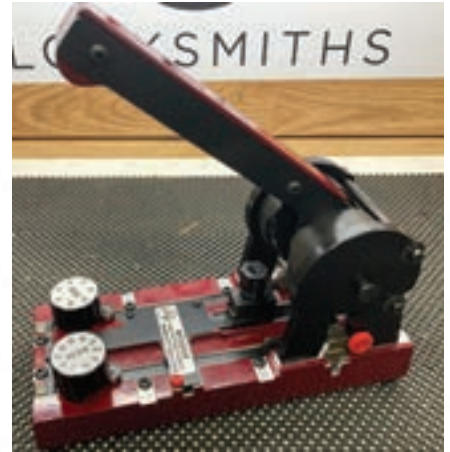
Figure 5. The author likes to use a Rytan punch to make the keys for both SC1 and KW1.
