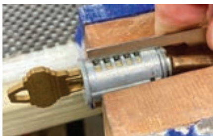
Figure 31. Align the prongs of the tool with the five slots in the cylinder, and press down and hold.
