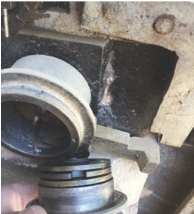
Figure 8. A close-up view of the Yale OB three-wheel lock shows the curb in the author's hand.
