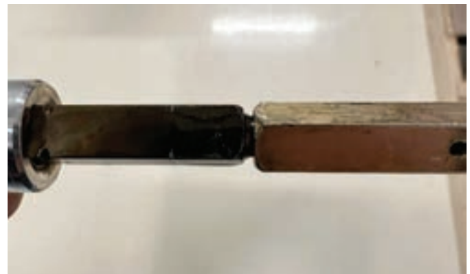
Figure 4. The spindles are backed off one complete turn.
