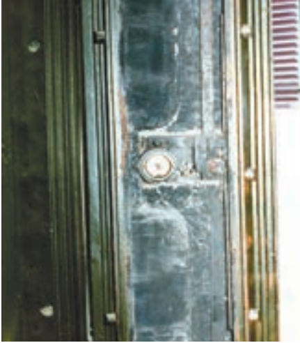
Figure 13. This one was drilled before. You can see all the holes between the lock and boltwork. The author's first hole location was chosen because perhaps he saw a patch and followed it. Sometimes that works out; other times (like this one), it was an air hole.
