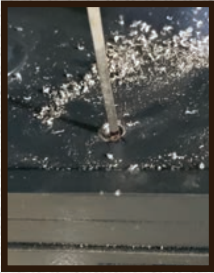
Figure 10. The author came up with a successful drill point of 3½" from handle center toward the hinges.
