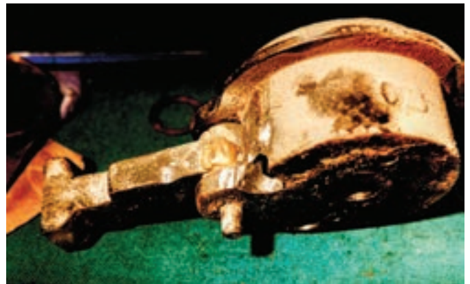
Figure 16. The author removed the lock case. You can see the hole he drilled into the case.
