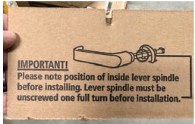
Figure 2. The installers apparently ignored these instructions.
