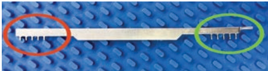
Figure 27. Circled in green is the end of the tool that is used for resetting the KW1 Kwikset SmartKey cylinder, and the one circled in red is used for both the SC1 Kwikset SmartKey cylinders and the Schlage SecureKey cylinders.
