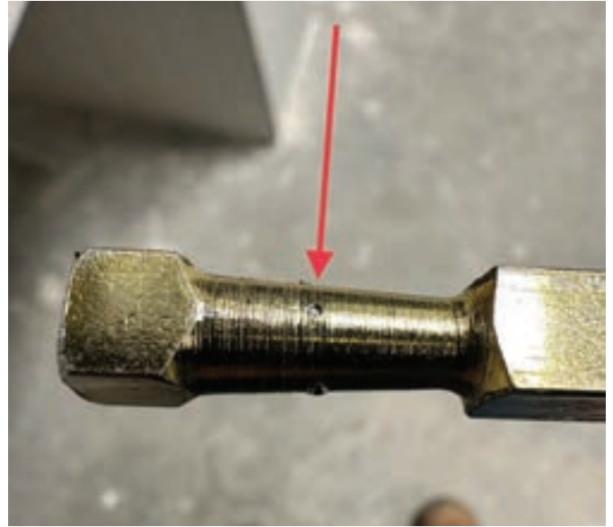
Figure 6. The mark made by the set screw indicated that this was the used part.
