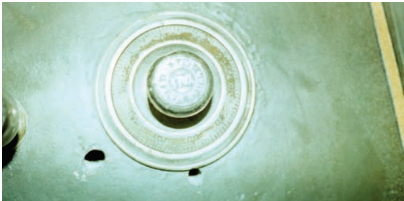
Figure 12. The author started the opening by drilling a hole between the dial and the handle, thinking it was a larger case, perhaps a roller-bolt-style lock. This ended up in open air inside the safe. But it did allow him to ID the lock as an OB-style lock. The second hole drilled 1\frac{3}{16} " allowed him to carefully enter the lock case and decode the combination. It has a four-wheel Yale OB lock. Today, the author would suggest drilling a little further down to peek into the lock case next to the lever.
