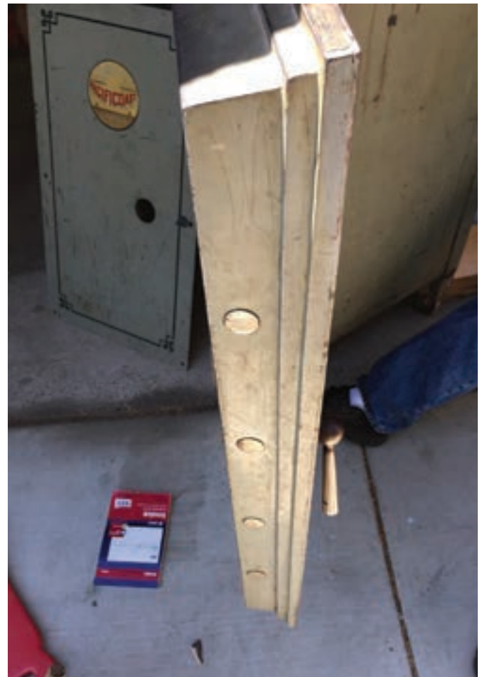
Figure 5. The four bolts are 2\frac{1}{2} " from the face of the door to the centerline of the bolts. They are located at 8", 15\frac{1}{2} ", 23\frac{1}{2} " and 30\frac{1}{2} " down from the top of the door.
