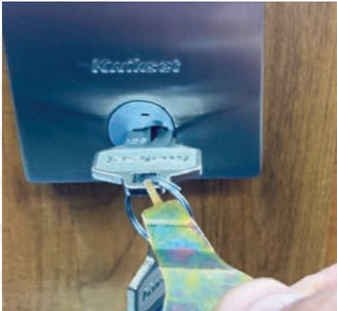
Figure 10. The author is removing the SmartKey learn tool.
