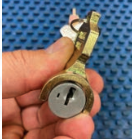
Figure 21. Turn the reset tool and the cylinder clockwise until it stops around the 1 o'clock position.
