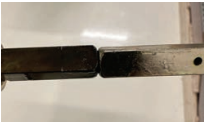
Figure 3. Start by turning the spindles until they touch each other.
