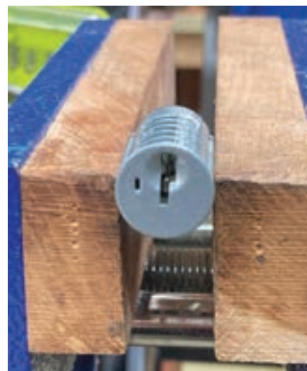
Figure 29. Hold the SC1 SmartKey cylinder upside down with the learn slot on the left side at the 9 o'clock position.
