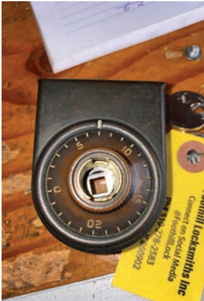
Figure 7. The key cylinder is removed.
