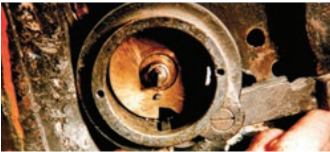
Figure 15. If you look closely, you can see the bottom edge of the hole the author drilled to view the wheel pack. This is a more dangerous location than drilling next to the fence and peeking up with a 70- or 90-degree scope. However, it works great if you only have a straight-view scope or ophthalmology scope for viewing the wheels.
