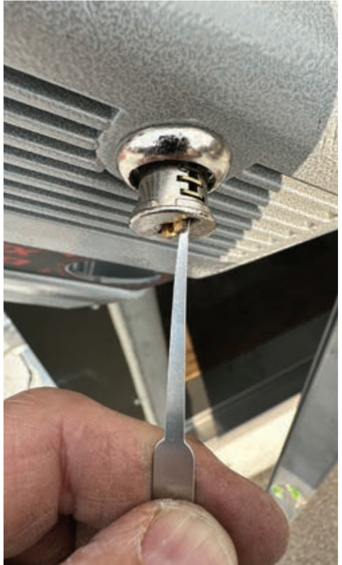
Figure 29. The author put the tip of the feeler pick beside the key and twisted so he could get the key out.
