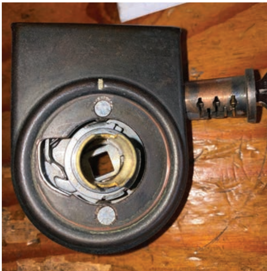
Figure 10. The dial is removed, showing two wheels and a lever.
