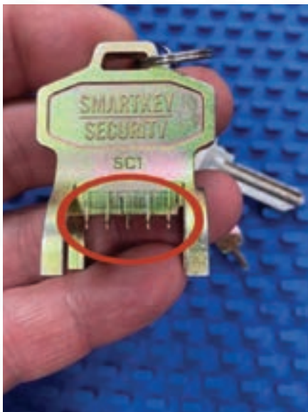
Figure 17. The reset tool has five prongs.
