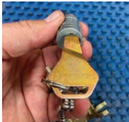
Figure 23. Make sure that the tool is pushed all the way in.
