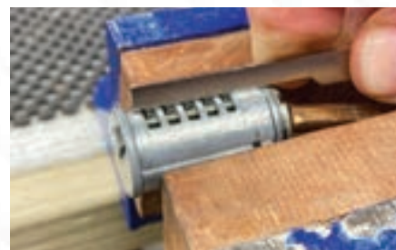
Figure 32. Remove the SC1 key blank while still pressing down with the Better Resetter tool.
