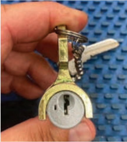
Figure 20. Firmly holding the cylinder and the reset tool in place.
