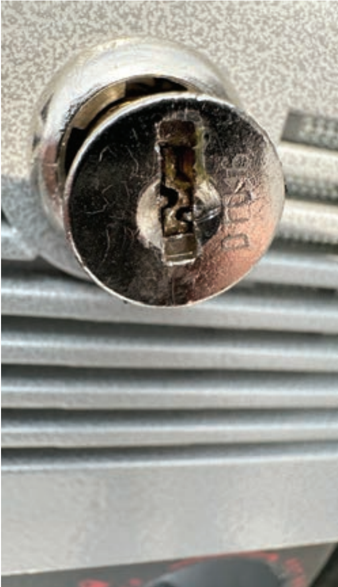
Figure 28. Someone had broken the Detex key off in the lock.
