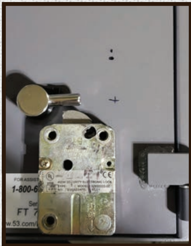
Figure 5. Using a flat wire and my scope, the author placed the wire on the center of the flat edge of the LA GARD lock's swingbolt and marked the depth with a marker on the wire. He then marked this point of reference on the outside of the door.
