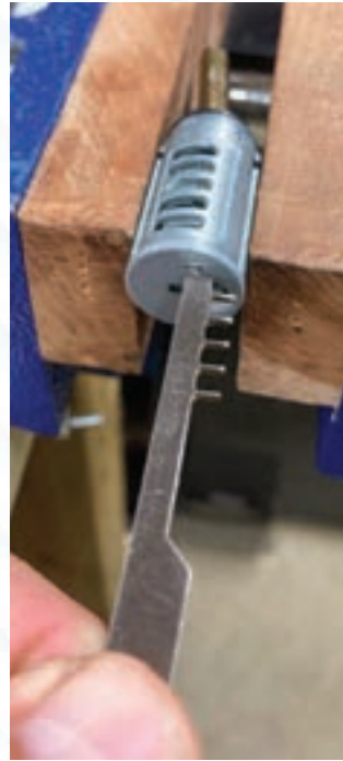
Figure 35. Insert the barb into the learn tool hole.
