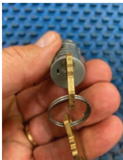
Figure 25. Turn the key to the 6 o'clock position.
