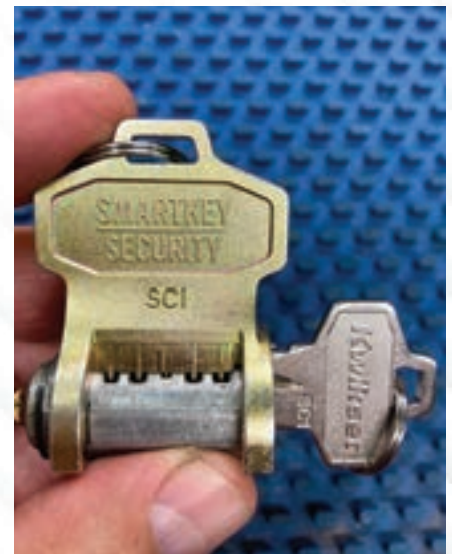
Figure 19. Push the tool down and hold the reset tool in place.
