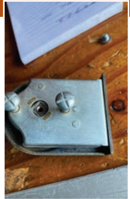
Figure 6. The key cylinder is shown with the dial-retaining screw removed.
