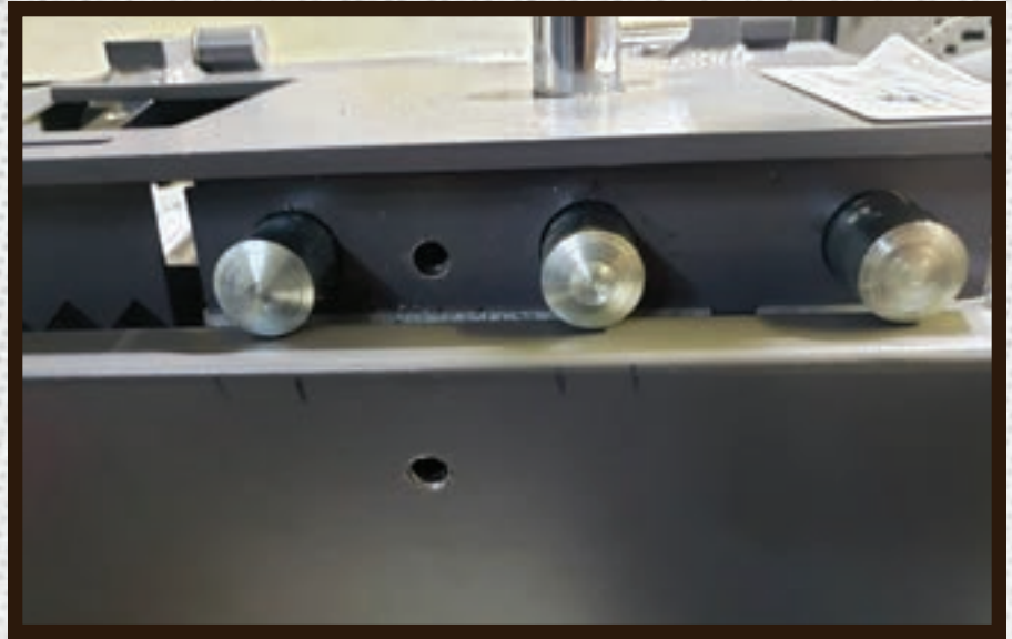
Figure 4. After getting the safe open, the author discovered a third bolt near the bottom that he had missed.
