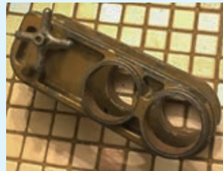
Figure 17. This Kwikset jig has double cross-bore guide holes.
