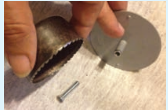
Figures 3 and 4. The author took a slightly worn out 2½" diameter hole saw and partially ground off the teeth.
