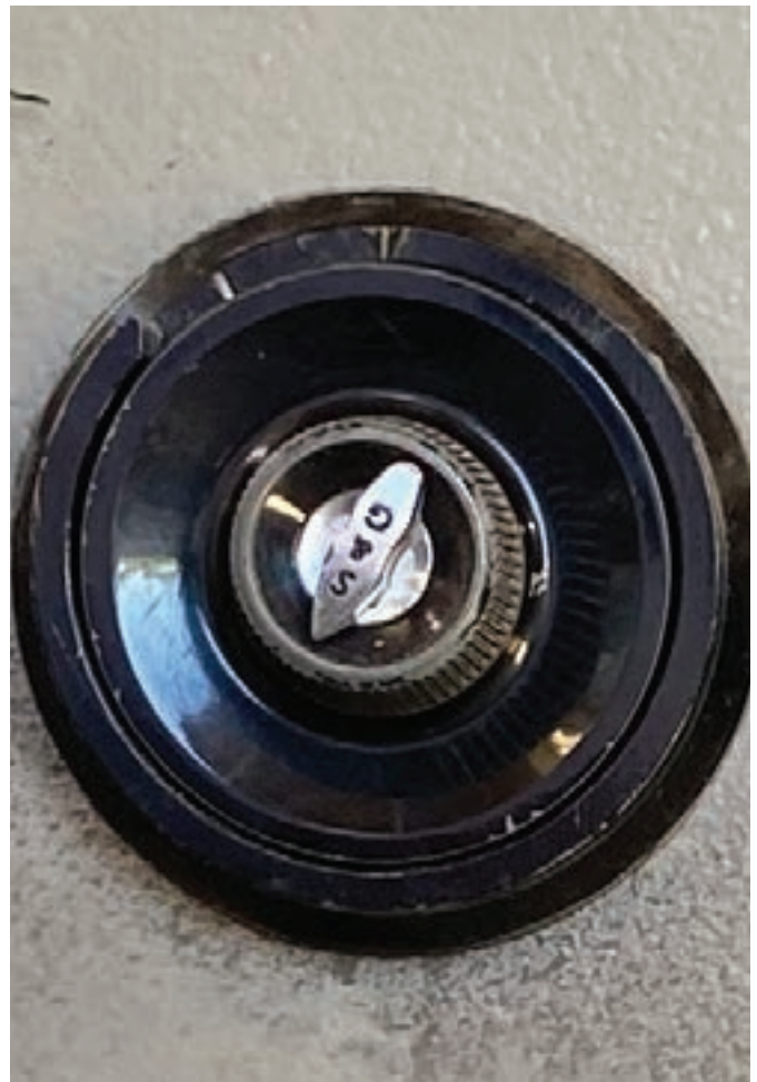
Figure 2. The S&G 8400 lock has a center thumbturn.
