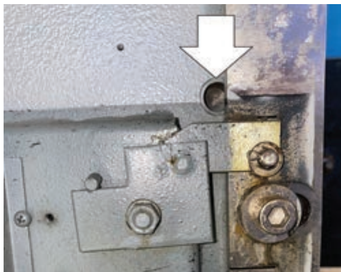
Figure 19. The door pan is removed, showing a location for a relocker used with another type of back cover on another model door with a right hand mounted lock.
