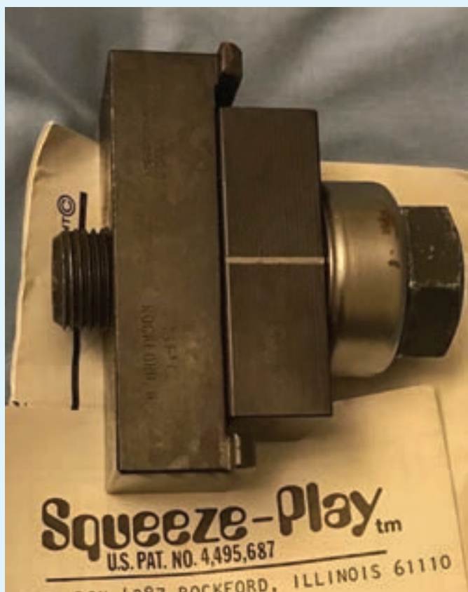
Figure 19. Here is the Squeeze-Play from Sieveking Products Company, which is a latch mortiser for hollow metal doors.
