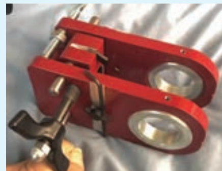
Figure 18. This Bullseye jig has a single cross-bore guide hole on each side.
