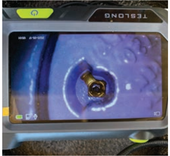
Figure 12. The wheel hubs are aligned, and you can see the change key tip stop.
