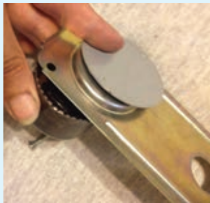
Figure 5. The hole saw is positioned into the side of the mounting plate with the circular indentation.
