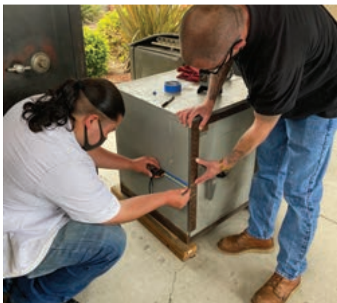
Figure 7. Dustin and Louie guessed the door thickness for scoping, using the measurements of 1.5" door plate, .5" hardplate plus lock body thickness for a first hole guess at 3" from the door face.
