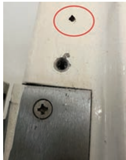
Figure 11. The red circle shows where the weld broke.
