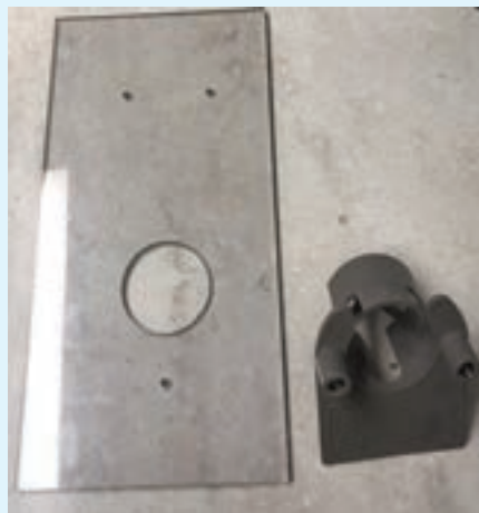
Figure 12. This template has a 2 1/8" diameter hole cut in the position where the cross bore for the previous latch lock was located.
