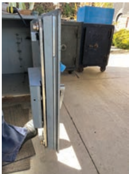
Figure 15. The boltwork is a long locking bar: 23" tall x 2" wide x \frac{3}{8} " thick.
