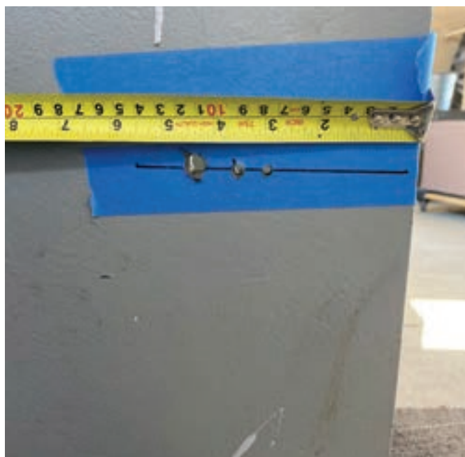
Figure 8. The hole is 4.5" from the body face.
