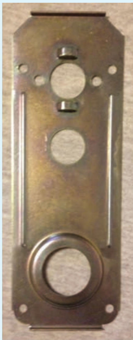
Figure 1. To make a custom installation jig for the KABA Simplex 1000 locks, the author started with one of the mounting plates.
