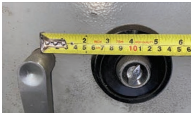
Figure 5. Dial center to handle center was 4".
