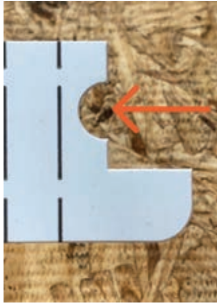
Figure 6. The latch bolt location card has a cutout to fit over the deadlatch of the latch bolt.
