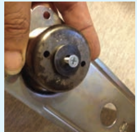
Figure 6. The teeth side of the hole saw is pressed into the circular indentation.
