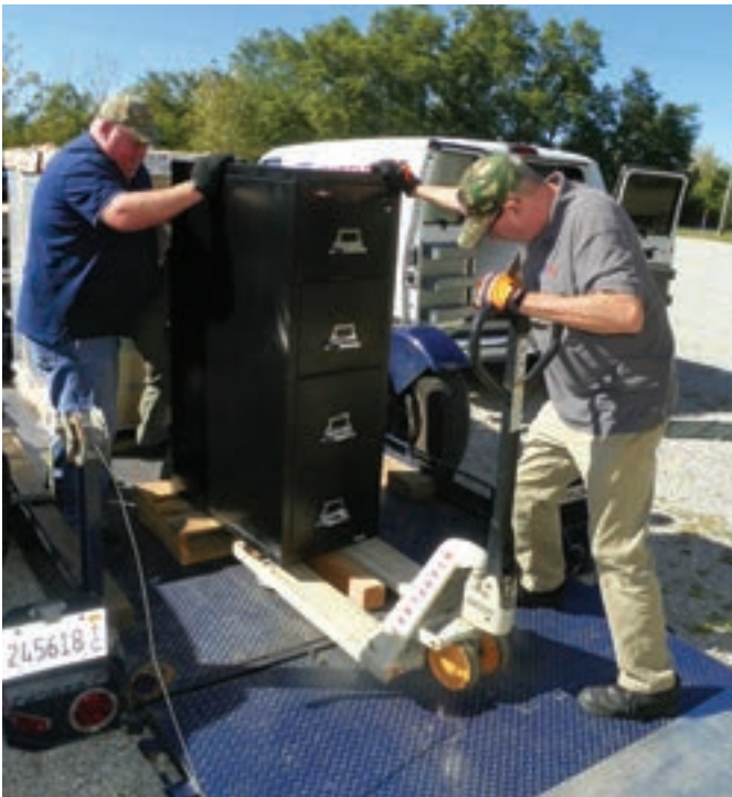
Figure 12. Number One is Ready – File cabinet #1 has been moved from the pallet to the pallet jack. A long 4x4 block was used to increase stability. Notice that more aluminum sheeting was used to bridge the height difference from the tailgate to the sidewalk.
