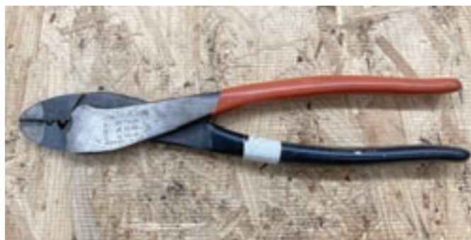
Figure 26. The author likes using these Sta-Kon (Thomas & Betts) crimping pliers.
