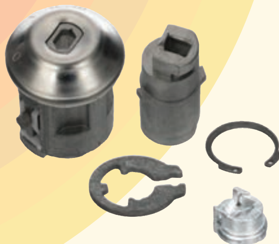
Figure 17. Shown here are the housing, plug, C-clip and retainer of a Ford Tibbe ignition lock.
