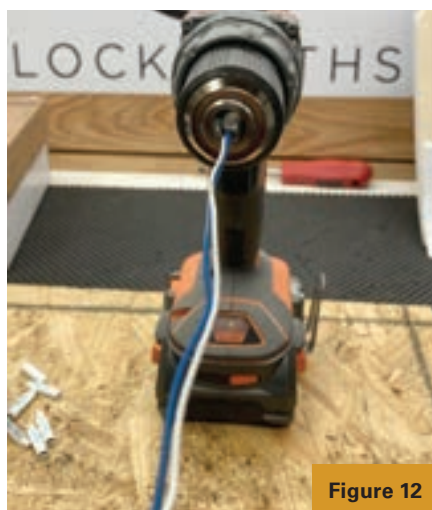
Figures 12 and 13. The author uses a drill to wind the wires together.
