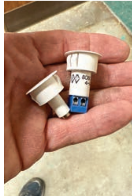
Figure 17. Here are the contact and magnet that come with each lock.
