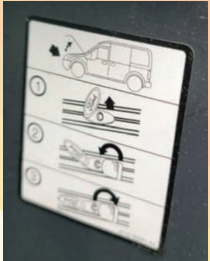
Figure 25. This image shows the procedure for a hood release.
