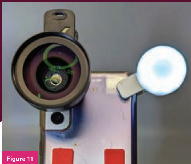
Figures 11 and 12. The Glow Clip LED light is rechargeable and has three levels of brightness.
