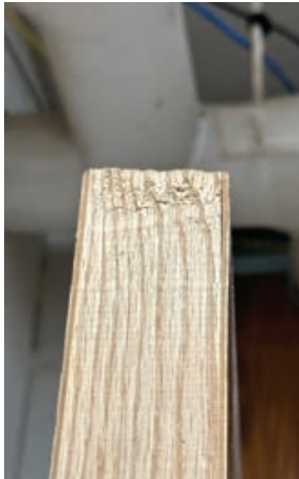
Figure 3. It's visible how the plane sniped the top of the door.
