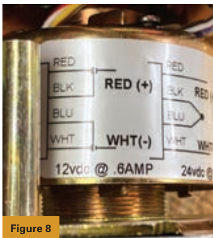
Figures 8 and 9. Here's the wiring diagram that can be found on the body of the lock for both 12 VDC and 24 VDC.
