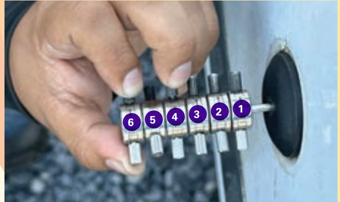
Figure 18. Here's a visual aid for spacing for the Lishi Ford Tibbe pick.
