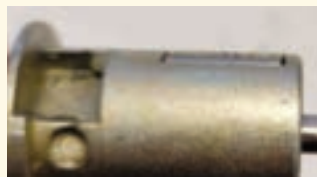
Figure 7. This image shows the side bar of a door lock dropped into the plug after a properly cut key has been turned.
