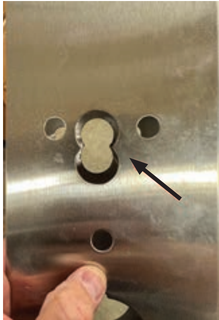
Figure 15. Here's a modification to the plate to make room for stashing the excess wire.
