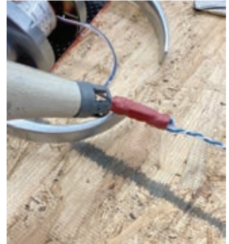
Figure 18. The author applied heat to the heat shrink tubing.
