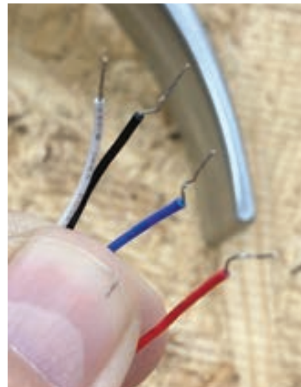
Figure 7. There are four wires (white, black, blue and red) that will connect to the incoming power.
