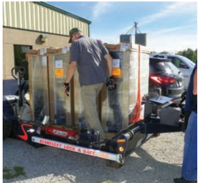
Figure 8. On The Ground – With the trailer lowered and all of the straps loose and mostly out of the way, Gene headed for the aluminum sheets to smooth out the transition points of the path of travel. Any large, heavy load will handle better if you use every opportunity to eliminate or overcome any steps, ridges, bumps or gradient differences before you start moving the load.
