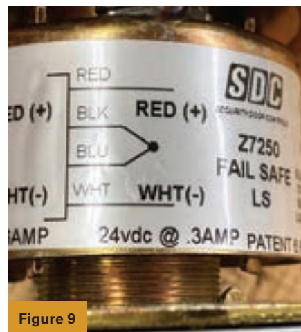
Figures 8 and 9. Here's the wiring diagram that can be found on the body of the lock for both 12 VDC and 24 VDC.
