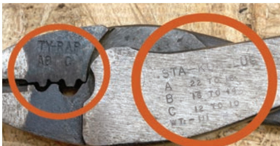
Figure 27. The author's crimping pliers have the terminal and wire gauge sizes stamped on the side of the tool.
