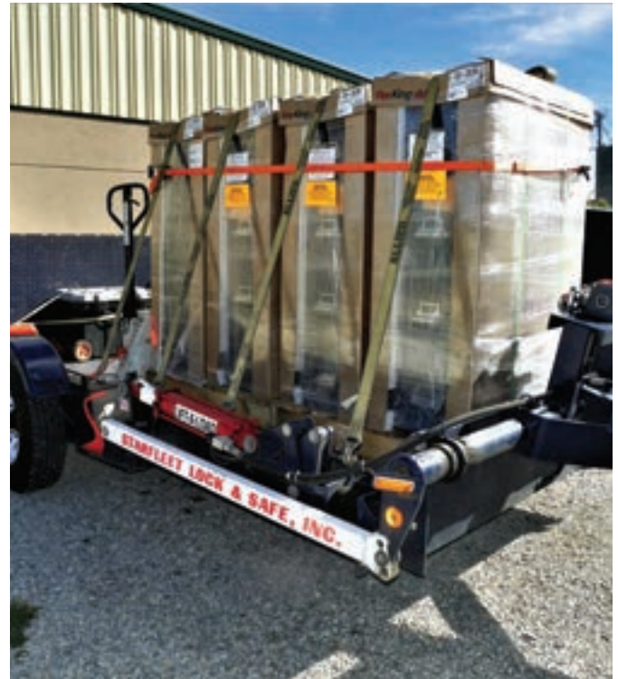
Figure 2. Loaded for Fire – With the Lift-A-Load trailer packed with the four FireKing #1831-C-BL files; standard and narrow pallet jacks; various thicknesses of aluminum sheets; and plenty of wood blocks of various sizes, we arrived at the job location.
