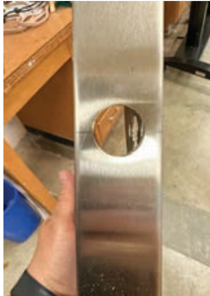
Figure 16. This is a 1" hole drilled on the lock edge of the plate and on the same centerline as the top hole of the figure eight shown in Figure 15.
