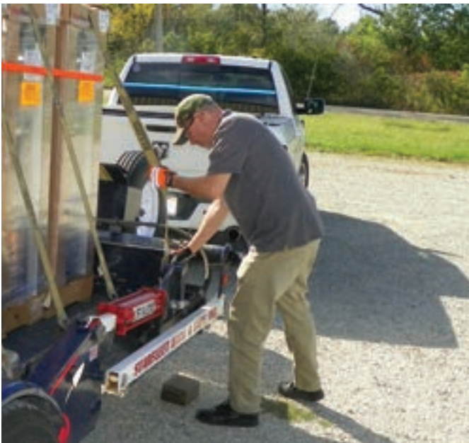
Figure 7. Blocks In Place – As Gene released the large straps on the other side, you could spot the 4x6 wood block placed under both front corners of the trailer bed. This gravel parking lot was sloped enough that we needed to add support to ensure that when we lowered trailer bed, it would be level with the sidewalk area for smooth unloading.
