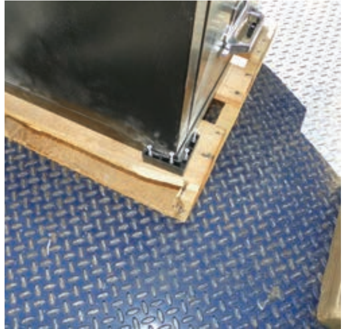
Figure 11. Remove the Brackets – Small nylon brackets with four screws each are used to prevent movement of the file on the pallet during shipping. We usually save a few such little items for use on future projects. Sometimes you simply need a black 90-degree plastic widget.
