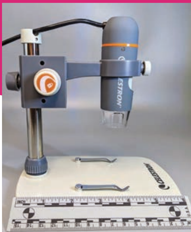
Figure 8. The Celestron 44308 “pro” version has a weighted base and an adjustable rail, so it stays steady.
