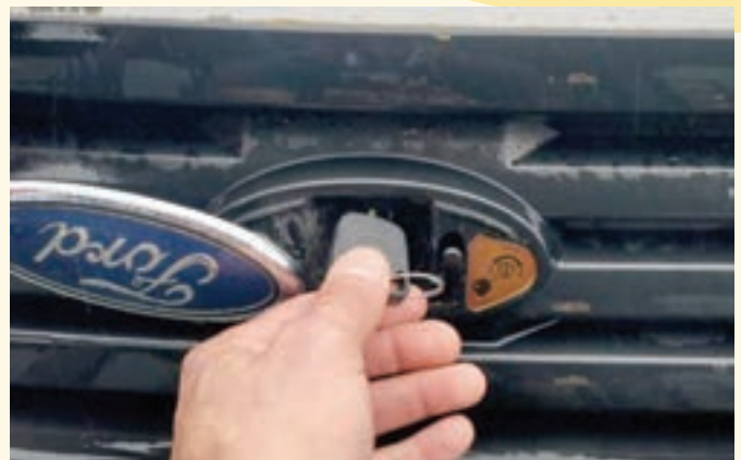
Figure 26. The key is disengaging the hood release.
