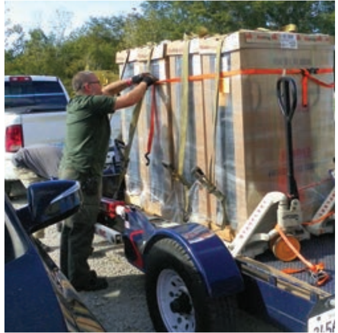
Figure 6. Release the Other Straps – The smaller orange strap was wrapped around the cabinets and intersected with the large straps to make one cohesive block of weight secured to the trailer. The liability of a loosely strapped load includes more than the potential damage or destruction of the load itself. Other motorists and pedestrians can be injured or killed by an improperly secured load.
