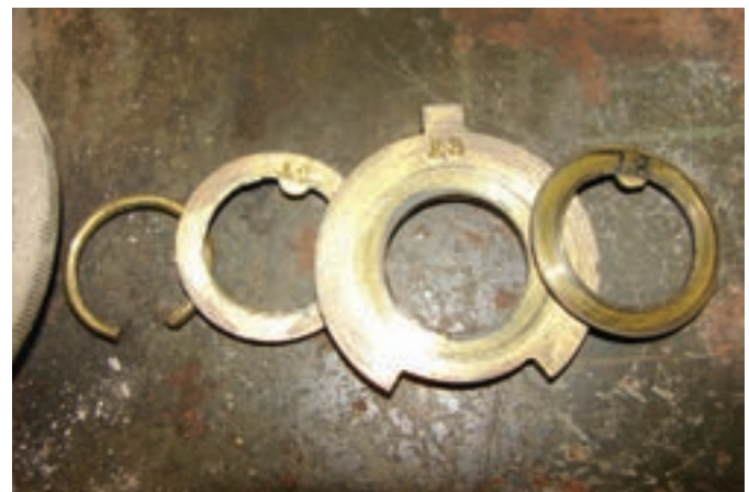
Figure 18. There is another spacer washer with tab below the "fly" washer.
