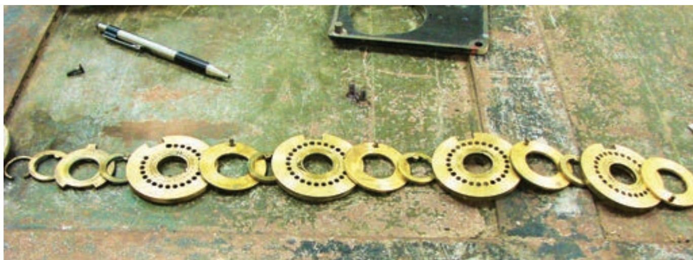
Figure 21. Here are all 15 parts that make up the wheelpack.
