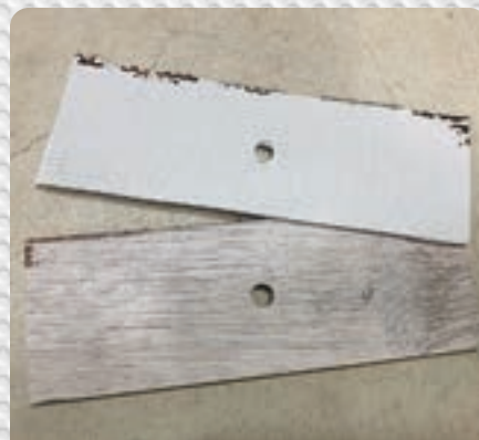
Figure 14. There were homemade spacers made from questionable material.
