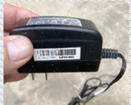
Figure 3. The 12 VDC transformer was plugged into an outlet under the receptionist's desk.
