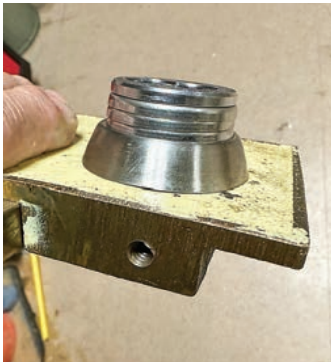
Figure 9. The BEST cylinder was a lot longer, so the author used three No. 1 cylinder rings on top of a No. 3 ring.
