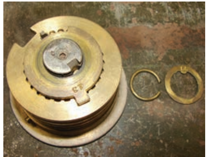
Figure 17. You can see the snap ring that holds everything below it in place plus the spacer washer with its tab.
