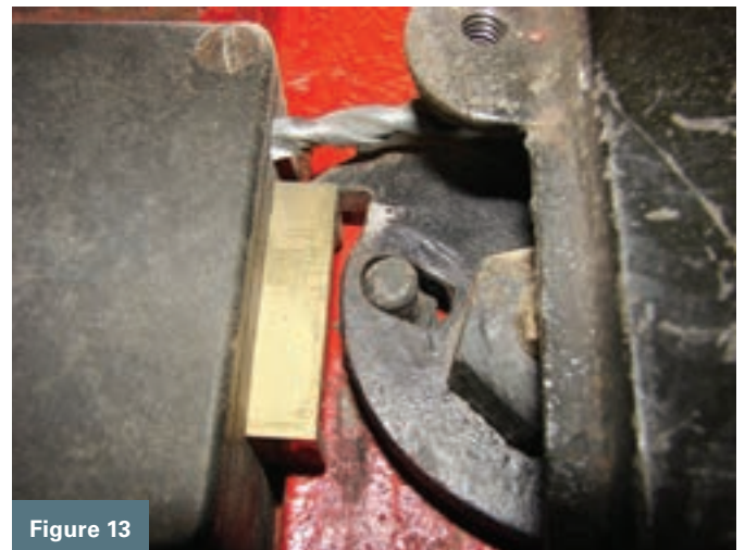
Figure 11. Here, you can see where the cam from the boltwork has entered the lock body.
