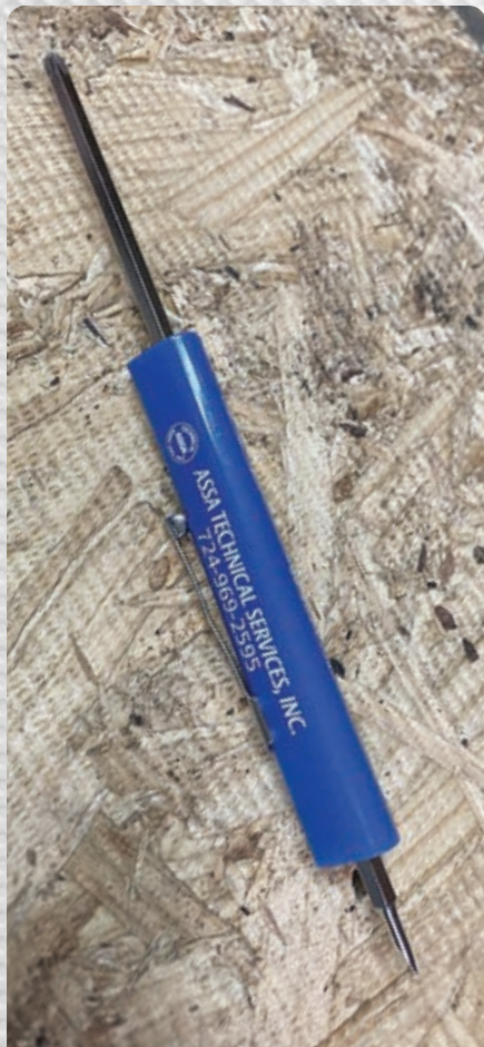
Figure 17. When working alone, the author places a small tweaker screwdriver on the door's magnet to find out if it is powered and working.
