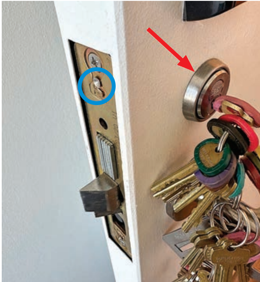
Figure 2. What was left of the screw head looked like what's in the blue circle.
