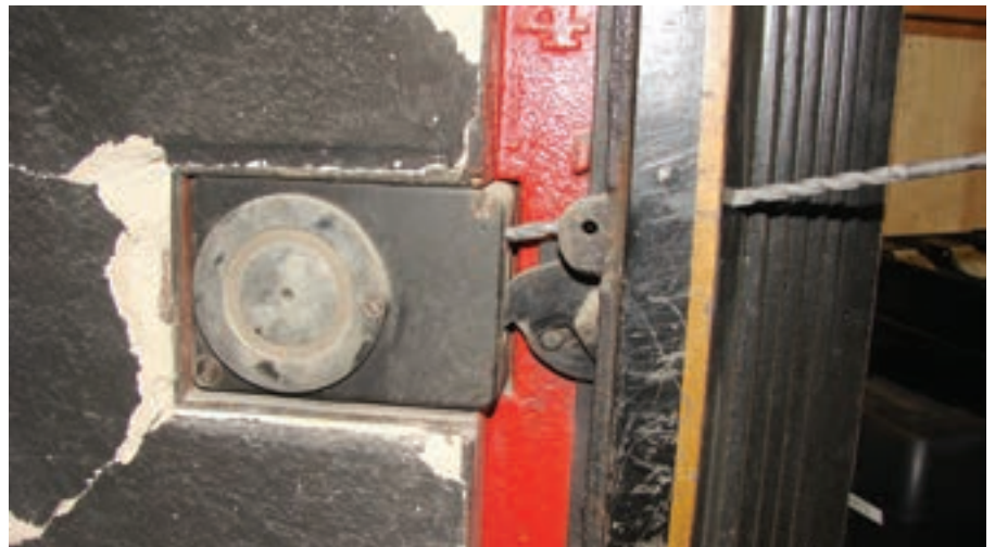
Figure 11. Here, you can see where the cam from the boltwork has entered the lock body.
