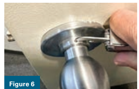
Figures 5 and 6. You can use the can/bottle opener you'll find on most multi-tools to tighten a loose rose ring that you'd ordinarily use a spanner wrench for.
