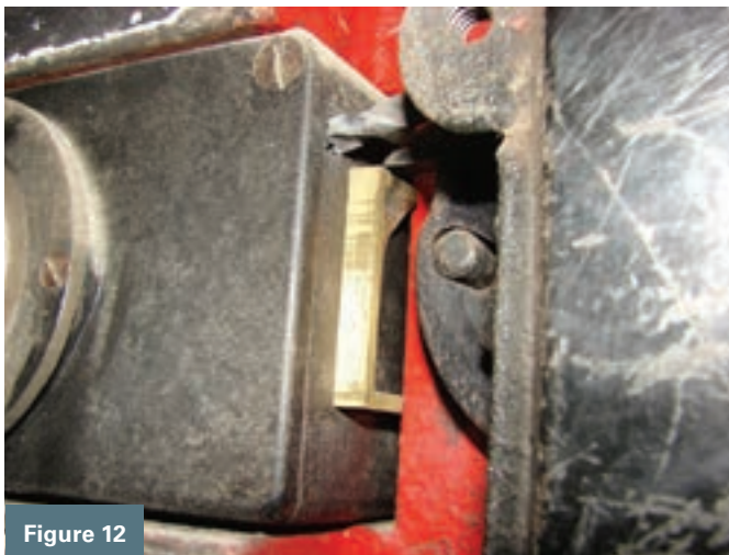
Figure 10. You can see the curb-style lock and where the drill penetrated the lock.
