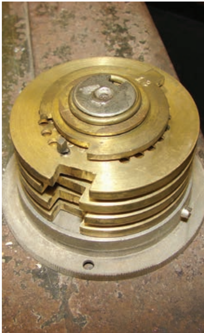
Figure 16. The wheelpack is a four-wheel lock.
