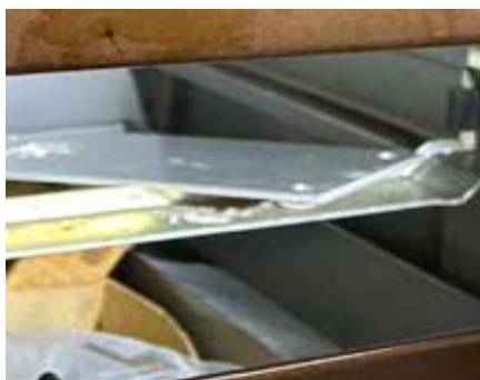
Figure 23. A pair of push plates had slid off the top drawer and were in the way.
