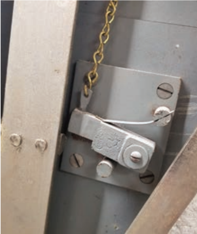
Figure 7. Disassembly. With the inner cover removed, the entire mechanism could be observed. This lower relocker used a strong spring to actively block the bolt mechanism if it were activated. The attached chain leads up to the lock case.
