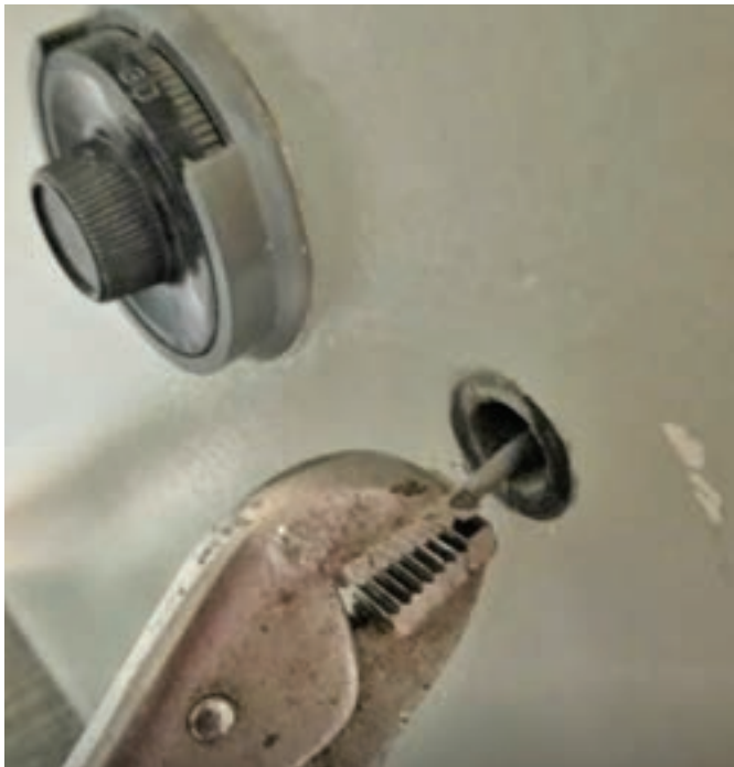
Figure 3. The Tap. Being fresh out of left-handed taps and bolts, I crossed my fingers and decided to go once again with my old pal “hope.” I drilled slowly and soon was able to put an easy-out extractor in the hole. The drilling went fine, as did the insertion of the screw extractor. I was praying it would give me enough torque to move the bolts without them breaking off. Using my trusty Vise-Grips, I began applying torque to the left as I vibrated around the makeshift handle with a small rubber hammer. Not even one small bit of movement.
