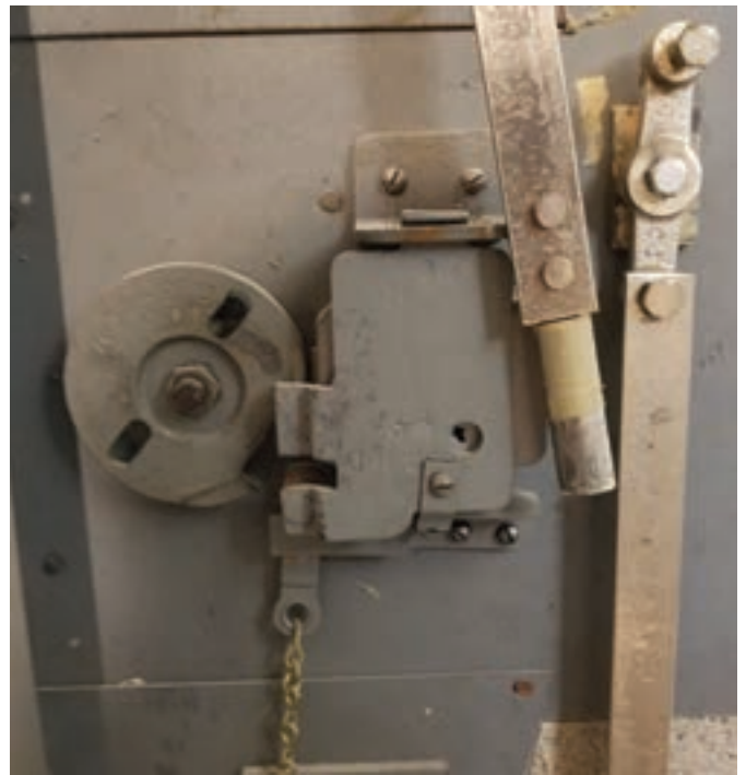
Figure 8. Dual Coverage. The relock plate attached to the back of the lock also employed a fusible link. If the lock is punched, the cover movement engages the relocker. If a torch is used, the fusible link would melt, again causing the bolt assembly to be in a bind. The upper bolt is visible here because I cleaned and properly lubed all pivot points and locking bolts and made a slight adjustment to the upper bolt guide in the process.
