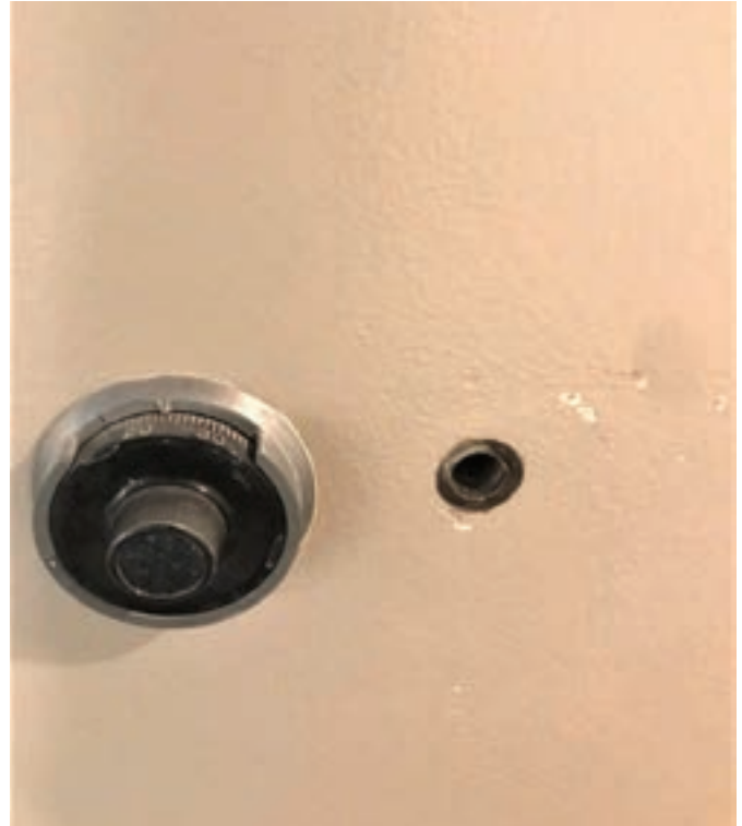
Figure 2. The Handle. Confused, I walked over to the door, and as I touched the handle, it fell to the floor. Looking down at the handle and then to the gaping hole in the door, I saw the jagged end of the arbor that had broken off exactly where it was supposed to: at the stress point engineered into it. Trying the dial, I noticed the reason it wasn't turning was because the bolt wouldn't throw, as it was hitting the bolt cam. Hmm... it appeared that this thing was already at least partly unlocked. Hoping for the correct answer, I asked which way the handle turned to open the door. My thoughts of drilling and tapping to put a Grade 8 bolt into the broken shaft to turn it were dashed when the answer was "to the left."
