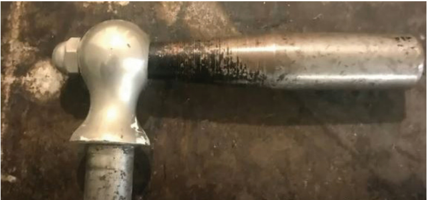
Figure 9. The Fix. I disassembled and removed the drive cam and arbor, then beveled the edges. I clamped the handle and remainder together into the "V" of a piece of angle iron to ensure a straight alignment during the repair. I welded the arbor together, ensuring that I got good penetration and a solid weld. After applying a wee bit of dressing with a flap disc to make a nice smooth surface, the handle assembly was ready to go.
