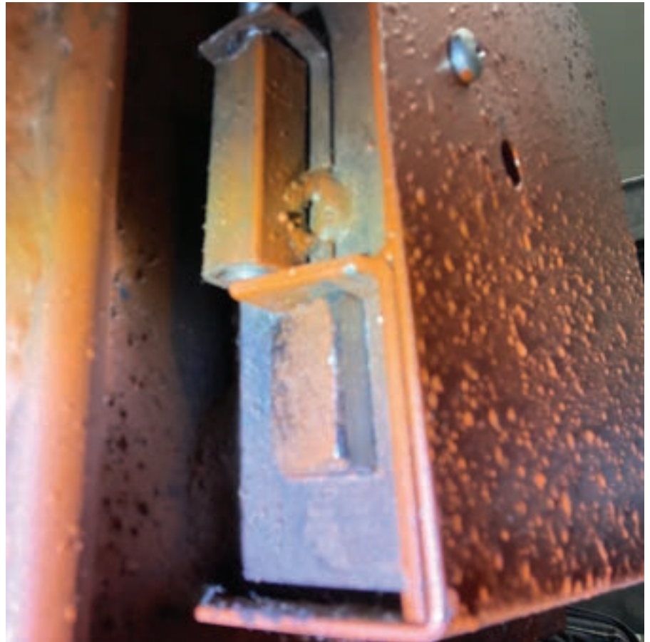
FIGURE 17. The door pan is reattached and holding the relocker.
