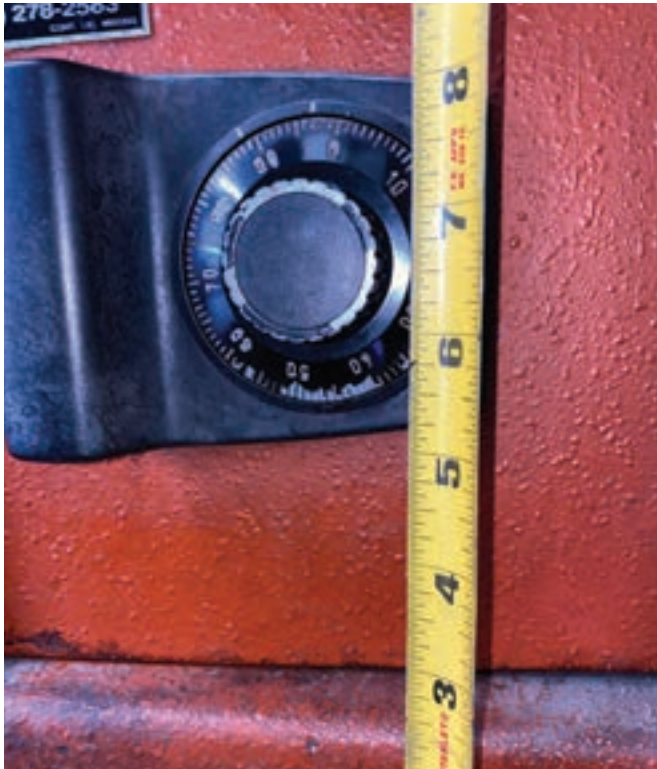
FIGURE 2. The author is measuring from the bottom of the safe to dial center.
