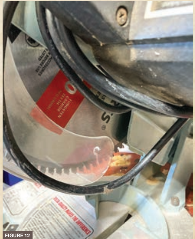
FIGURES 11 AND 12. The author installed a new 10" 80-tooth tungsten carbide blade specifically for cutting aluminum and plastic.
