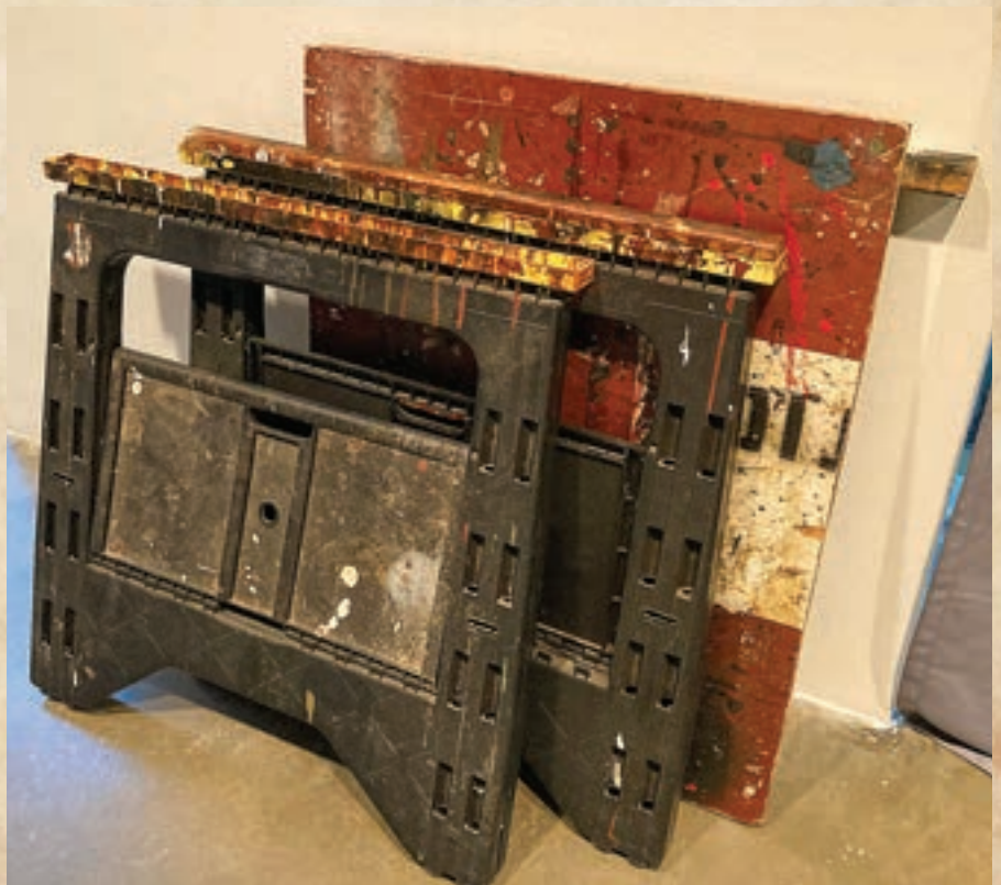
FIGURE 8. The author's portable workbench consists of just two foldable sawhorses and a sheet of ½" thick pine plywood.
