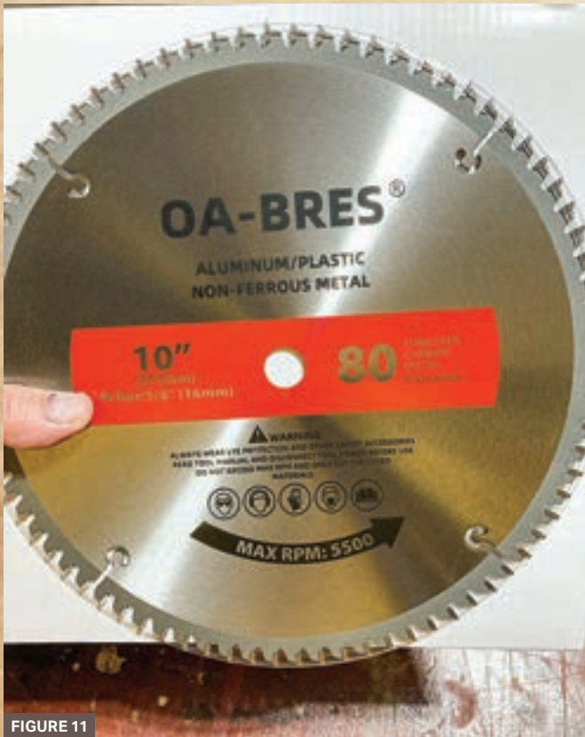
FIGURES 11 AND 12. The author installed a new 10" 80-tooth tungsten carbide blade specifically for cutting aluminum and plastic.
