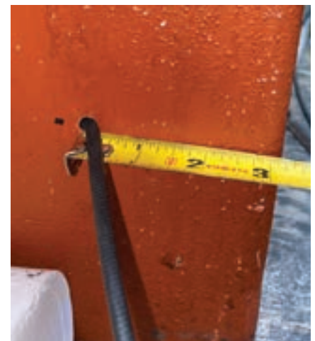
FIGURE 4. The depth estimate is 3" from the face of the body.
