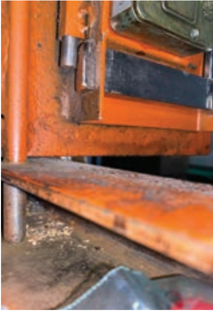
FIGURE 9. The external relocker has fired.
