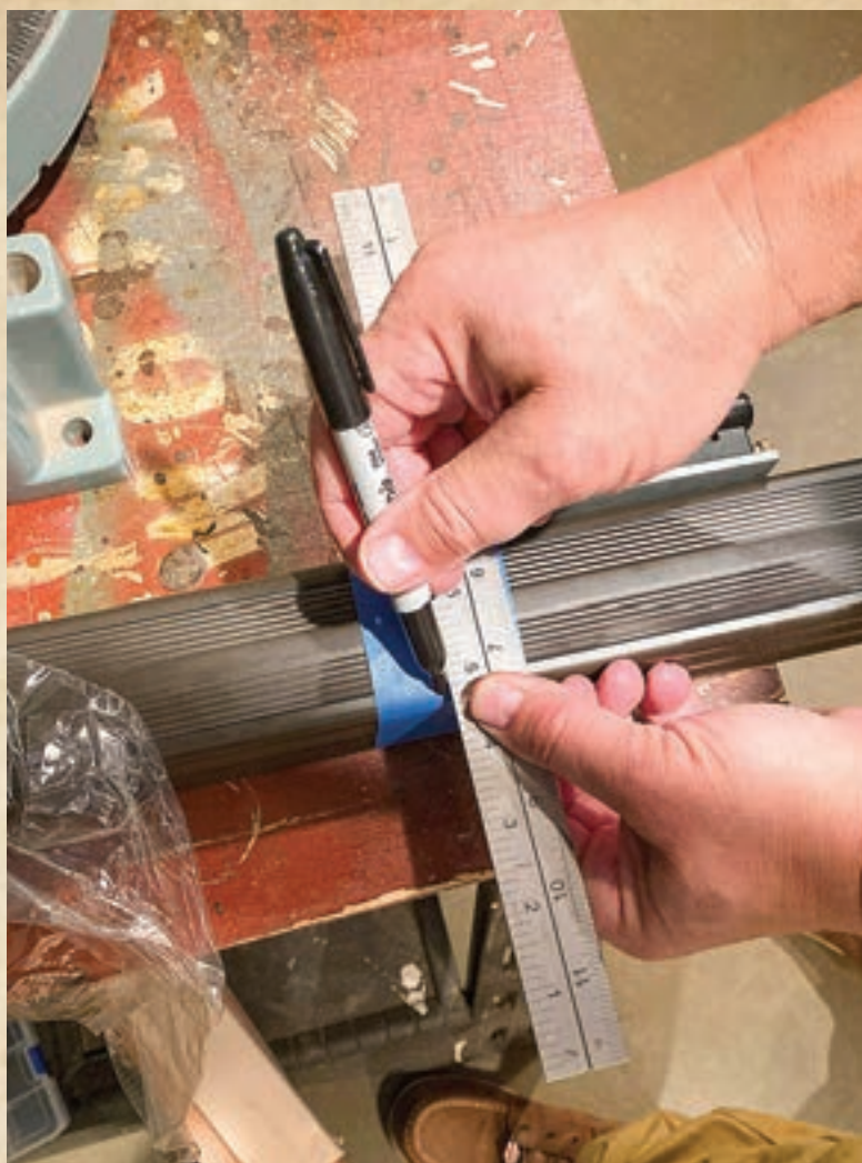
FIGURE 14. The author used a tape measure to measure where he was going to cut the bar and then used a combination square and pen to make a cut mark.
