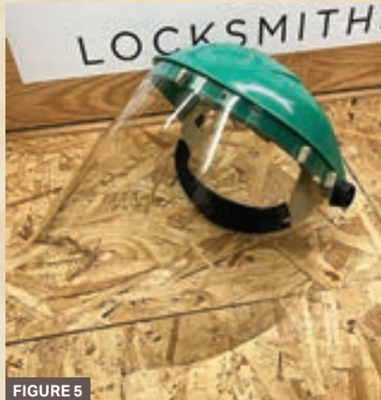
FIGURES 4 AND 5. Safety goggles and a face shield are a must to protect your eyes.
