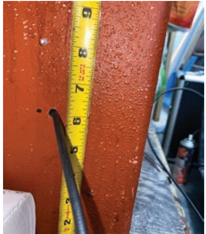
FIGURE 3. For an RH lock, deduct \frac{1}{2} " from dial center for the change keyhole.
