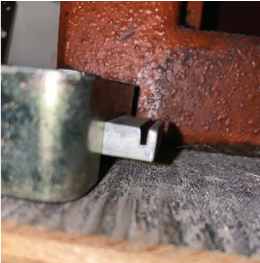
FIGURE 14. You can see the cutout in the lock bolt.
