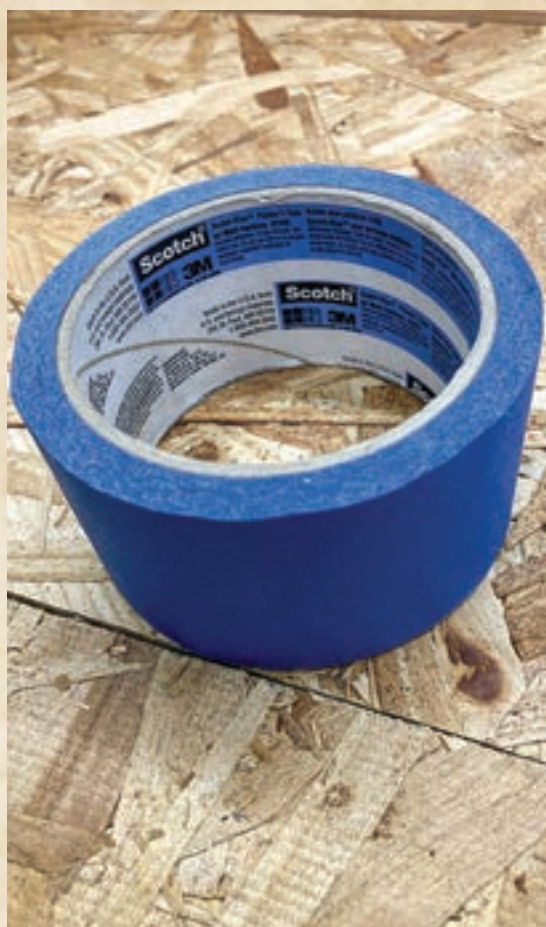
FIGURE 13. By using painter's tape, the author could clearly see his cut lines, and the bar was protected from debris and scratches.
