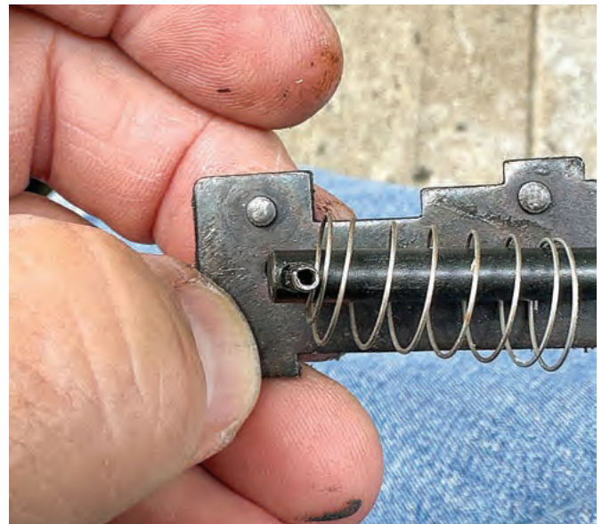
FIGURE 22. The author is holding the slide in the position it will be in to make the chassis fail-secure.
