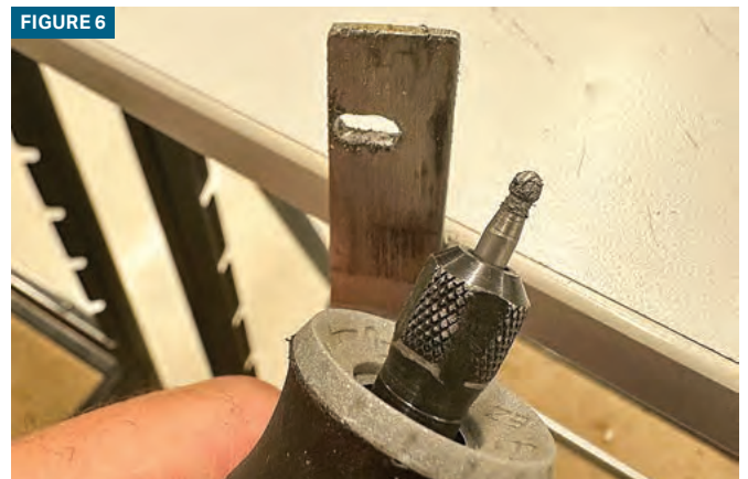
FIGURE 4. The author used a carbide Dremel tool to grind down two of the rivets on the back of the locks.
