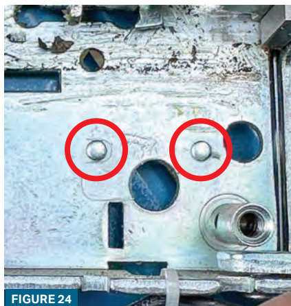
FIGURES 23 AND 24. In Figure 23, you can see the bottom of the bracket that holds the solenoid. The arrows point to a hole and a slot that will fit over the two circled projections in Figure 24.
