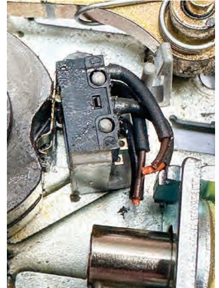
FIGURE 14. The two RQE switches are shown after the wires were cut and removed.
