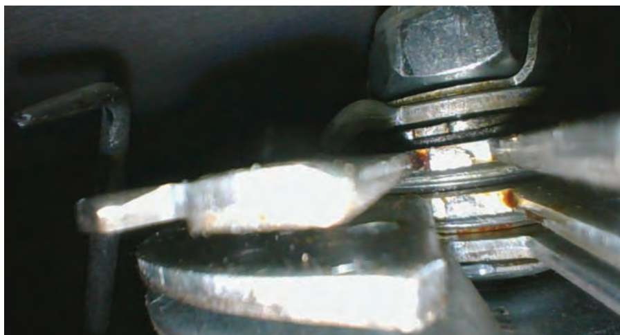
FIGURE 6. All the wheels are almost lined up. You can see the shrum tool in the background used to move the wheels.
