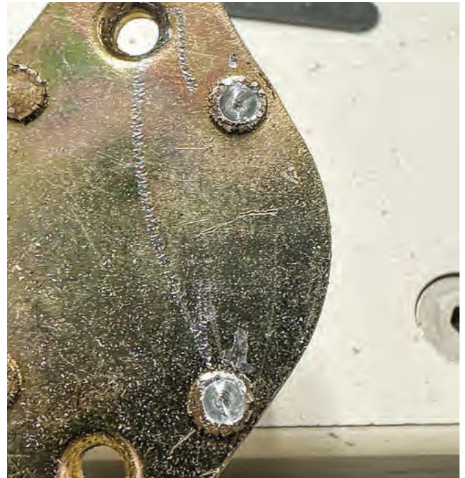
FIGURE 4. The author used a carbide Dremel tool to grind down two of the rivets on the back of the locks.
