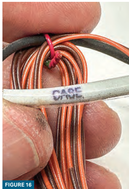
FIGURES 15 AND 16. Here are close-up views of the RQE wire labels.
