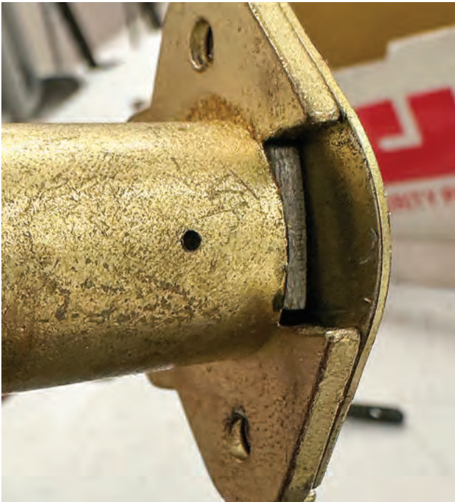
FIGURE 3. Here is the access hole to push in the plug retainer.
