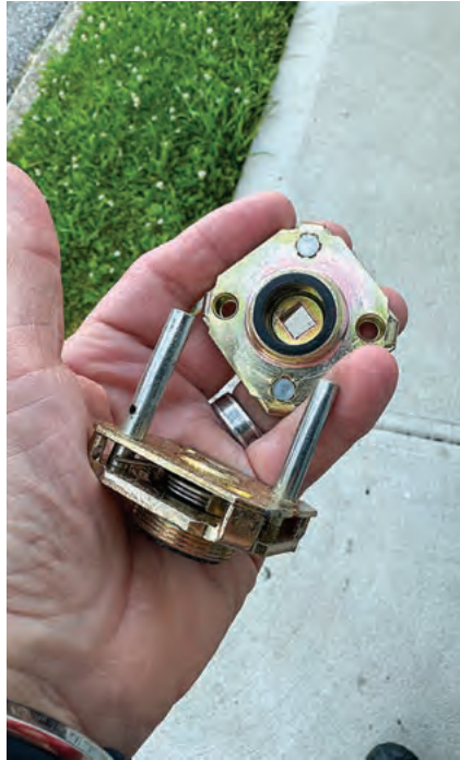
FIGURE 8. The author suspected the spring cassettes needed replacing.
