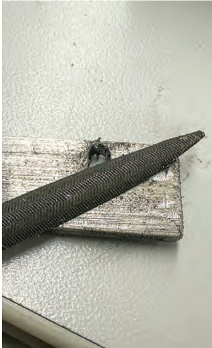
FIGURE 7. A file was used to remove any burrs from the bolt.
