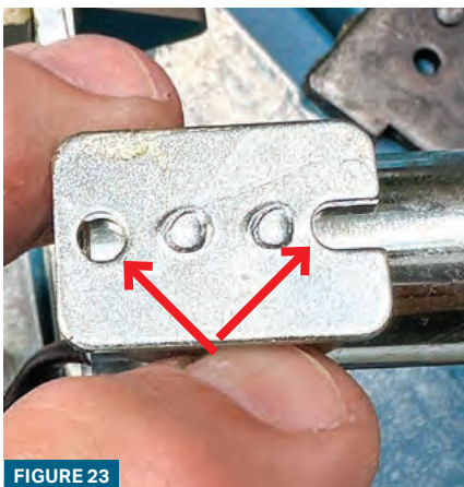
FIGURES 23 AND 24. In Figure 23, you can see the bottom of the bracket that holds the solenoid. The arrows point to a hole and a slot that will fit over the two circled projections in Figure 24.
