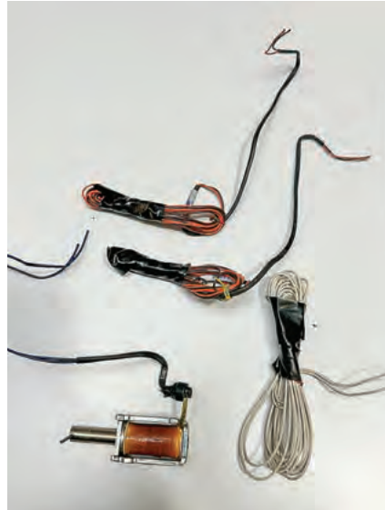
FIGURE 13. From the top down are two request to exit (RQE) wires, a door position switch wire and the burnt-out solenoid.
