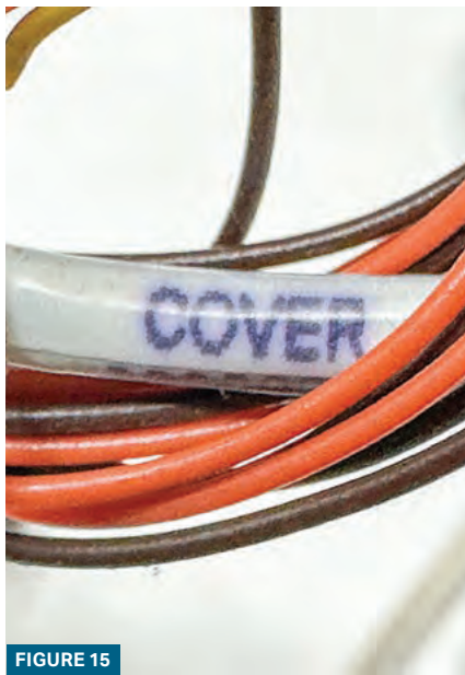
FIGURES 15 AND 16. Here are close-up views of the RQE wire labels.
