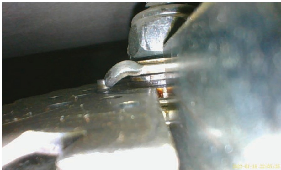
FIGURE 8. The fence is entering the wheel pack.
