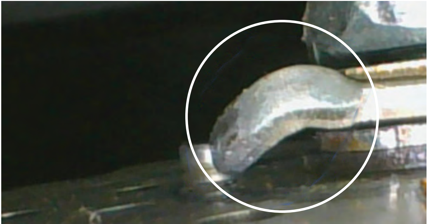
FIGURE 5. Circled is one of the bent drive cam pins. It is supposed to be seated in a hole in the wheel directly below.
