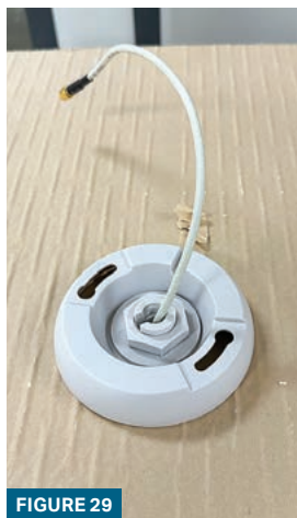
FIGURES 27-29. You can see the sequence of securing the antenna with the plastic washer and nut.
