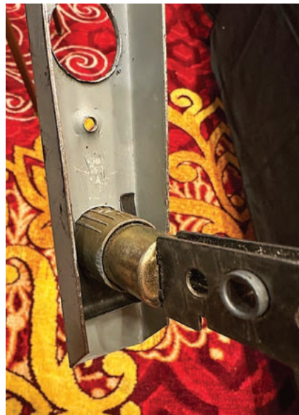
FIGURE 8. The locksmith had cut slots on the drive bolt and used a metal clip.
