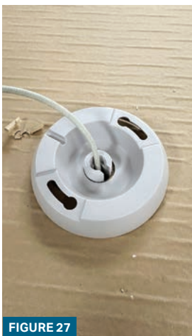
FIGURES 27-29. You can see the sequence of securing the antenna with the plastic washer and nut.
