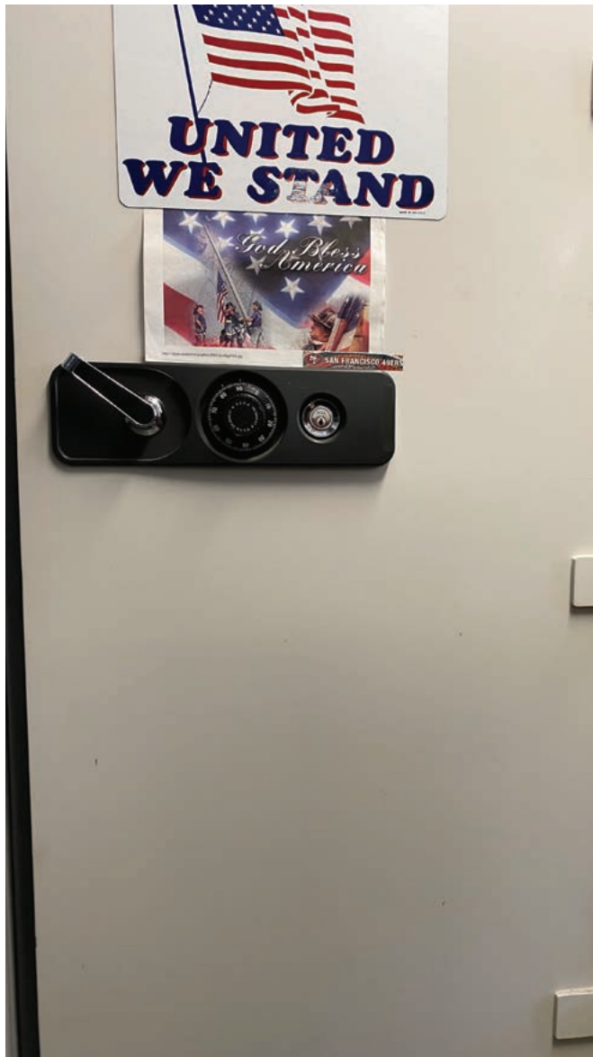
FIGURE 1. When I arrived at the job site, I was taken to the safe in the garage. The question then was: Is this a direct drive lock or a standard magic module lock? To tell for sure, let's take the door pan off.
