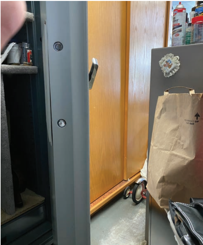
FIGURE 3. There are two door bolts on the opening side at 18¼" and 25¼" from the top of the door.
