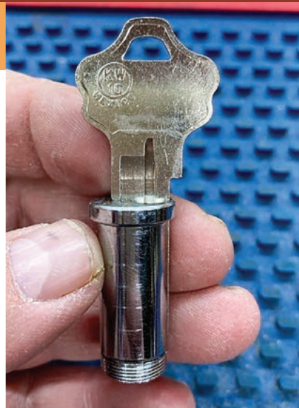
FIGURE 23. A KW10 key blank may also be used.
