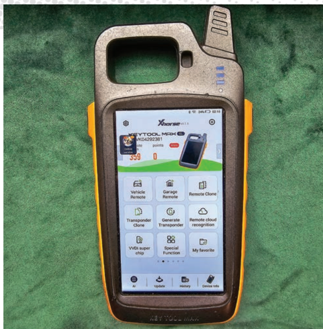
FIGURE 2. VVDI Key Tool Max by Xhorse is one option for writing chips.
