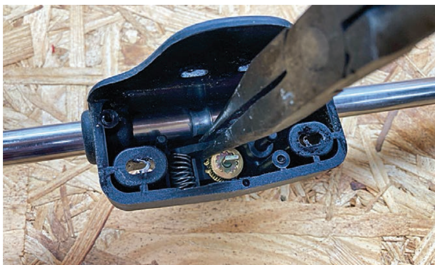
FIGURE 13. The author is removing the Lokk Bolt lock collar and collar lock spring.
