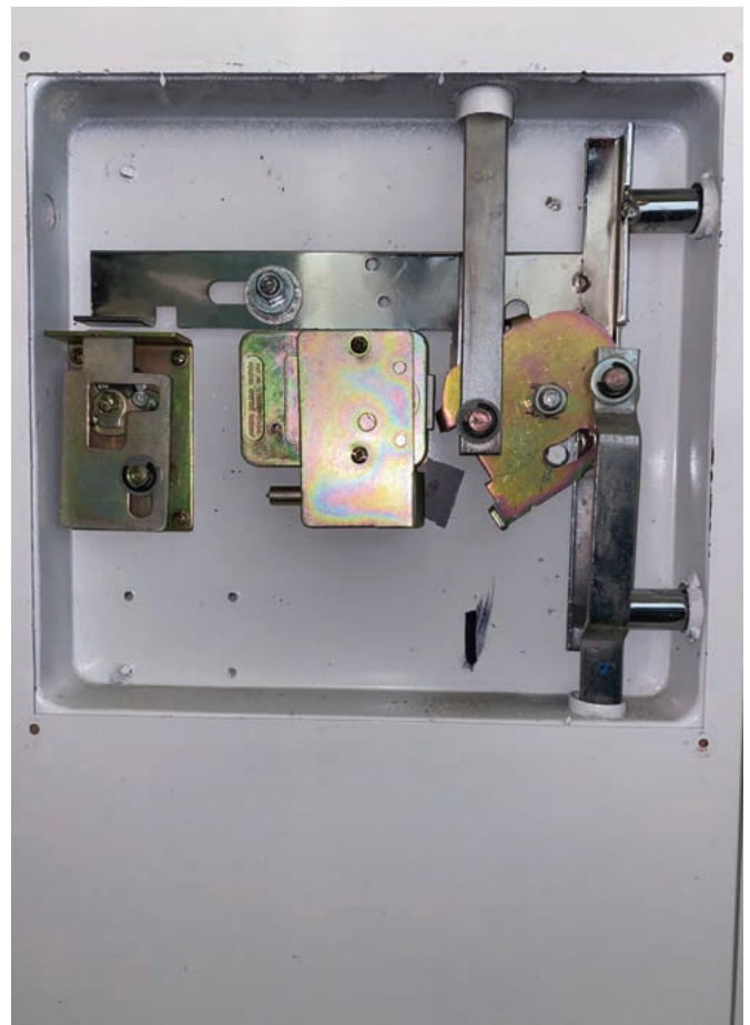
FIGURE 2. You can see the door pan here. It had a standard LA GARD combination lock. I told the customer no problem — I can upgrade it to an electronic lock.
