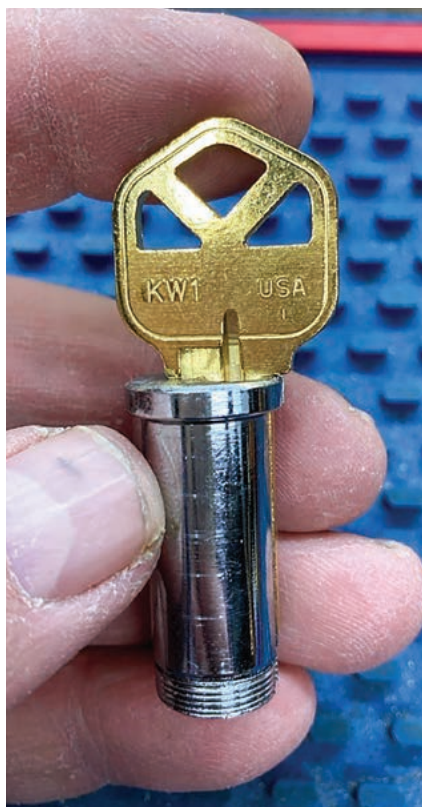
FIGURE 21. A KW1 key blank can be used if you don't have a KW5.
