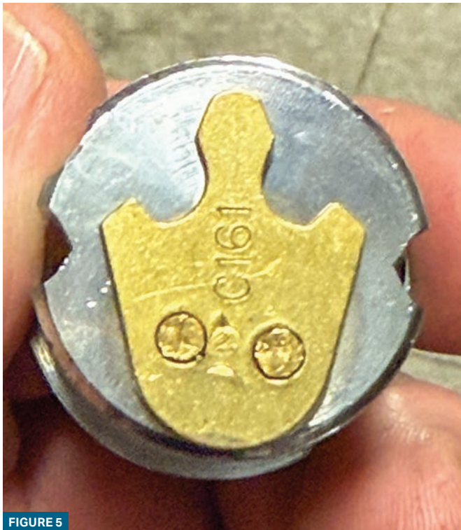
FIGURES 5 AND 6. These photos show a mortise cylinder correctly timed versus incorrectly.
