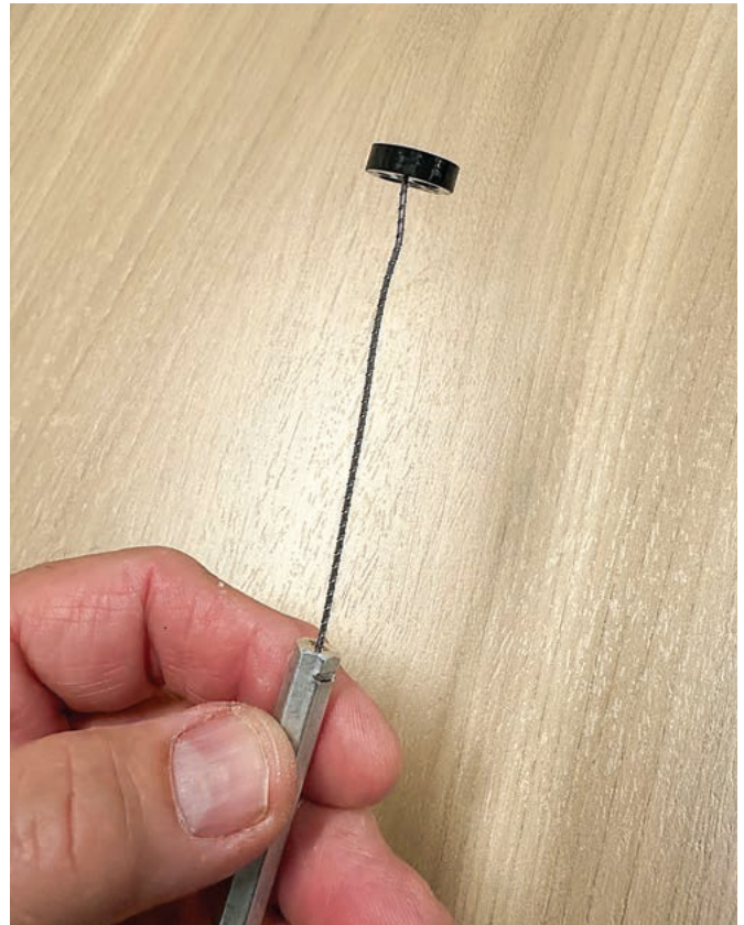
FIGURE 2. The author used a fairly stiff spiral key extractor that wouldn't bend and screwed it into the spacer to pull it out.
