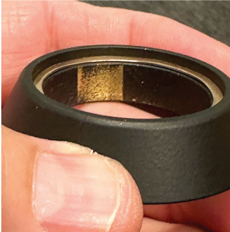
FIGURE 7. The author is holding the cylinder ring with the wave washer inside of it.
