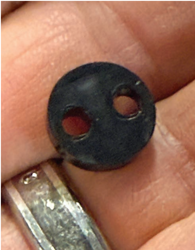
FIGURE 1. A contractor used a black plastic spacer in a six-pin BEST core that was installed in a seven-pin lock.
